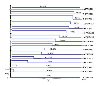
Figure 8. The different signals generated by the ARDUINO Board
