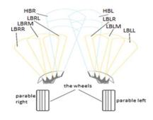
Figure 4. lighting trajectories for different lamps
