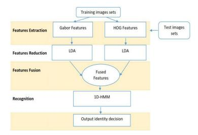
Figure 1. The overall of the proposed face recognition system.
