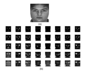
Figure 2. An example of the Gabor magnitude output: (a) the initial image (b) the magnitude output of the filtering operation with a bank of 40 Gabor filters.
