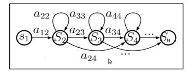
Figure 4. An example of a Left-Right 1D-HMM with N states.
