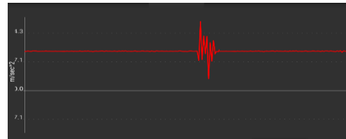
Figure 7. Accelerometer graph on speed breaker
