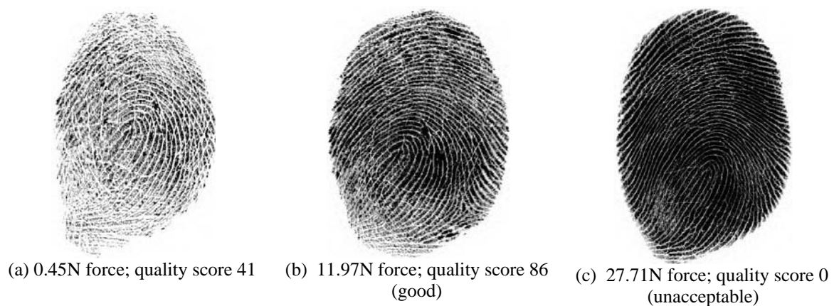
Figure 2. The flat fingerprint images and quality scores of the left thumb at three force levels
