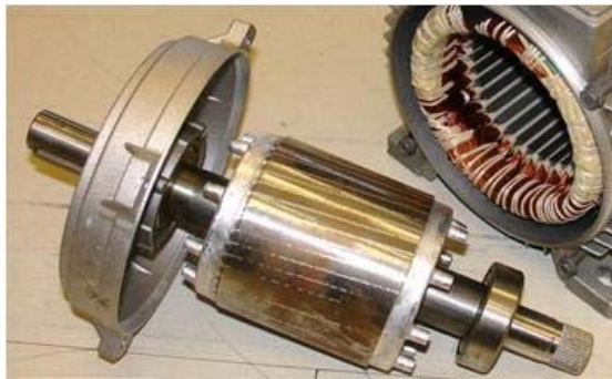
Figure 1. Squirrel cage rotor
