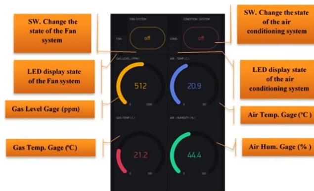
Figure 9. The developed smartphone application based Blynk platform
