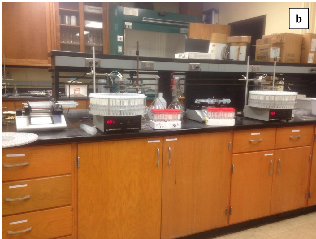
Figure F6. a) and b) lab settings with auto samplers collecting the leachate samples
