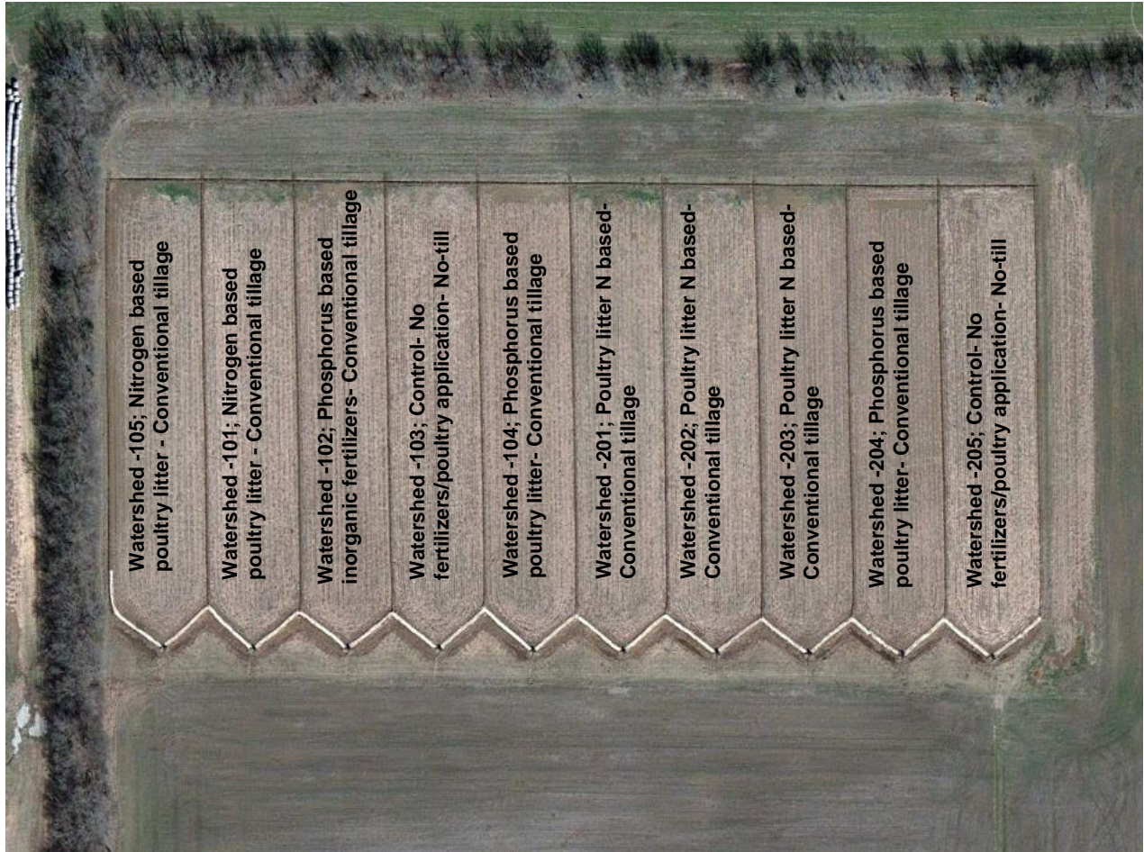
Figure A3: Watersheds layout at the Crawford County runoff study with management practices. Watersheds with nitrogen based turkey litter-notill treatment were not used in this study. The slope of the site was approximately 1%.
