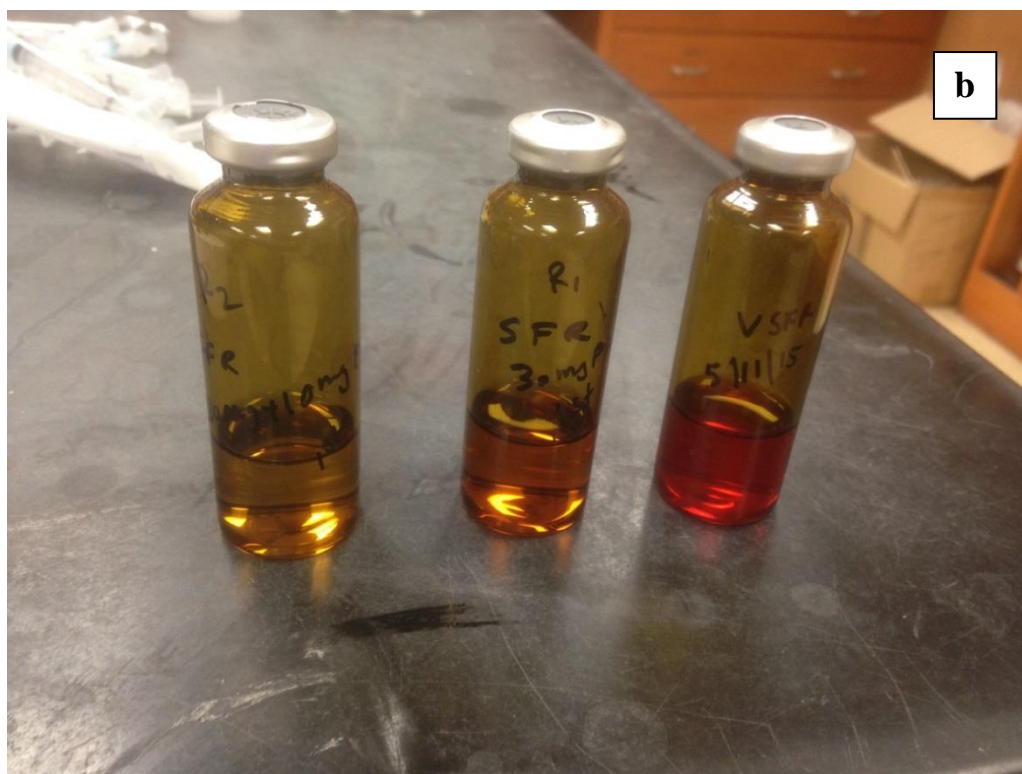
Figure F4. a) techniques showing deoxygenation (with helium gas), and re-vacuum of bottles b) Samples collected for reduced iron ( \text{Fe}^{2+} ) analysis
