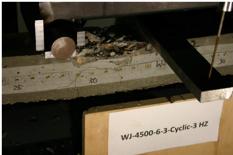
Figure 510 Picture of Failed Prism for WJ-4500-6-3-Cyclic
