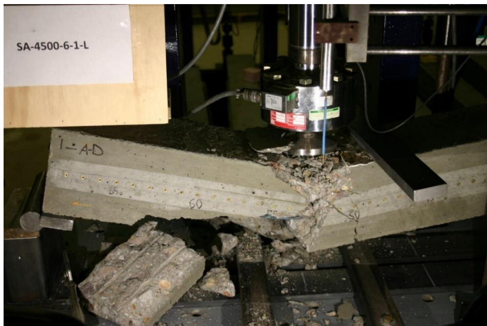
Figure 370 Picture of Failed Prism for SA-4500-6-1-L
