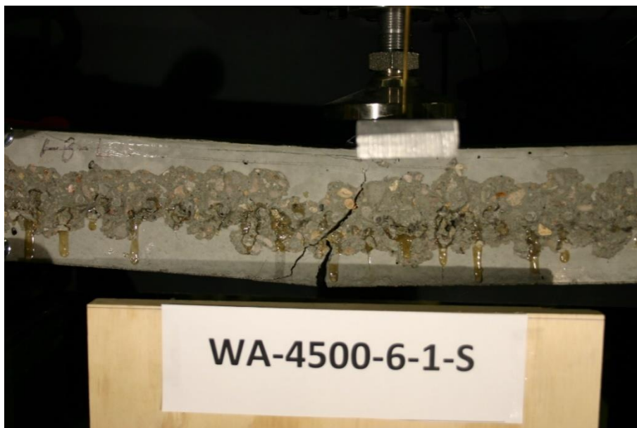
Figure 115 Picture of Failed Prism WA-4500-6-1-S
