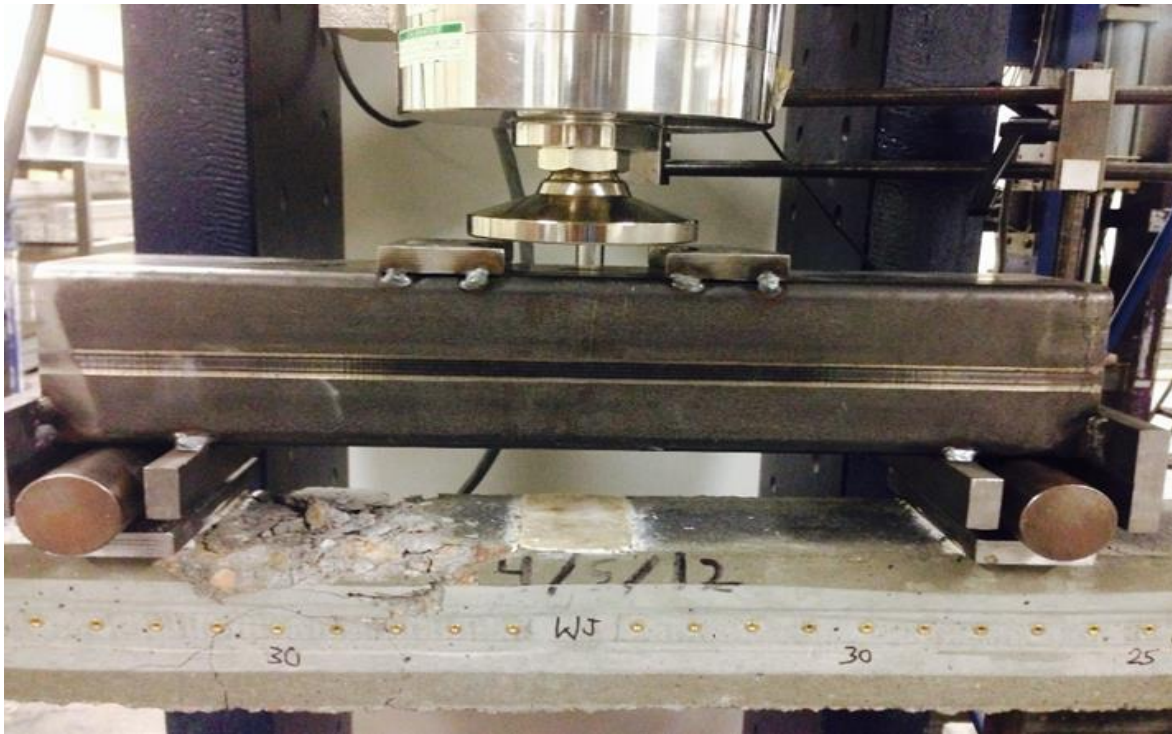
Figure 32. Spreader beam used to apply load to the pretensioned prism for cyclic loading test
