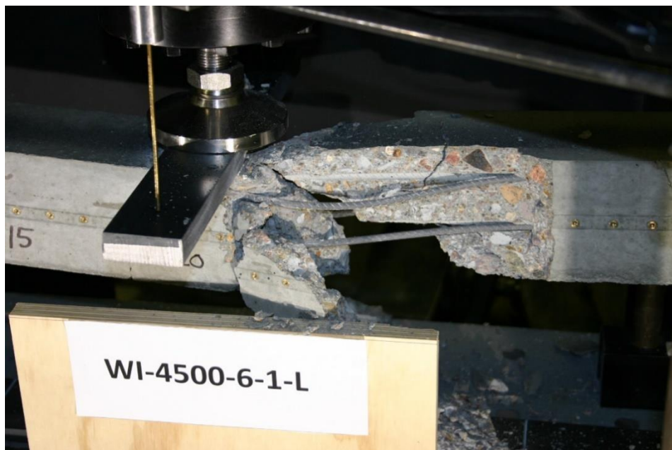
Figure 177 Picture of Failed Prism WI-4500-6-1-L
