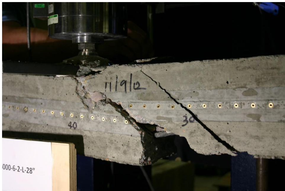
Figure 470 Picture of Failed Prism for SD-6000-6-2-L
