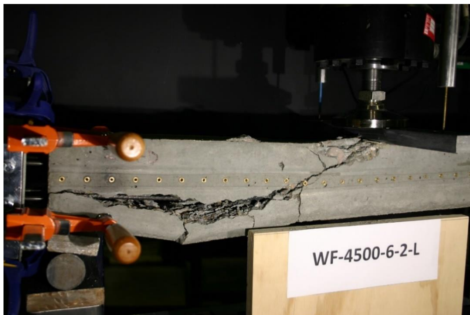
Figure 157 Picture of Failed Prism WF-4500-6-2-L
