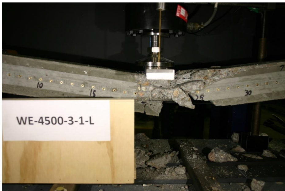
Figure 225 Picture of Failed Prism WE-4500-3-1-L
