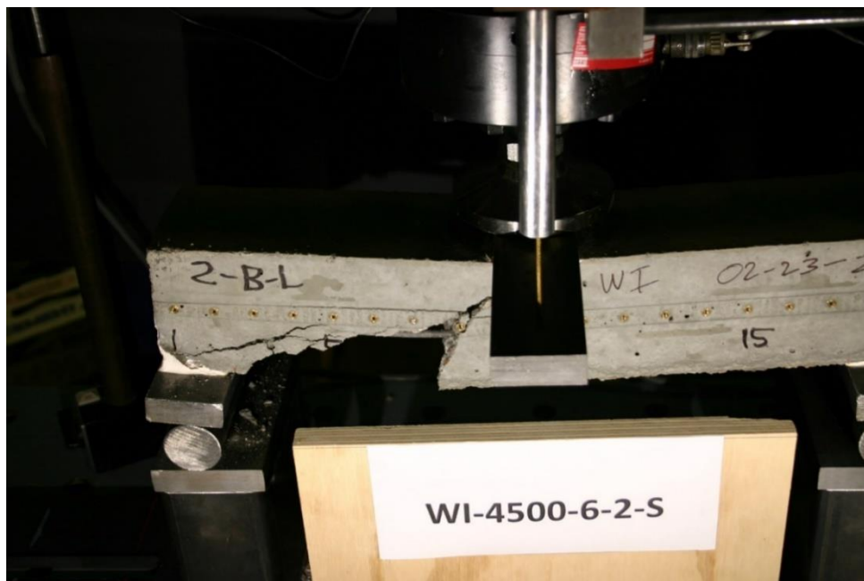
Figure 183 Picture of Failed Prism WI-4500-6-2-S
