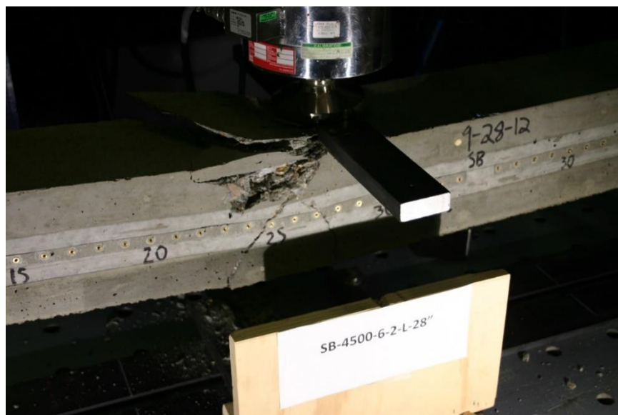
Figure 384 Picture of Failed Prism for SB-4500-6-2-L
