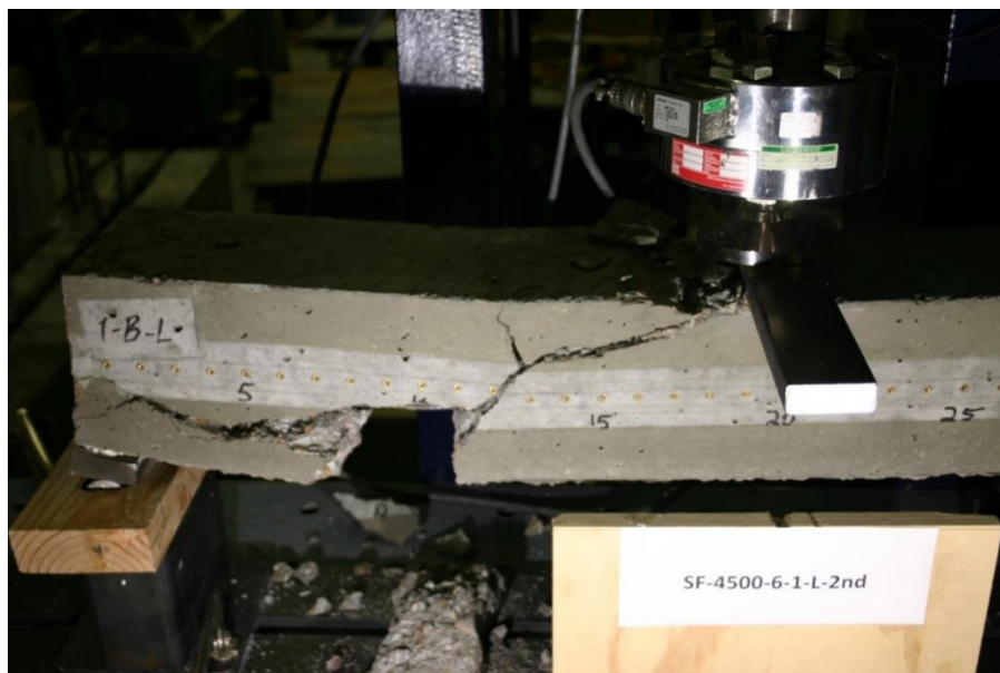
Figure 411 Picture of Failed Prism for SF-4500-6-1-L-2nd
