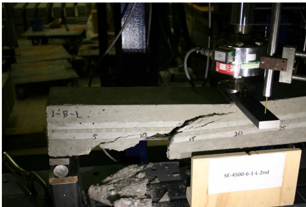
Figure 402 Picture of Failed Prism for SE-4500-6-1-L-2nd
