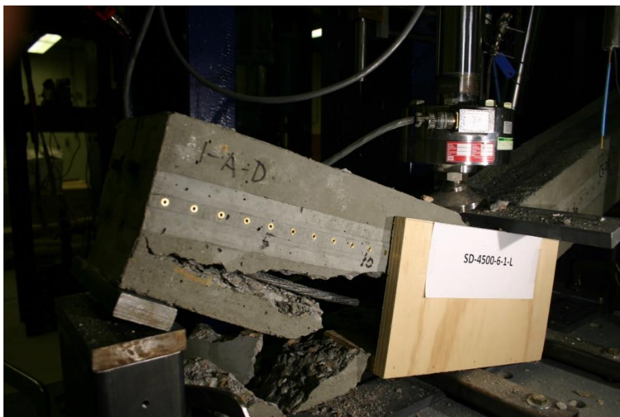
Figure 390 Picture of Failed Prism for SD-4500-6-1-L
