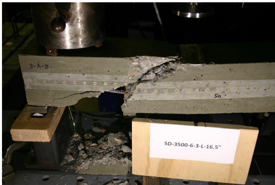
Figure 434 Picture of Failed Prism for SD-3500-6-3-L
