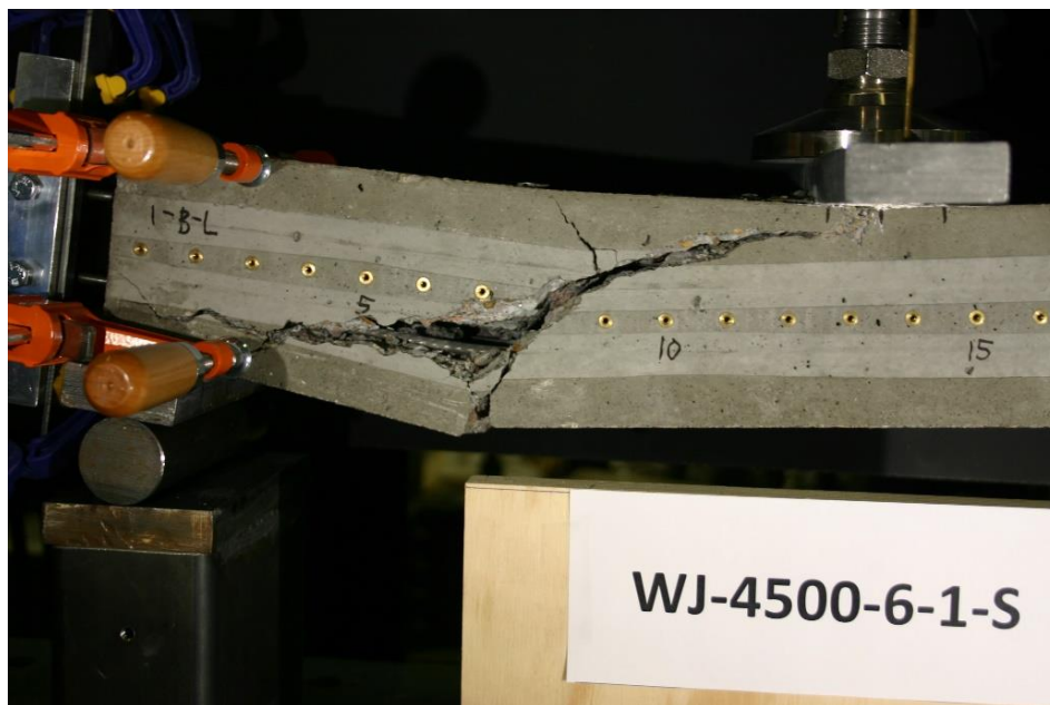
Figure 187 Picture of Failed Prism WJ-4500-6-1-S
