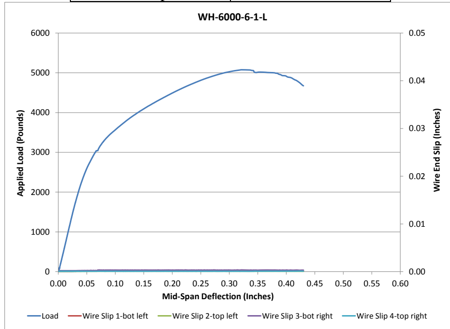
Figure 315 Load Deflection and Wire End Slip WH-6000-6-1-L
