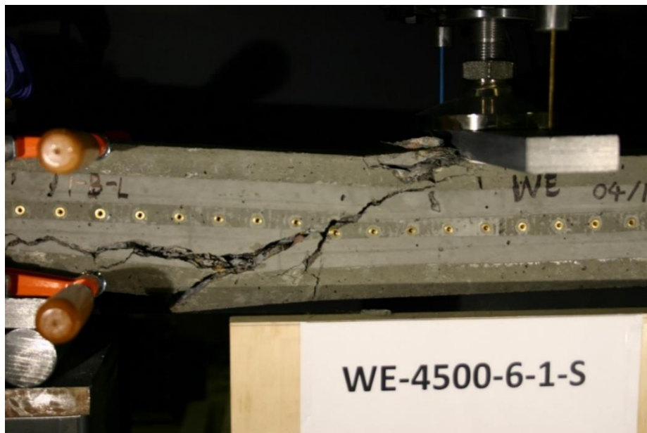
Figure 147 Picture of Failed Prism WE-4500-6-1-S
