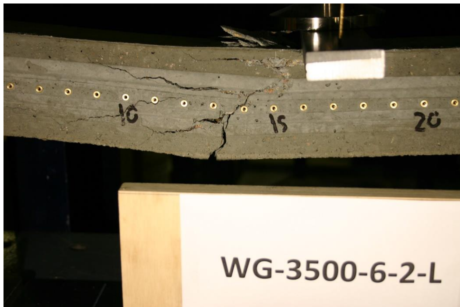
Figure 350 Picture of Failed Prism for WG-3500-6-2-L
