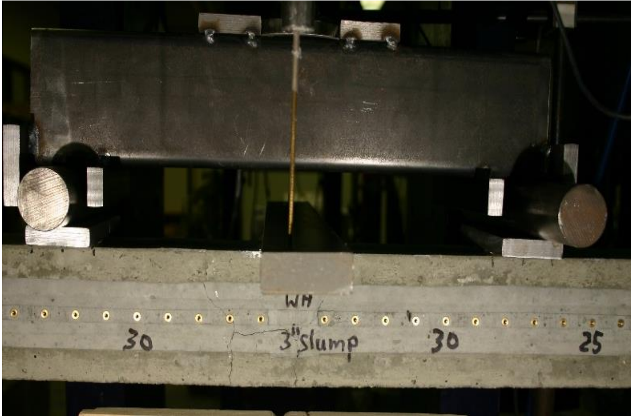
Figure 68. Prism made with WH wire failed at 89,875th cycle of loading (repeated test)
