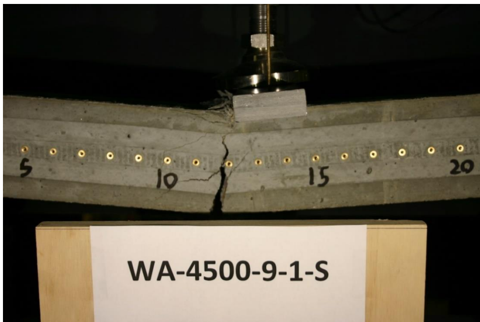
Figure 255 Picture of Failed Prism WA-4500-9-1-S
