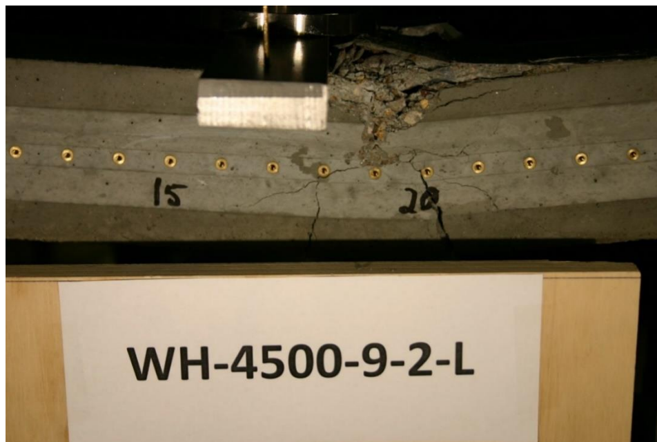
Figure 281 Picture of Failed Prism WH-4500-9-2-L
