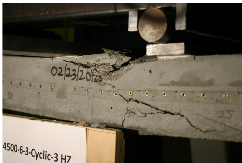
Figure 508 Picture of Failed Prism for WI-4500-6-3-Cyclic
