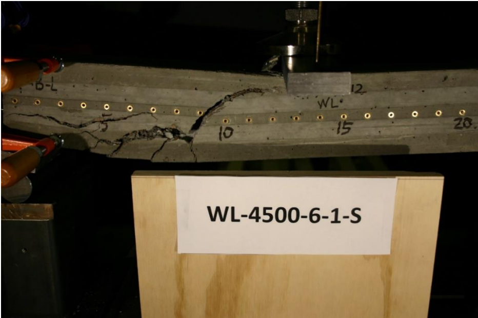
Figure 203 Picture of Failed Prism WL-4500-6-1-S
