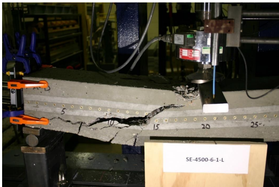
Figure 400 Picture of Failed Prism for SE-4500-6-1-L
