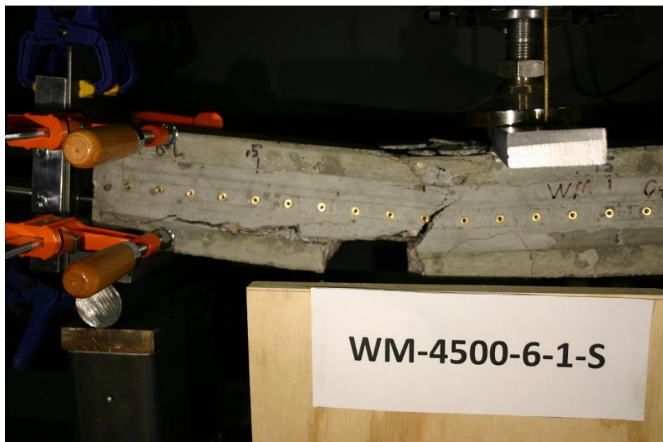
Figure 211 Picture of Failed Prism WM-4500-6-1-S
