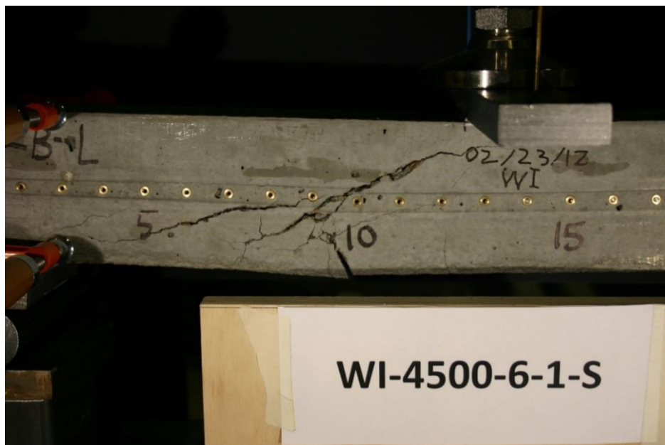
Figure 179 Picture of Failed Prism WI-4500-6-1-S
