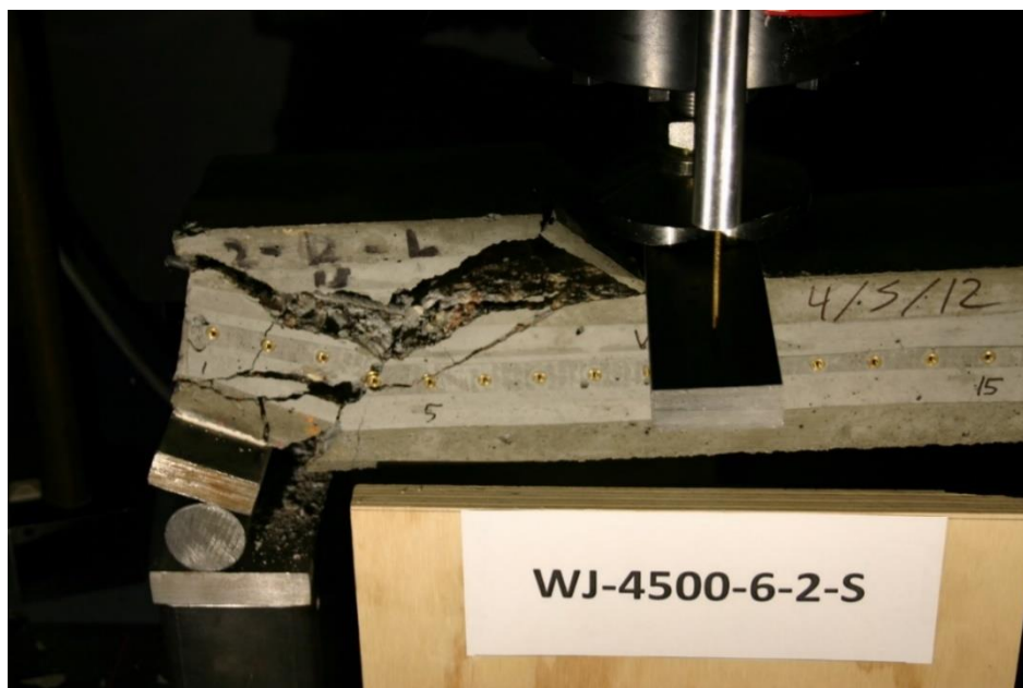
Figure 191 Picture of Failed Prism WJ-4500-6-2-S
