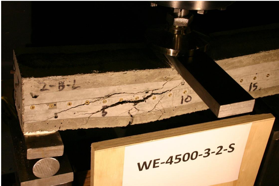
Figure 230 Picture of Failed Prism WE-4500-3-2-S
