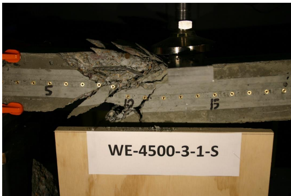
Figure 227 Picture of Failed Prism WE-4500-3-1-S
