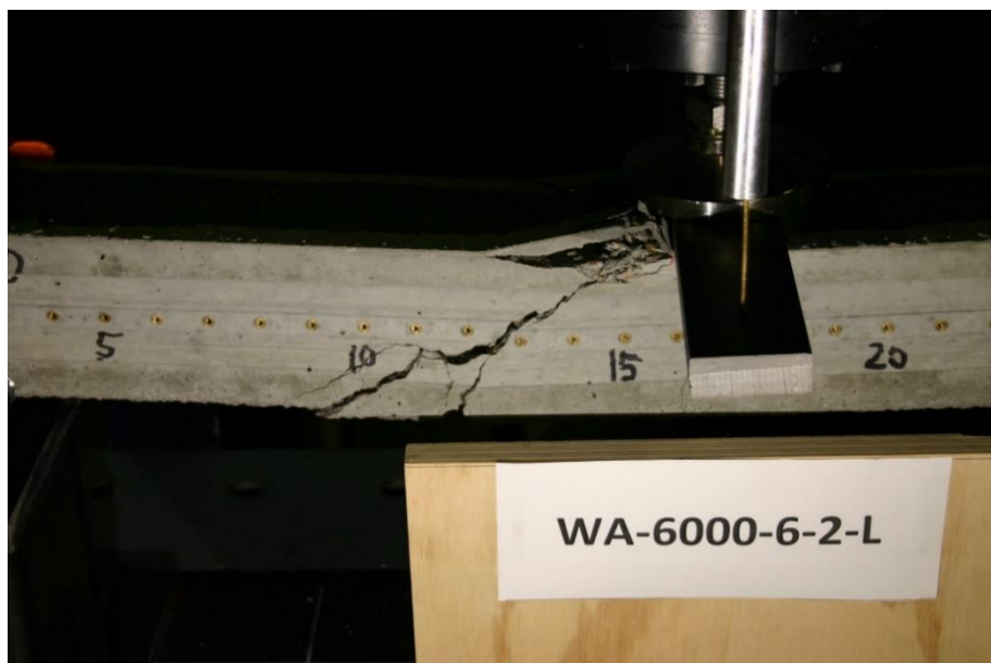
Figure 297 Picture of Failed Prism WA-6000-6-2-L
