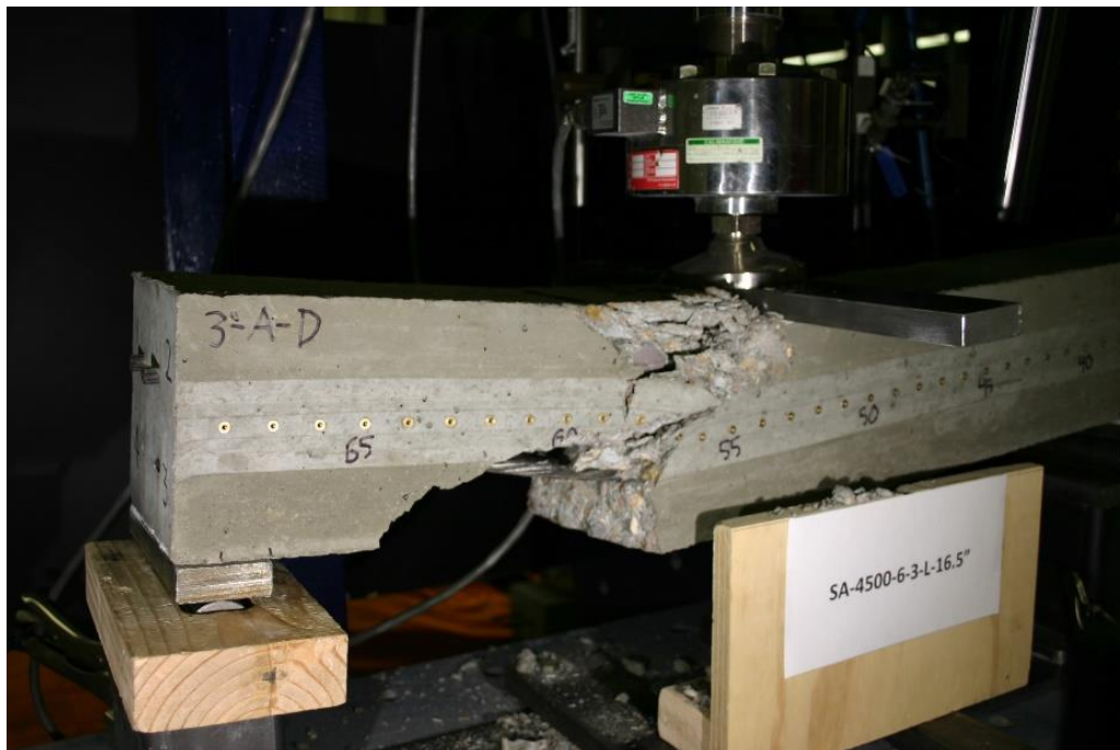
Figure 376 Picture of Failed Prism for SA-4500-6-3-L
