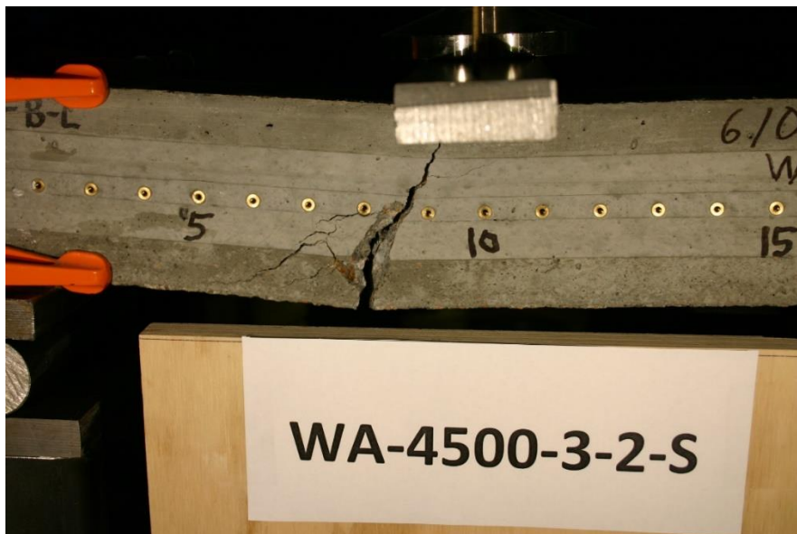
Figure 223 Picture of Failed Prism WA-4500-3-2-S
