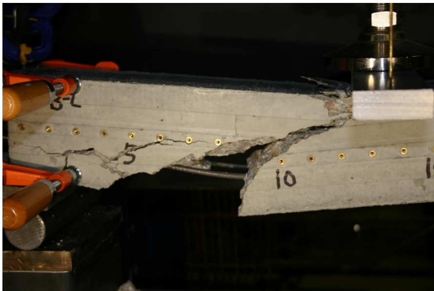
Figure 326 Picture of Failed Prism WK-6000-6-1-S
