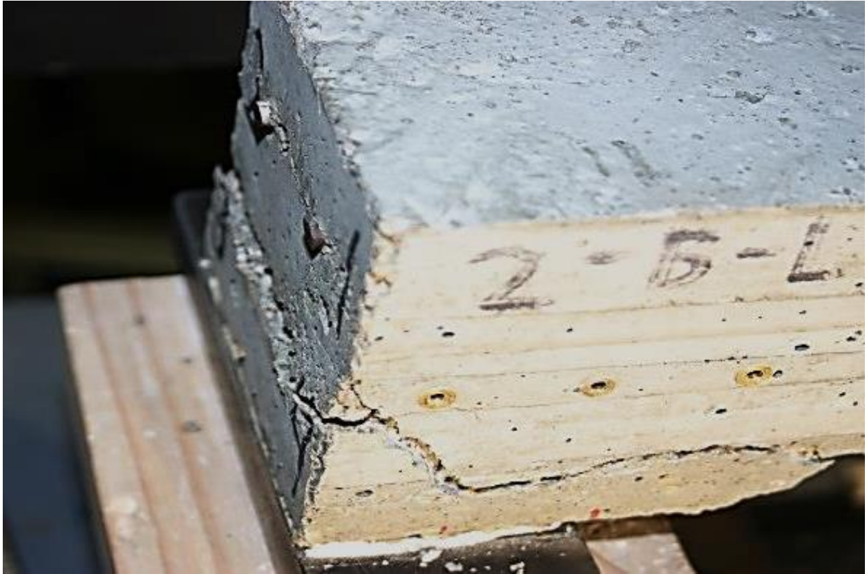
Figure 19. Horizontal-splitting mode where the prism split along the bottom row of prestress wires
