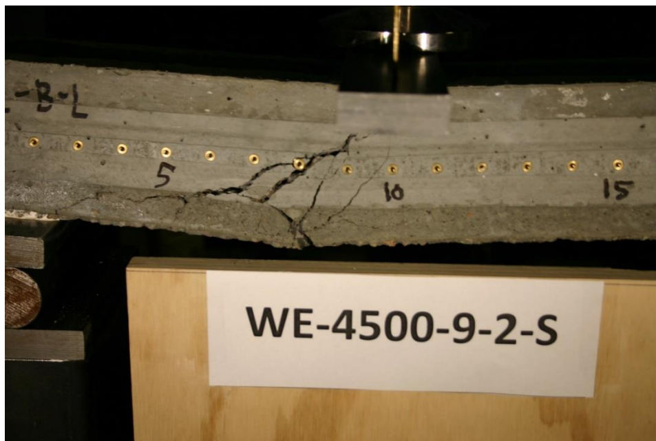
Figure 267 Picture of Failed Prism WE-4500-9-2-S
