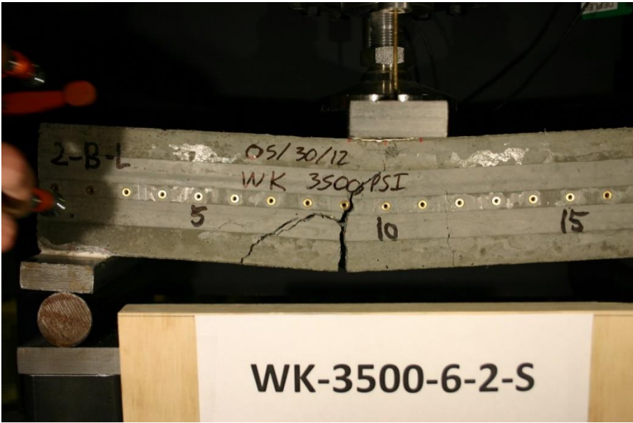
Figure 368 Picture of Failed Prism for WK-3500-6-2-S
