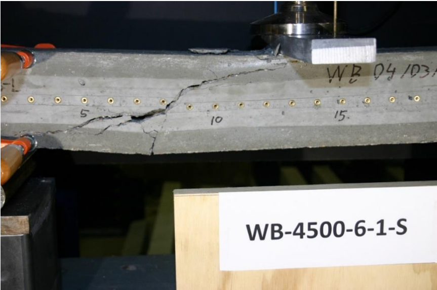
Figure 123 Picture of Failed Prism WB-4500-6-1-S
