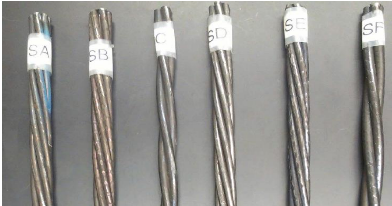
Figure 23. Sample of six strands with different indentation types and diameters [after: (Arnold, 2013)]
