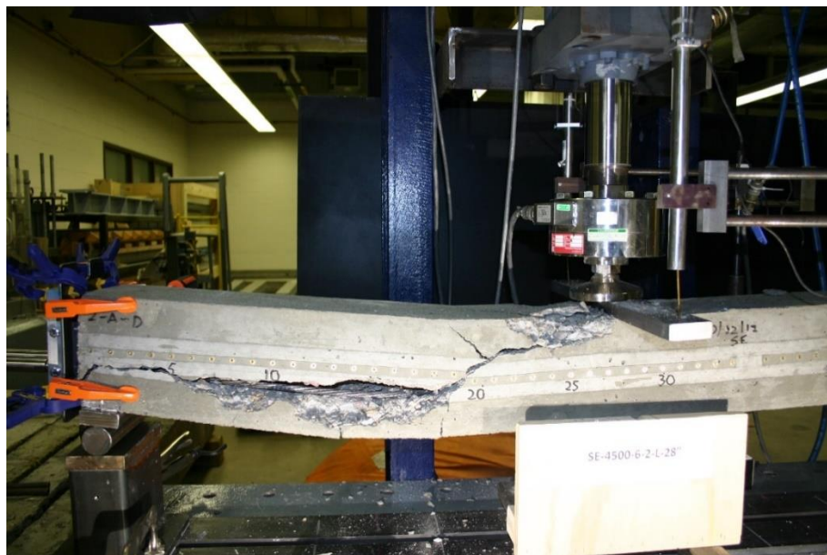
Figure 404 Picture of Failed Prism for SE-4500-6-2-L
