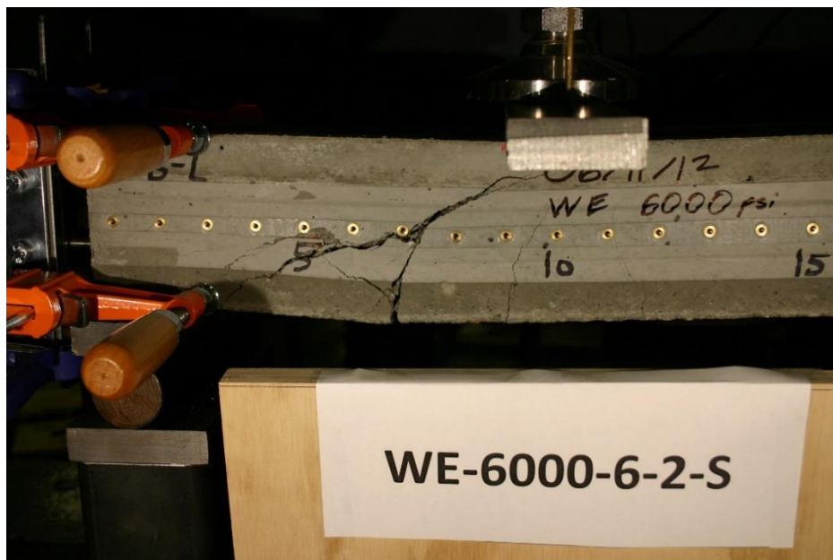
Figure 306 Picture of Failed Prism WE-6000-6-2-S
