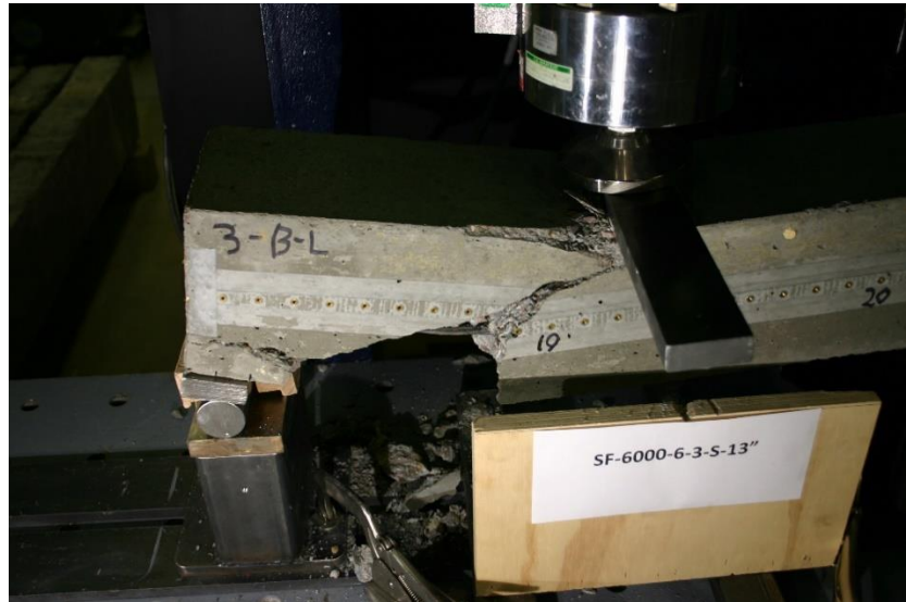
Figure 492 Picture of Failed Prism for SF-6000-6-3-S
