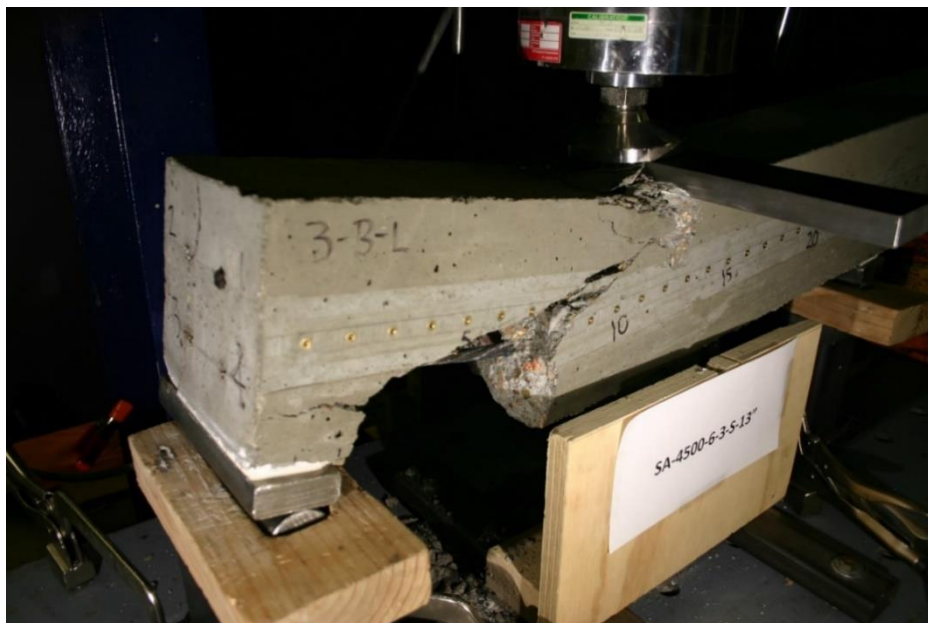
Figure 378 Picture of Failed Prism for SA-4500-6-3-S
