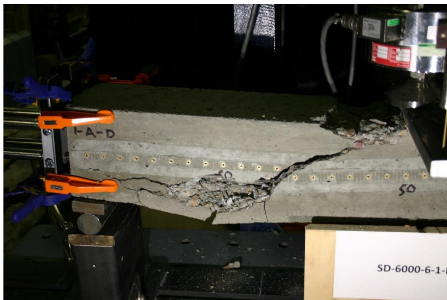
Figure 466 Picture of Failed Prism for SD-6000-6-1-L
