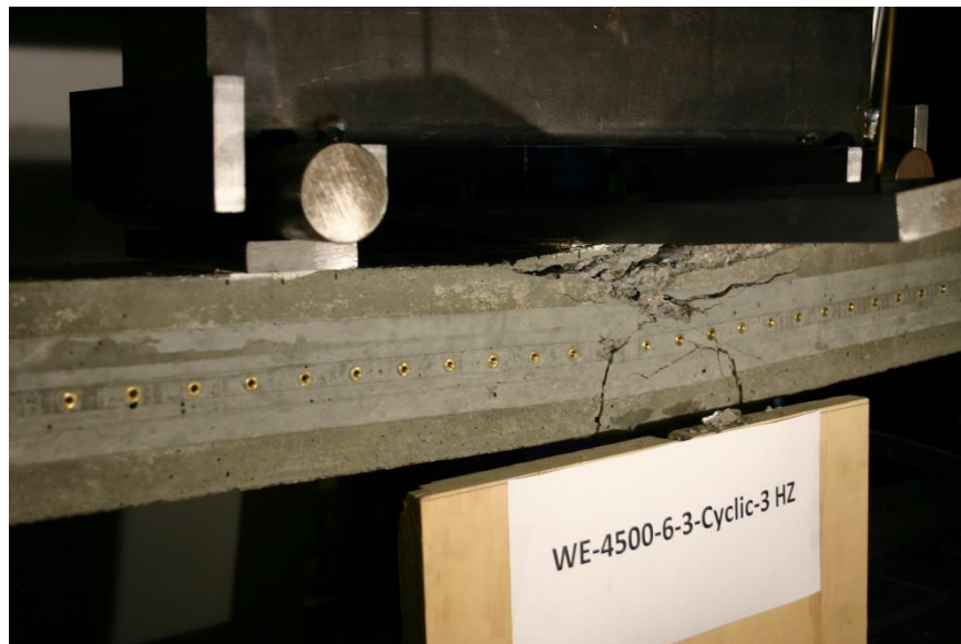
Figure 501 Picture of Failed Prism for WE-4500-6-3-Cyclic
