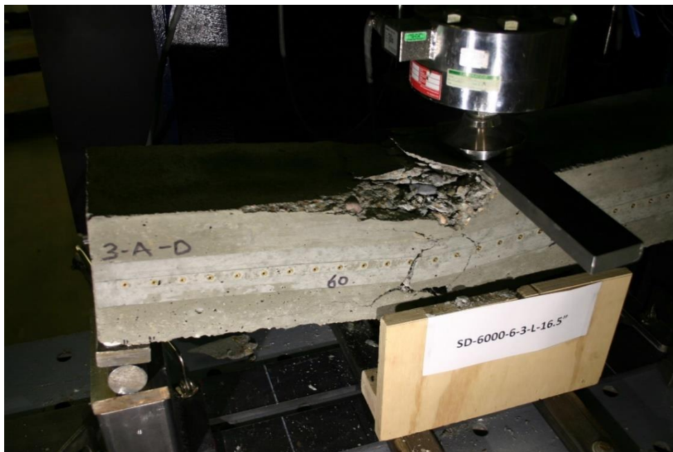
Figure 472 Picture of Failed Prism for SD-6000-6-3-L
