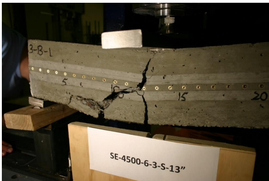
Figure 407 Picture of Failed Prism for SE-4500-6-3-S
