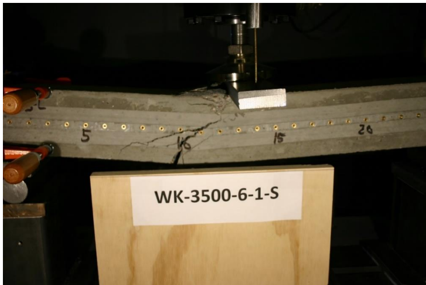
Figure 364 Picture of Failed Prism for WK-3500-6-1-S
