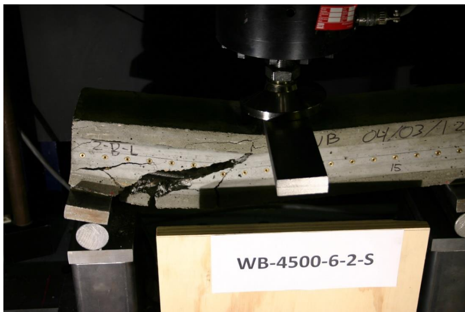
Figure 127 Picture of Failed Prism WB-4500-6-2-S
