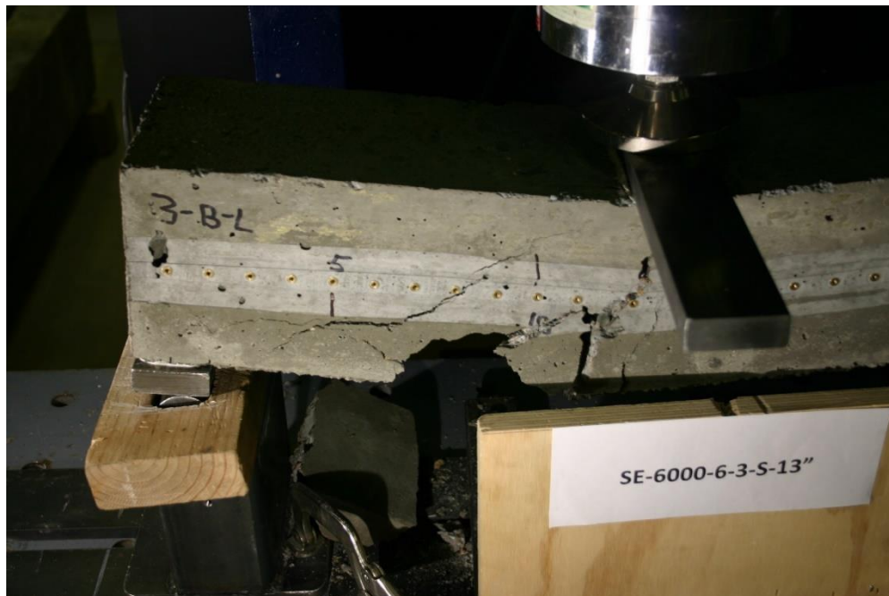
Figure 483 Picture of Failed Prism for SE-6000-6-3-S
