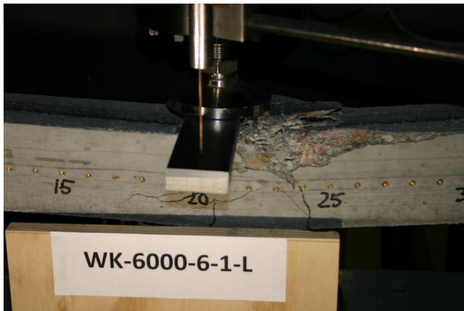
Figure 324 Picture of Failed Prism WK-6000-6-1-L
