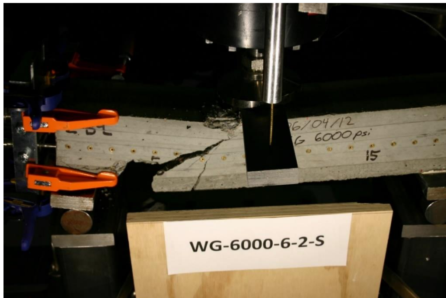
Figure 314 Picture of Failed Prism WG-6000-6-2-S
