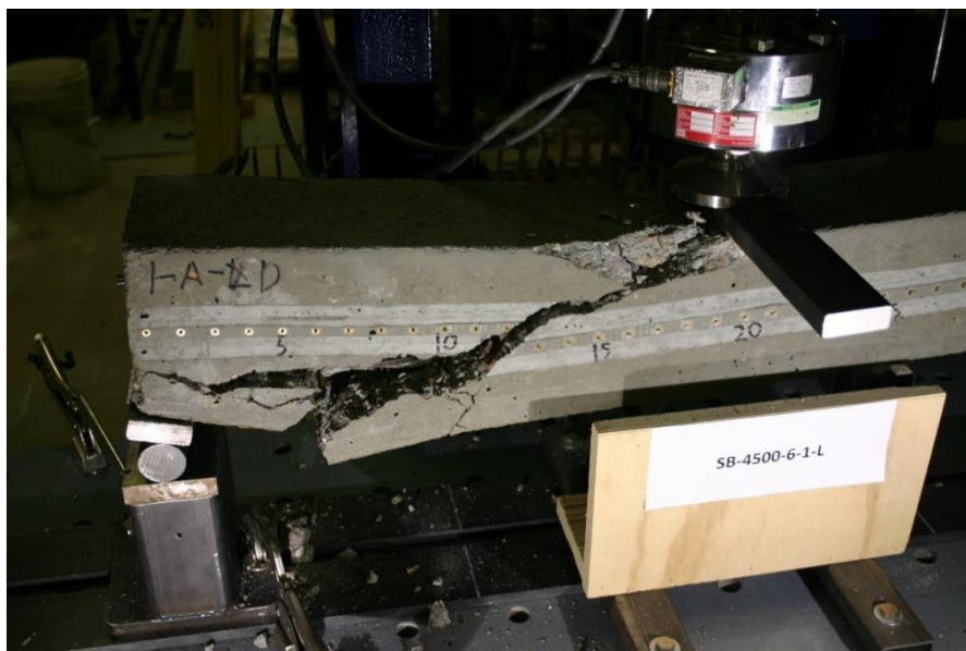
Figure 380 Picture of Failed Prism for SB-4500-6-1-L
