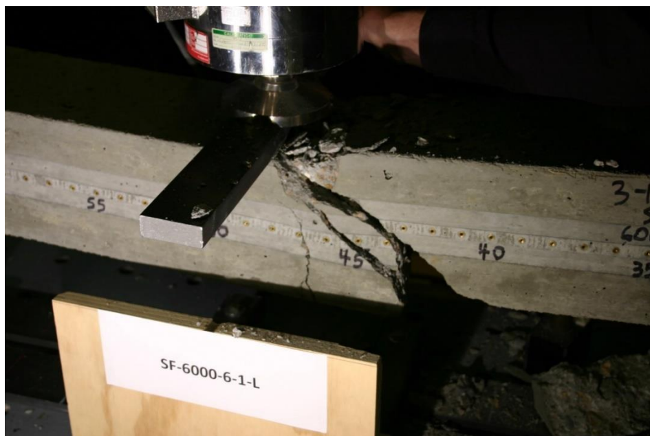
Figure 485 Picture of Failed Prism for SF-6000-6-1-L
