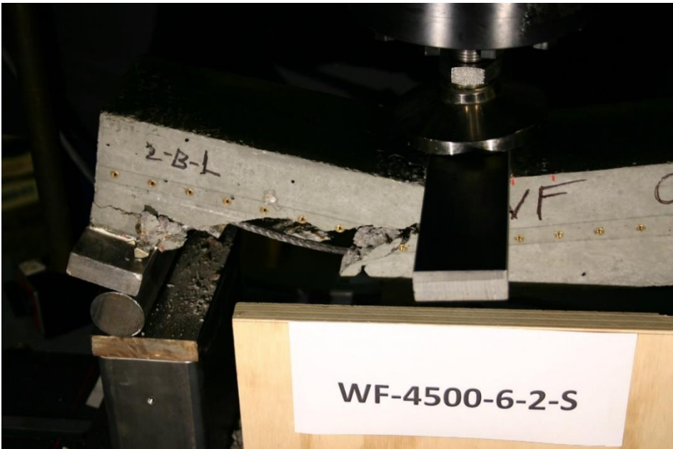
Figure 159 Picture of Failed Prism WF-4500-6-2-S
