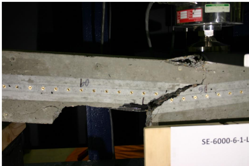
Figure 476 Picture of Failed Prism for SE-6000-6-1-L
