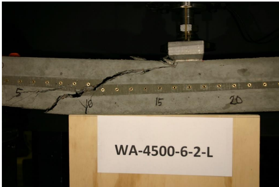
Figure 117 Picture of Failed Prism WA-4500-6-2-L
