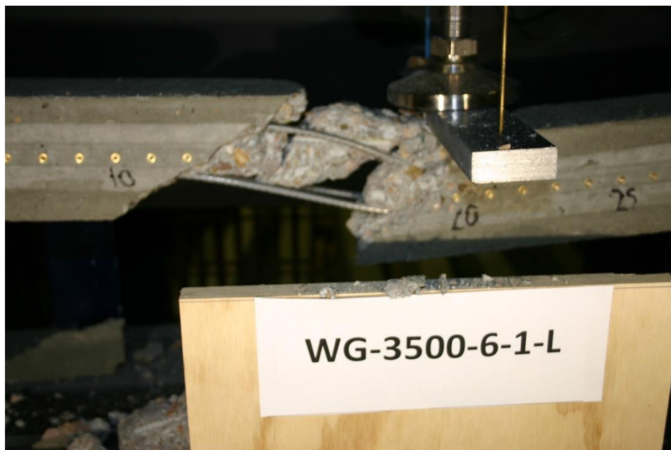
Figure 347 Picture of Failed Prism for WG-3500-6-1-L
