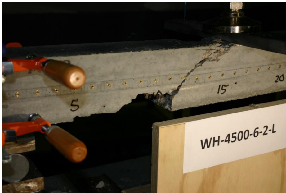
Figure 173 Picture of Failed Prism WH-4500-6-2-L
