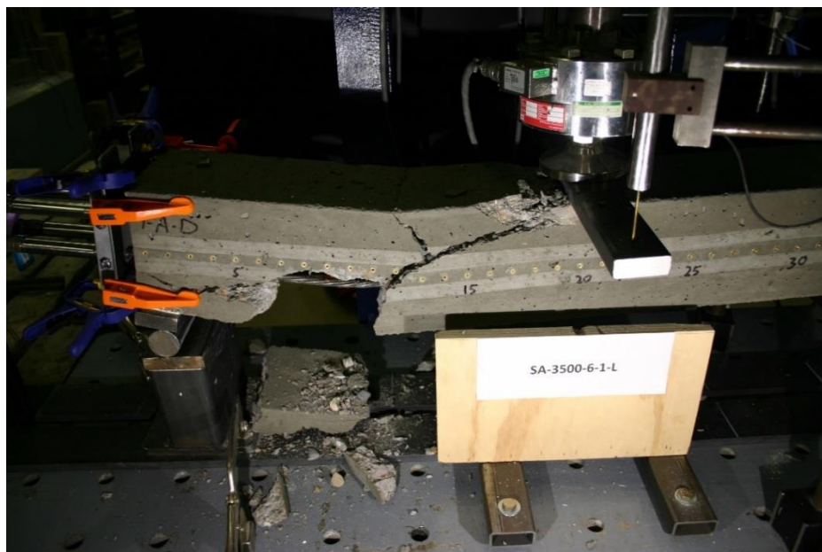
Figure 419 Picture of Failed Prism for SA-3500-6-1-L
