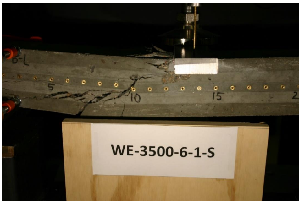
Figure 341 Picture of Failed Prism for WE-3500-6-1-S
