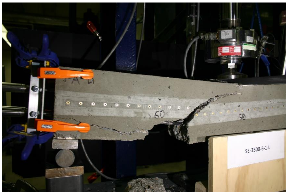
Figure 438 Picture of Failed Prism for SE-3500-6-1-L
