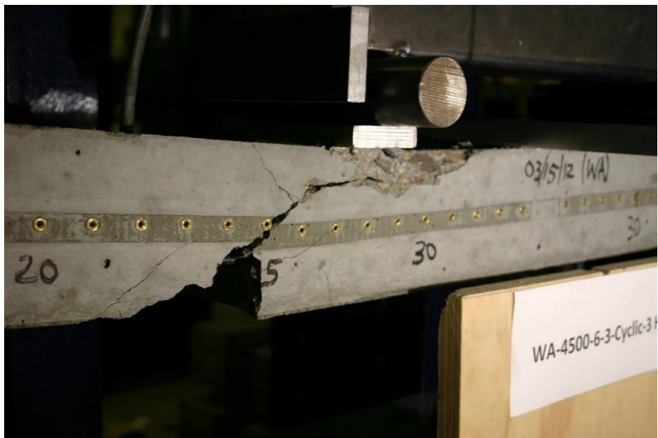
Figure 494 Picture of Failed Prism for WA-4500-6-3-Cyclic
