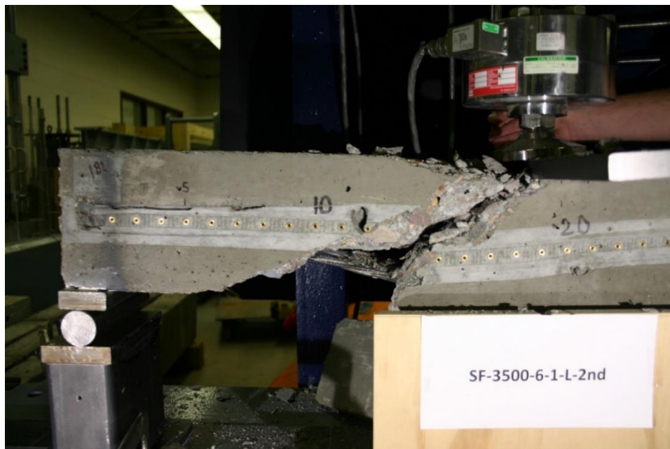
Figure 449 Picture of Failed Prism for SF-3500-6-1-L-2nd
