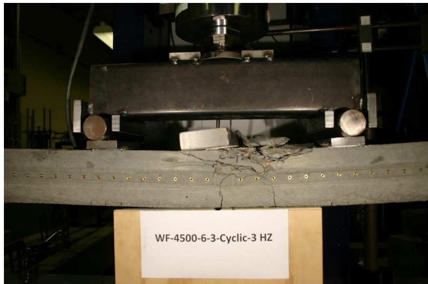
Figure 503 Picture of Failed Prism for WF-4500-6-3-Cyclic
