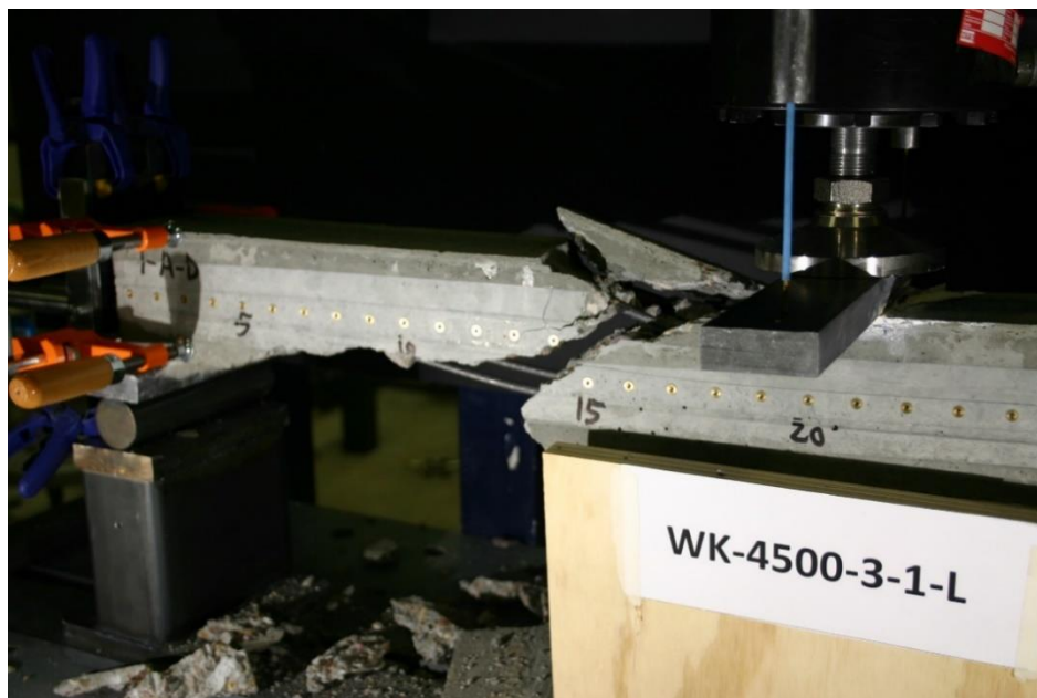
Figure 245 Picture of Failed Prism WK-4500-3-1-L
