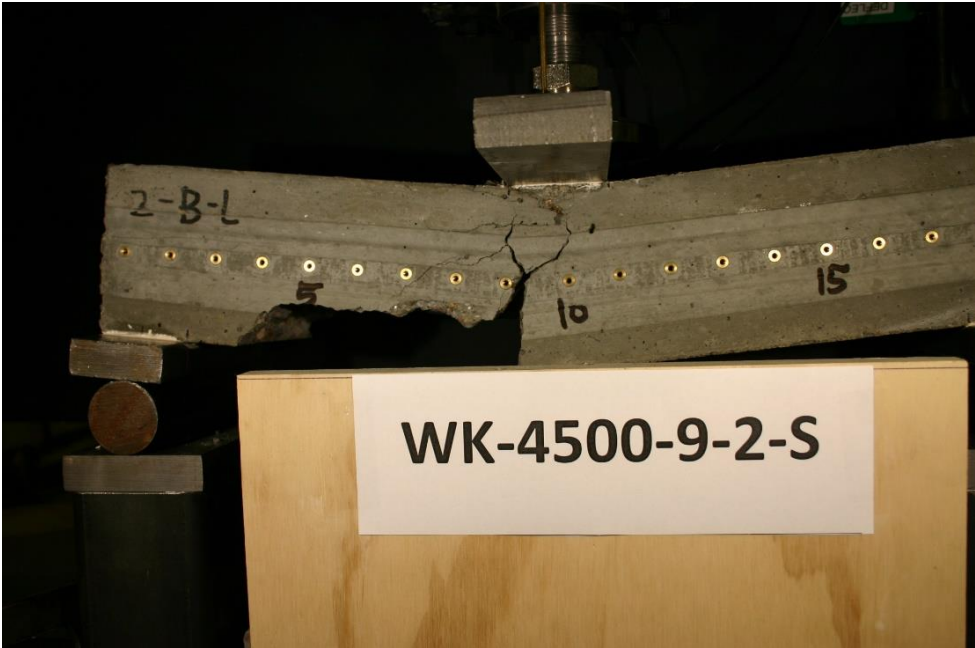
Figure 291 Picture of Failed Prism WK-4500-9-2-S
