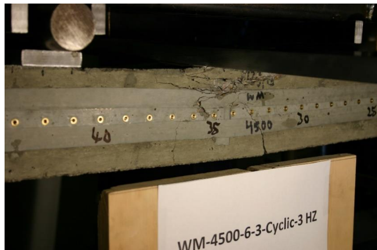
Figure 516 Picture of Failed Prism for WM-4500-6-3-Cyclic
