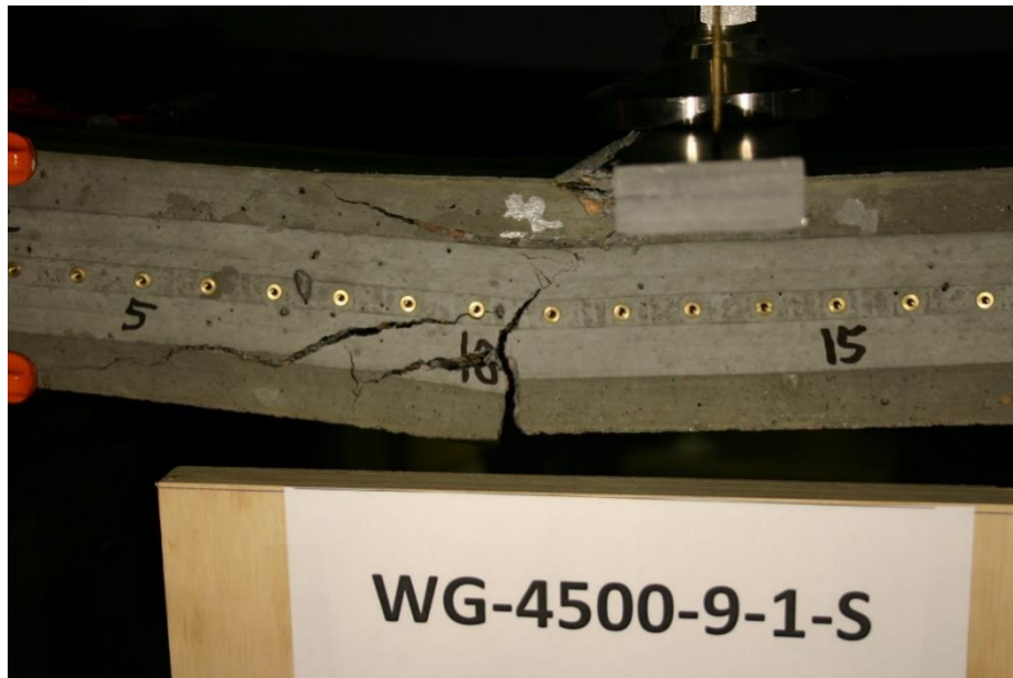
Figure 271 Picture of Failed Prism WG-4500-9-1-S
