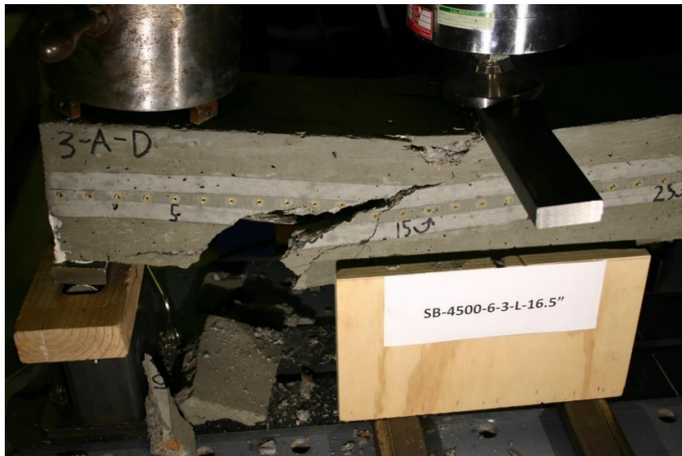
Figure 386 Picture of Failed Prism for SB-4500-6-3-L
