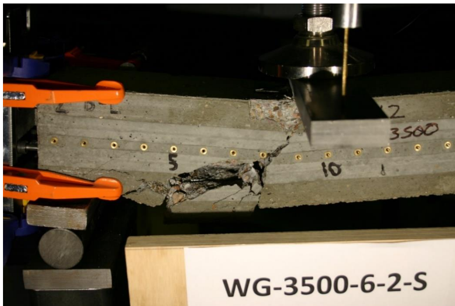
Figure 352 Picture of Failed Prism for WG-3500-6-2-S
