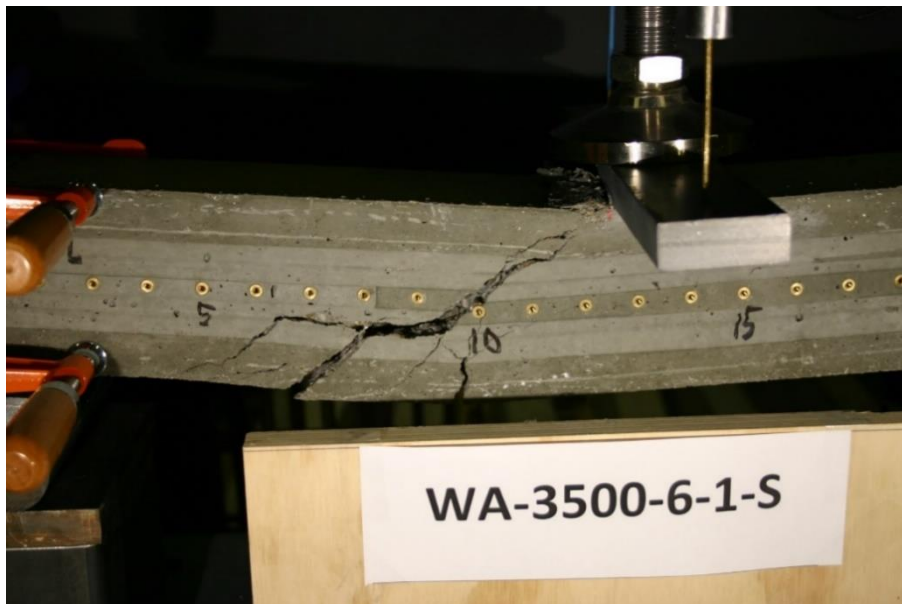
Figure 334 Picture of Failed Prism WA-3500-6-1-S
