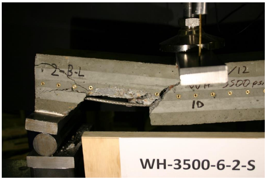
Figure 360 Picture of Failed Prism for WH-3500-6-2-S
