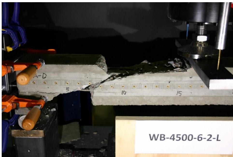
Figure 125 Picture of Failed Prism WB-4500-6-2-L
