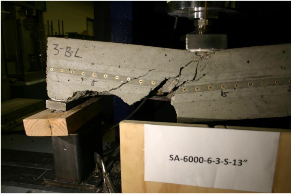
Figure 464 Picture of Failed Prism for SA-6000-6-3-S
