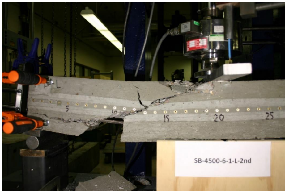
Figure 382 Picture of Failed Prism for SB-4500-6-1-L-2 nd
