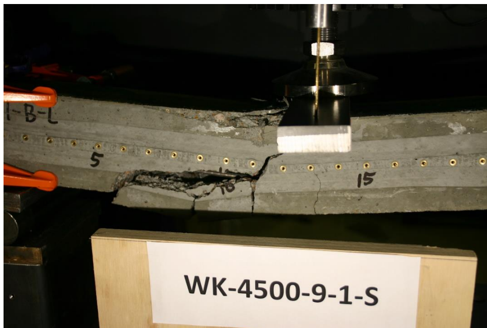
Figure 287 Picture of Failed Prism WK-4500-9-1-S
