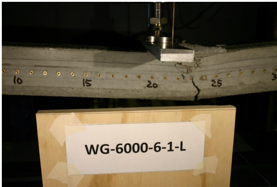
Figure 308 Picture of Failed Prism WG-6000-6-1-L
