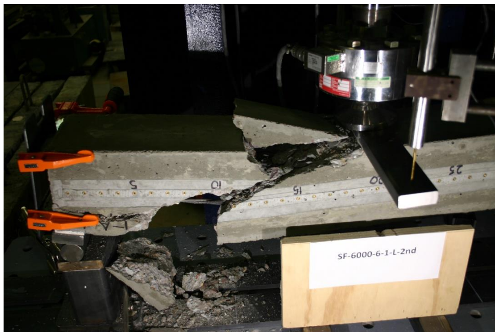
Figure 487 Picture of Failed Prism for SF-6000-6-1-L-2nd
