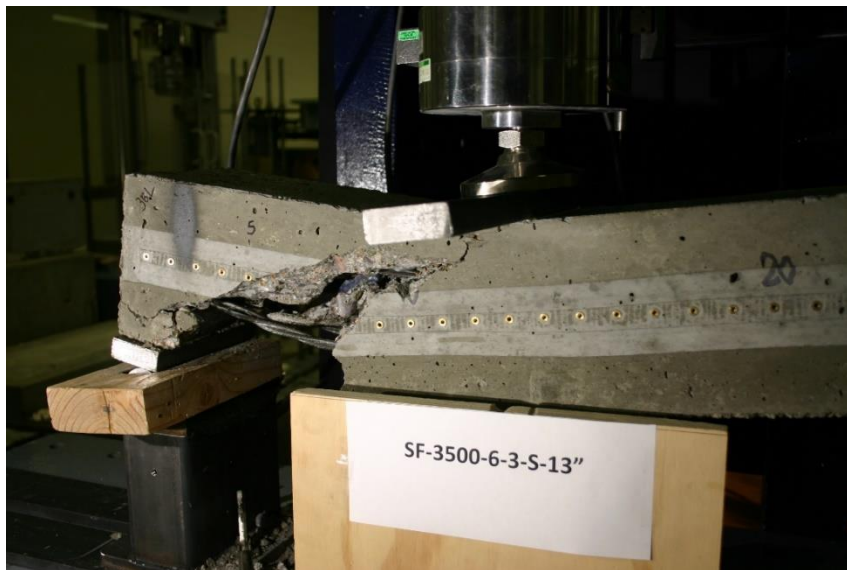
Figure 454 Picture of Failed Prism for SF-3500-6-3-S
