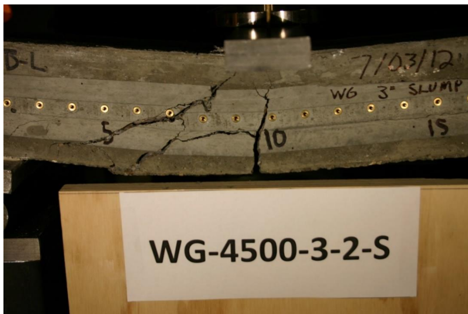
Figure 238 Picture of Failed Prism WG-4500-3-2-S
