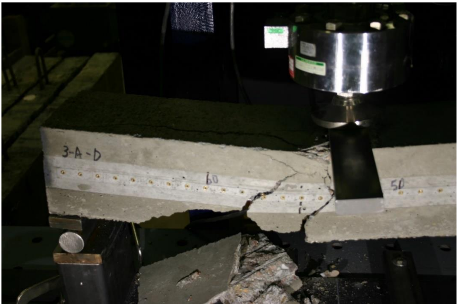
Figure 481 Picture of Failed Prism for SE-6000-6-3-L
