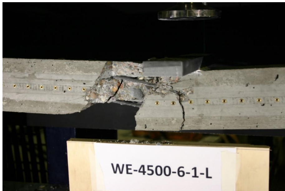
Figure 145 Picture of Failed Prism WE-4500-6-1-L
