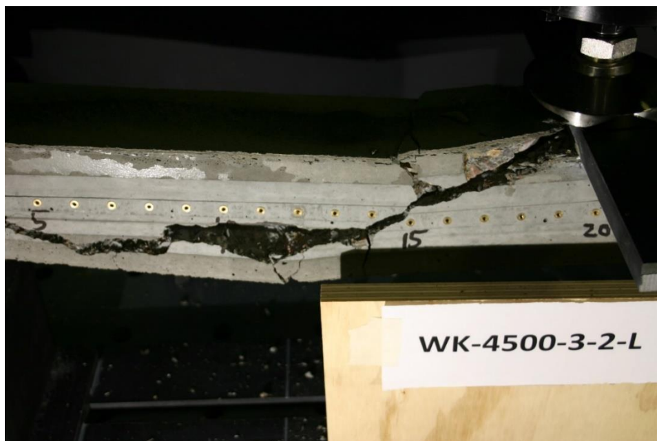
Figure 249 Picture of Failed Prism WK-4500-3-2-L
