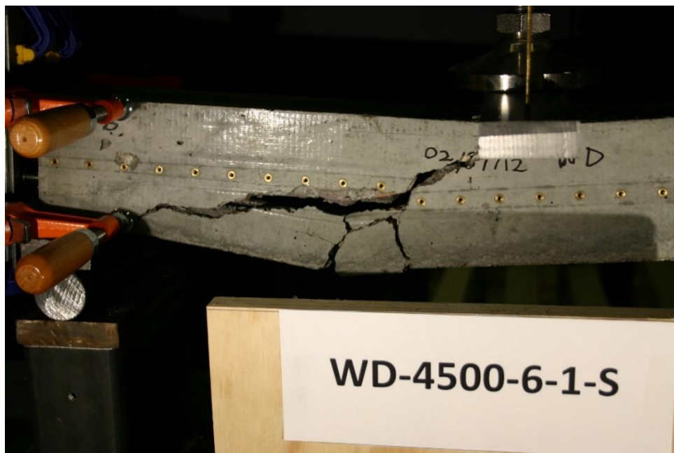
Figure 139 Picture of Failed Prism WD-4500-6-1-S
