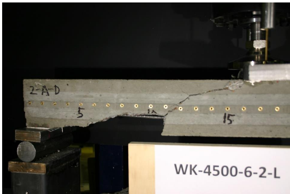
Figure 197 Picture of Failed Prism WK-4500-6-2-L
