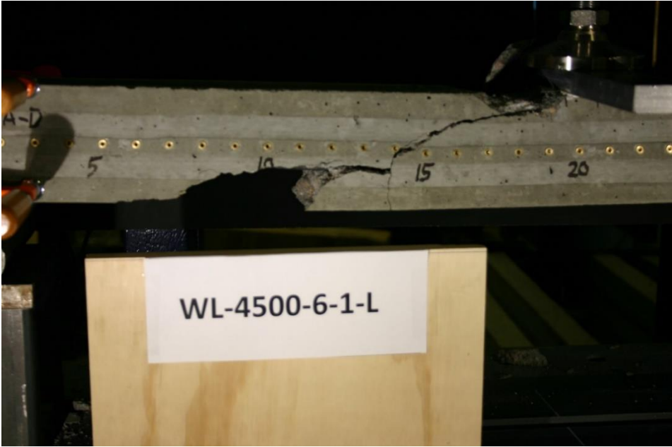
Figure 201 Picture of Failed Prism WL-4500-6-1-L
