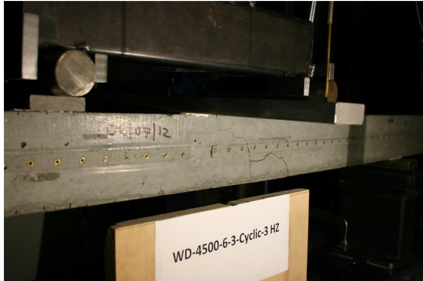
Figure 499 Picture of Failed Prism for WD-4500-6-3-Cyclic
