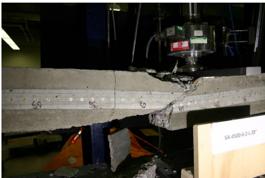
Figure 374 Picture of Failed Prism for SA-4500-6-2-L
