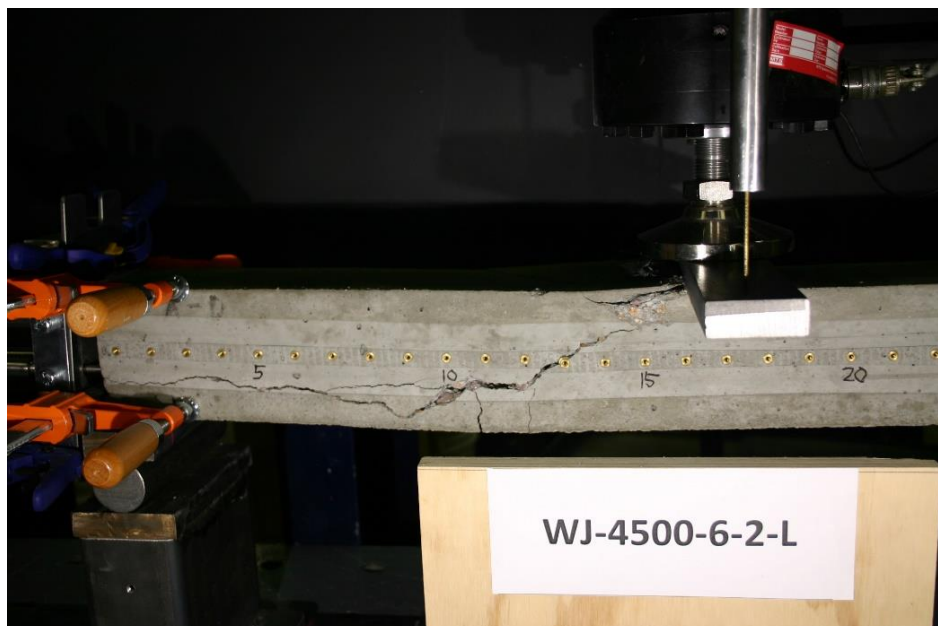
Figure 189 Picture of Failed Prism WJ-4500-6-2-L
