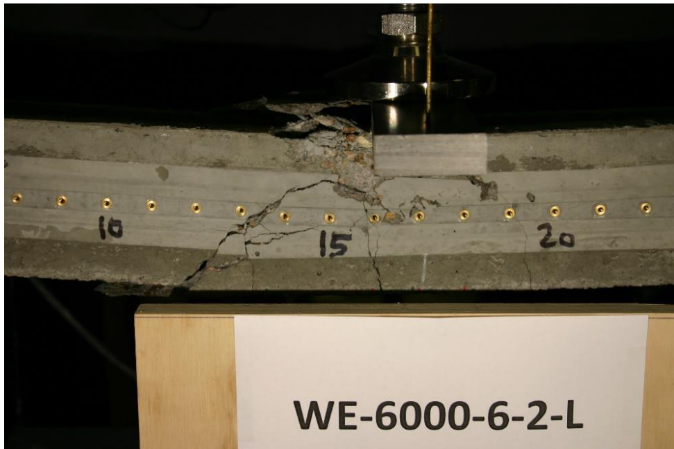
Figure 304 Picture of Failed Prism WE-6000-6-2-L
