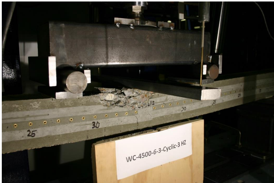
Figure 498 Picture of Failed Prism for WC-4500-6-3-Cyclic
