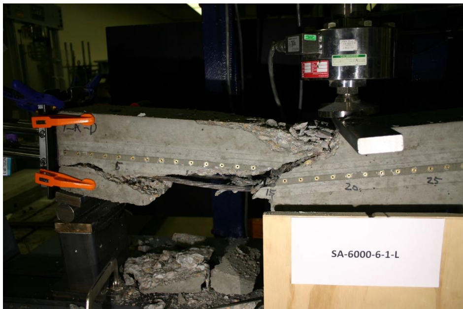
Figure 456 Picture of Failed Prism for SA-6000-6-1-L
