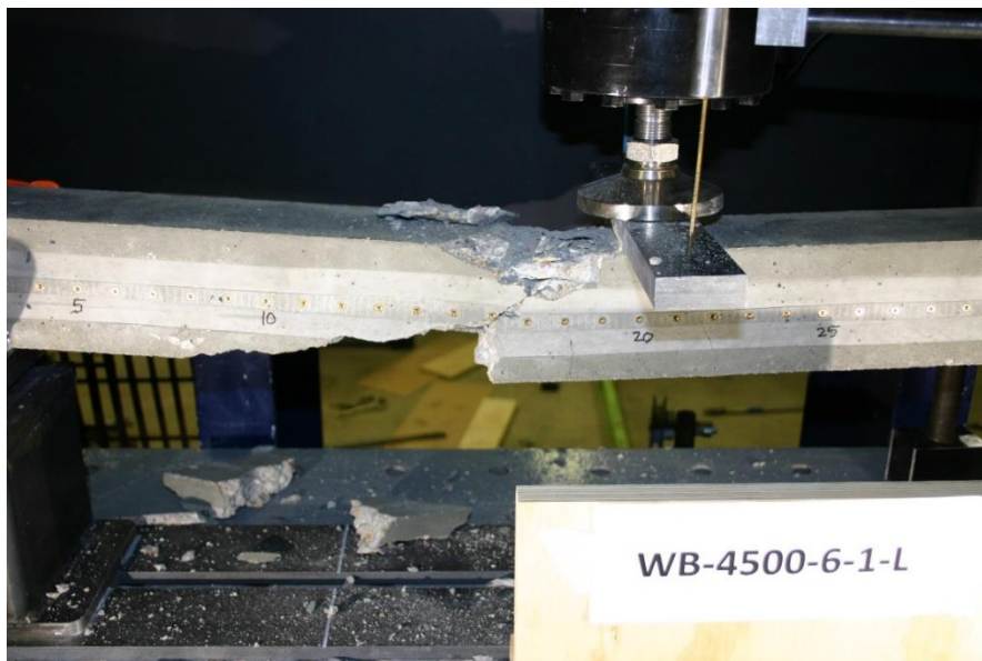
Figure 121 Picture of Failed Prism WB-4500-6-1-L
