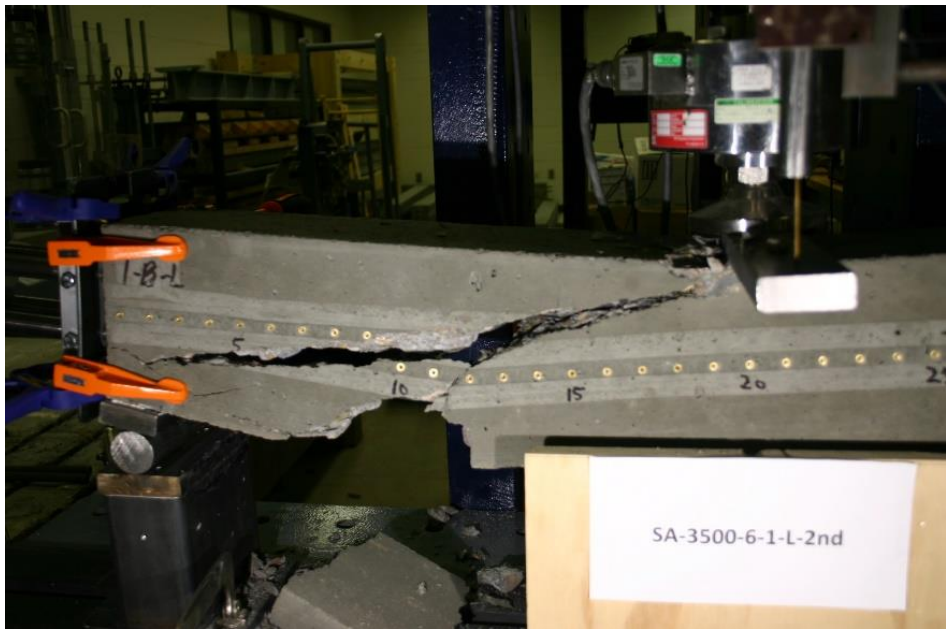
Figure 420 Picture of Failed Prism for SA-3500-6-1-L-2 nd
