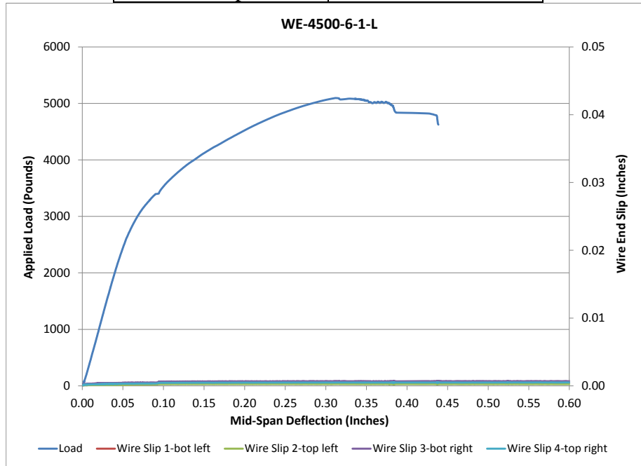
Figure 144 Load Deflection and Wire End Slip WE-4500-6-1-L
