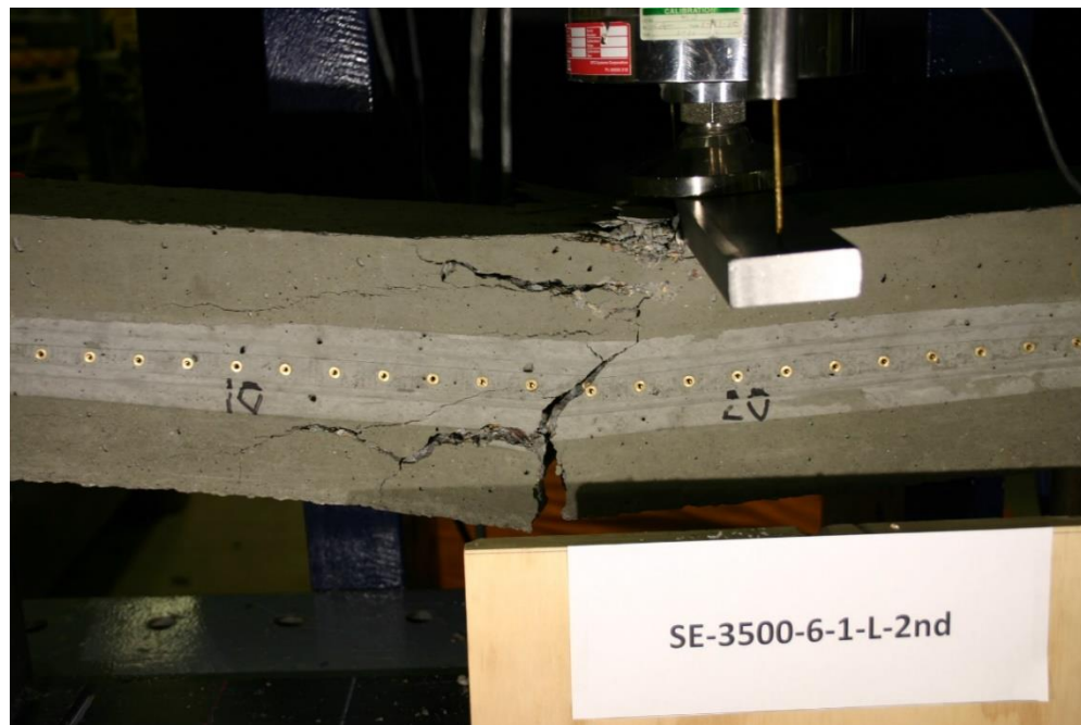
Figure 440 Picture of Failed Prism for SE-3500-6-1-L-2nd
