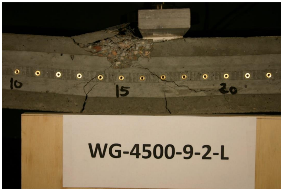
Figure 273 Picture of Failed Prism WG-4500-9-2-L
