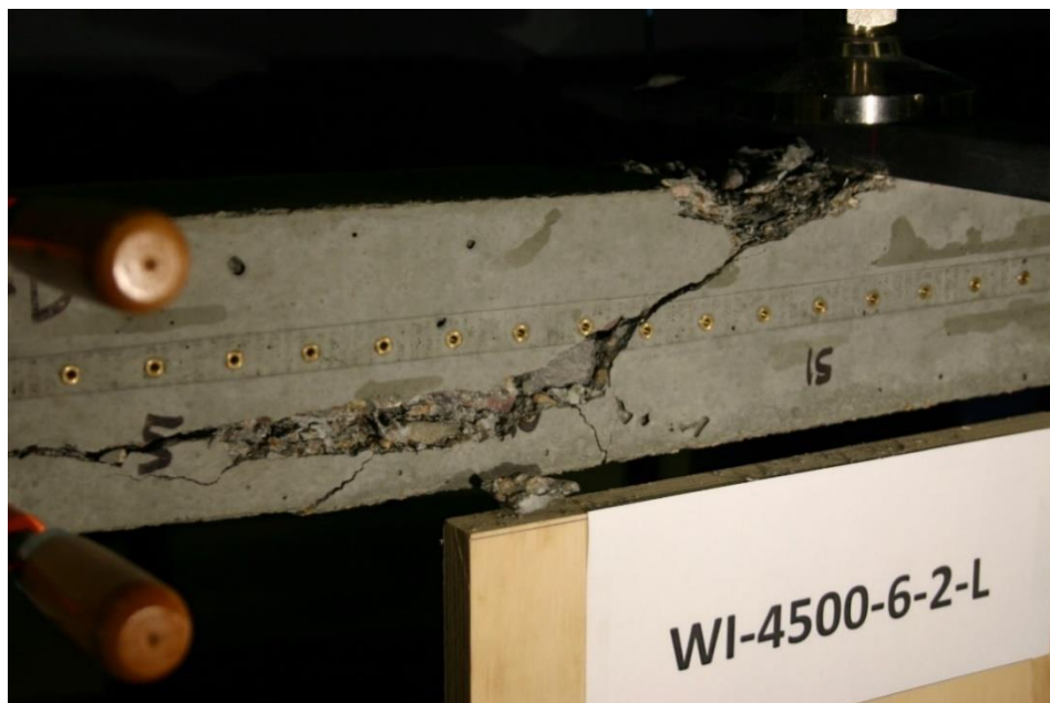
Figure 181 Picture of Failed Prism WI-4500-6-2-L
