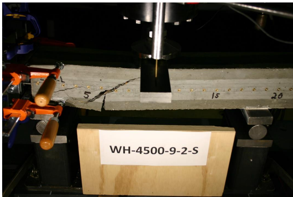
Figure 283 Picture of Failed Prism WH-4500-9-2-S
