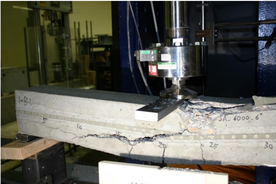
Figure 458 Picture of Failed Prism for SA-6000-6-1-L-2nd
