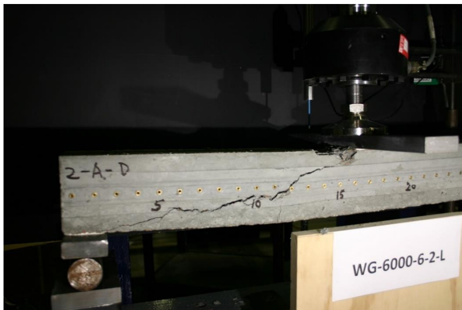
Figure 312 Picture of Failed Prism WG-6000-6-2-L
