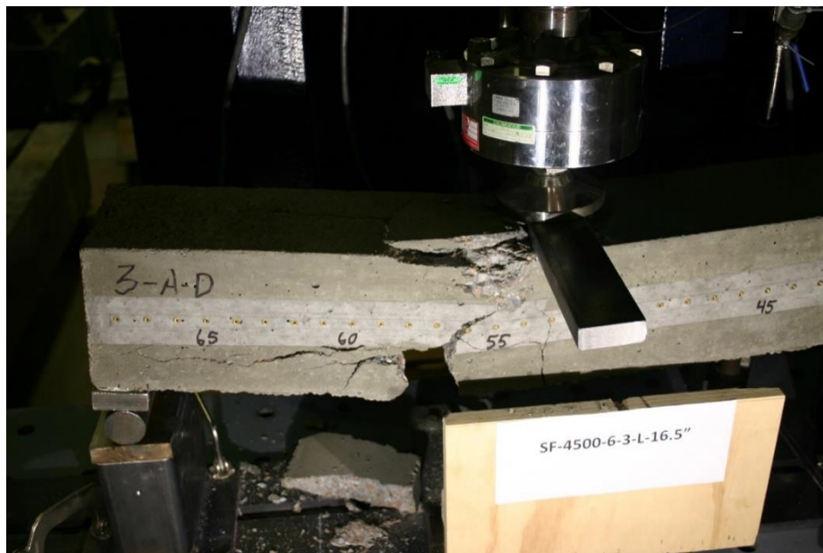
Figure 415 Picture of Failed Prism for SF-4500-6-3-L
