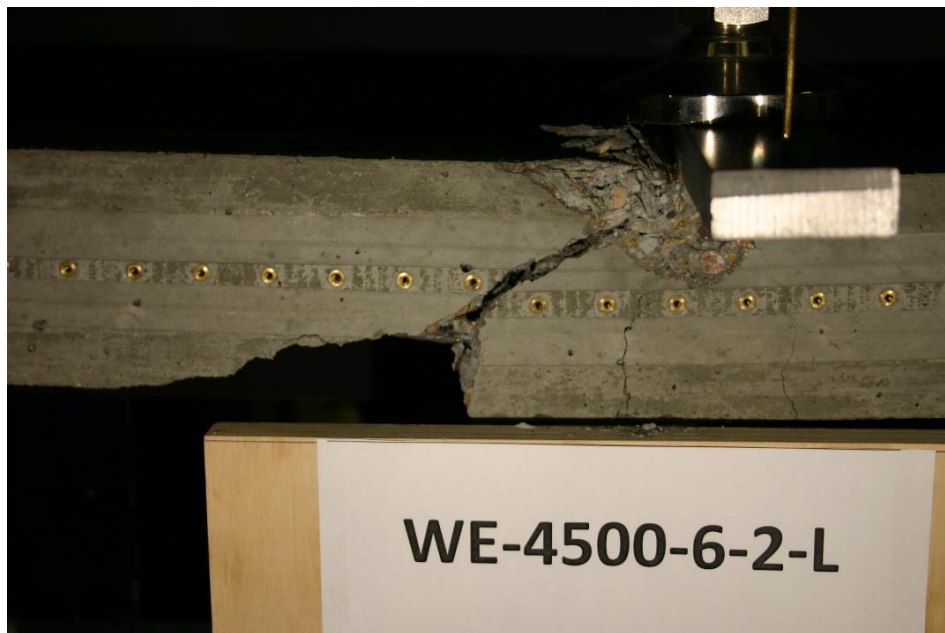
Figure 149 Picture of Failed Prism WE-4500-6-2-L
