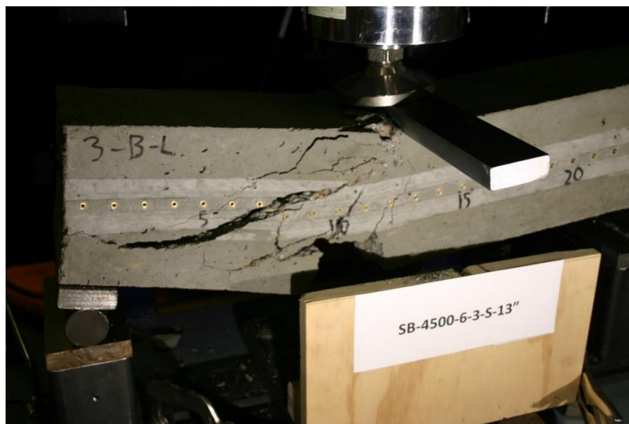
Figure 388 Picture of Failed Prism for SB-4500-6-3-S
