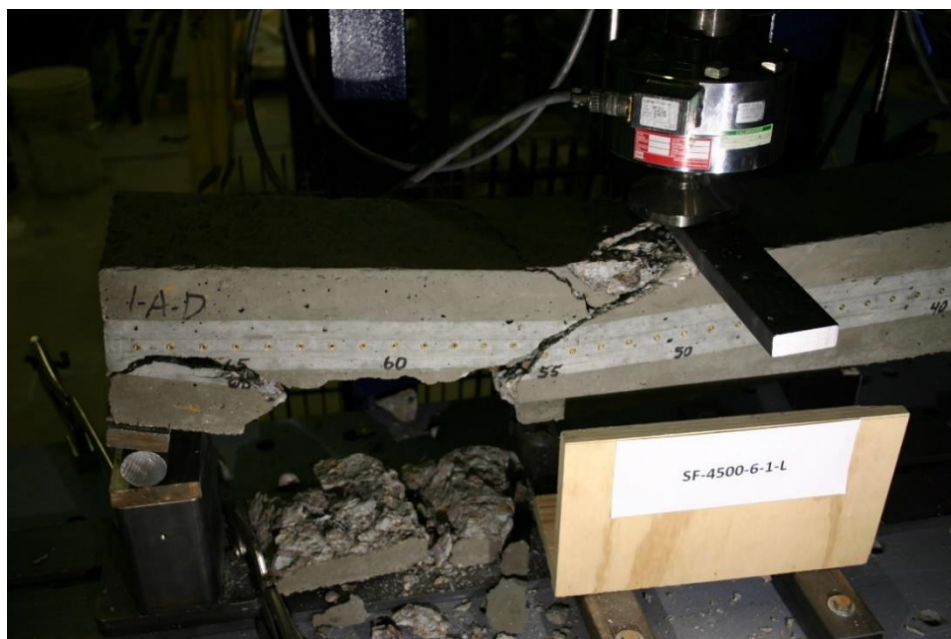
Figure 409 Picture of Failed Prism for SF-4500-6-1-L
