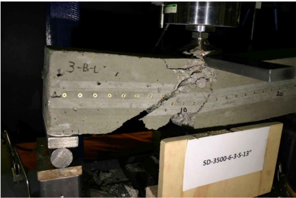
Figure 436 Picture of Failed Prism for SD-3500-6-3-S
