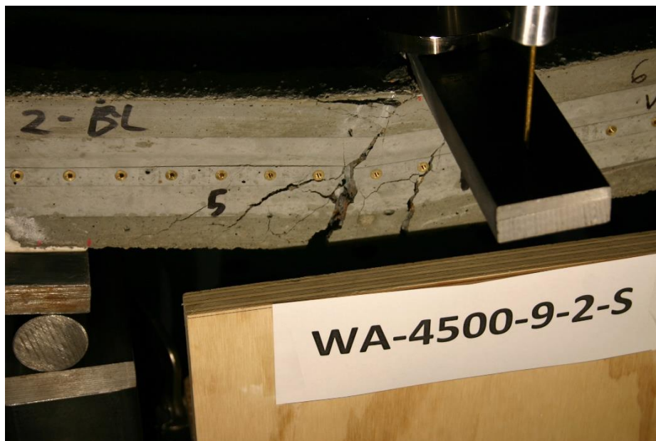
Figure 259 Picture of Failed Prism WA-4500-9-2-S
