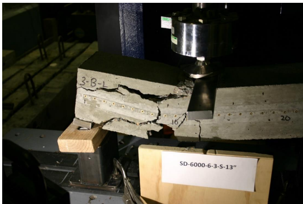
Figure 474 Picture of Failed Prism for SD-6000-6-3-S
