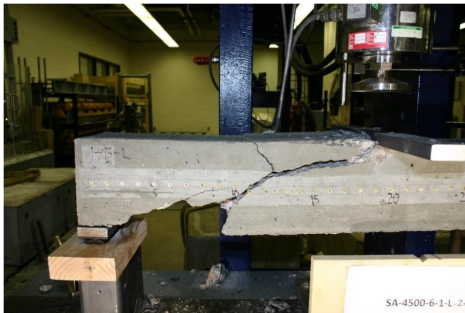
Figure 372 Picture of Failed Prism for SA-4500-6-1-L-2 nd
