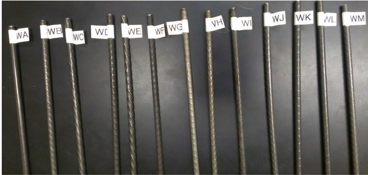
Figure 4. Picture of all 13 types of wire used in production of test prisms [after: (Arnold, 2013)]
