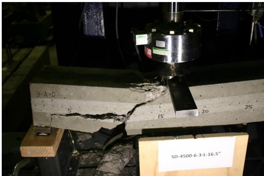
Figure 396 Picture of Failed Prism for SD-4500-6-3-L
