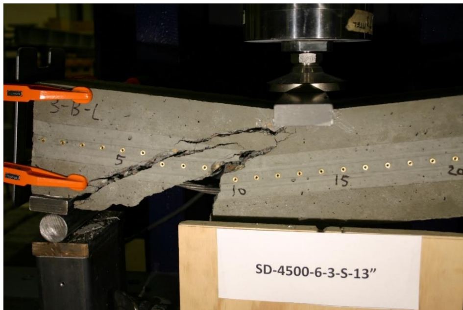
Figure 398 Picture of Failed Prism for SD-4500-6-3-S
