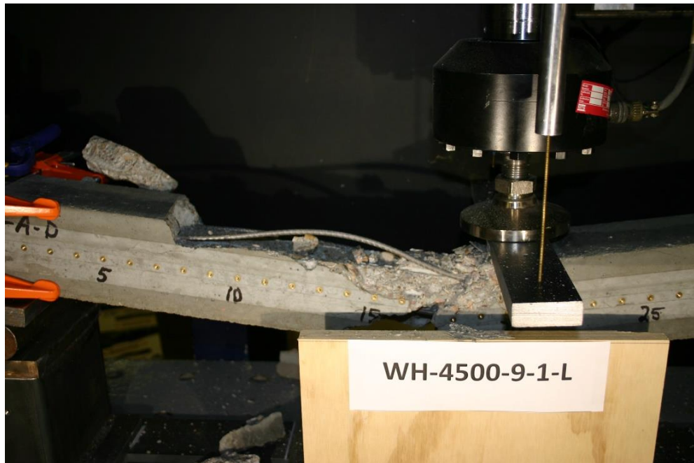
Figure 277 Picture of Failed Prism WH-4500-9-1-L
