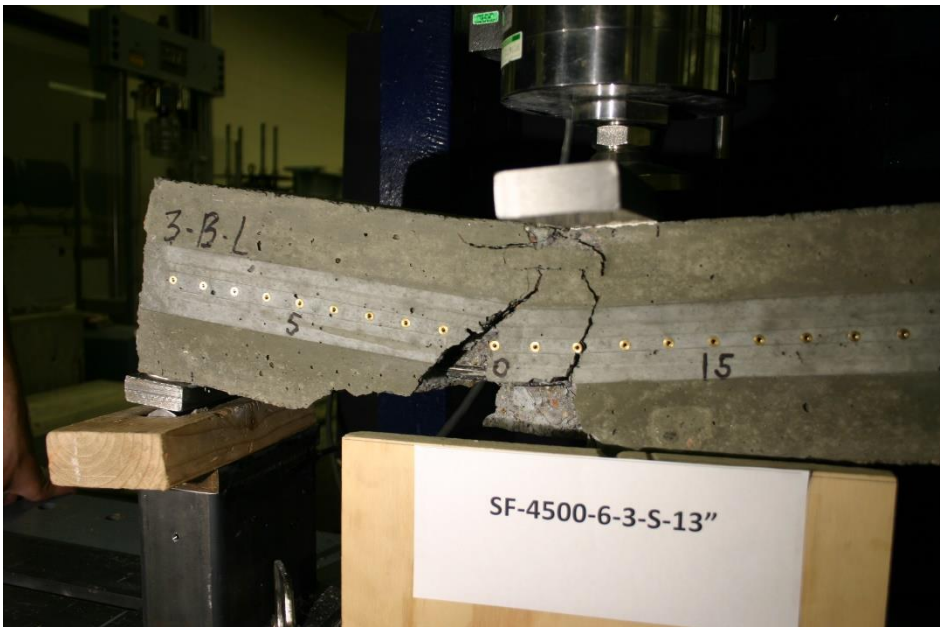
Figure 417 Picture of Failed Prism for SF-4500-6-3-S
