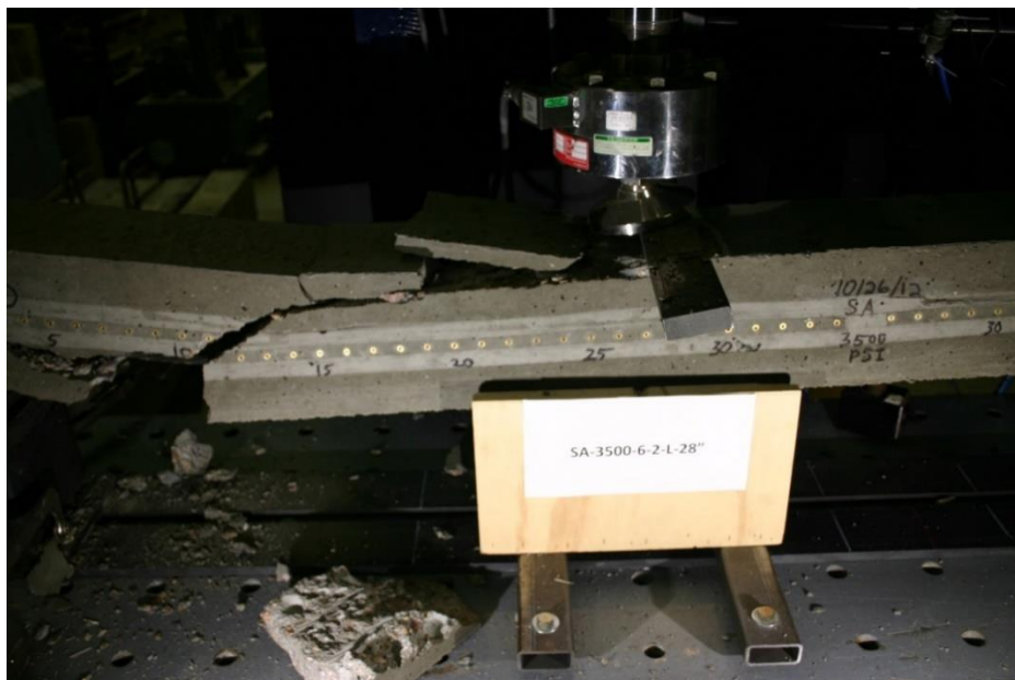
Figure 422 Picture of Failed Prism for SA-3500-6-2-L
