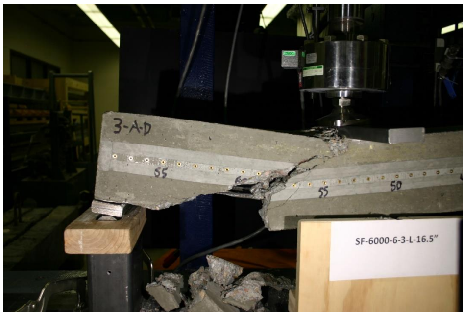
Figure 491 Picture of Failed Prism for SF-6000-6-3-L
