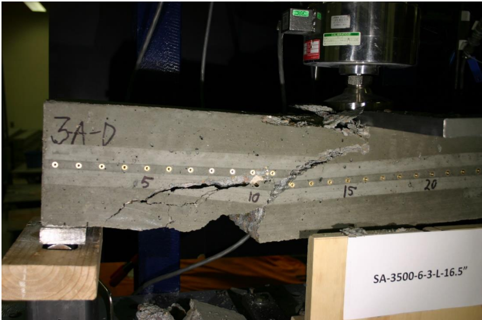
Figure 424 Picture of Failed Prism for SA-3500-6-3-L
