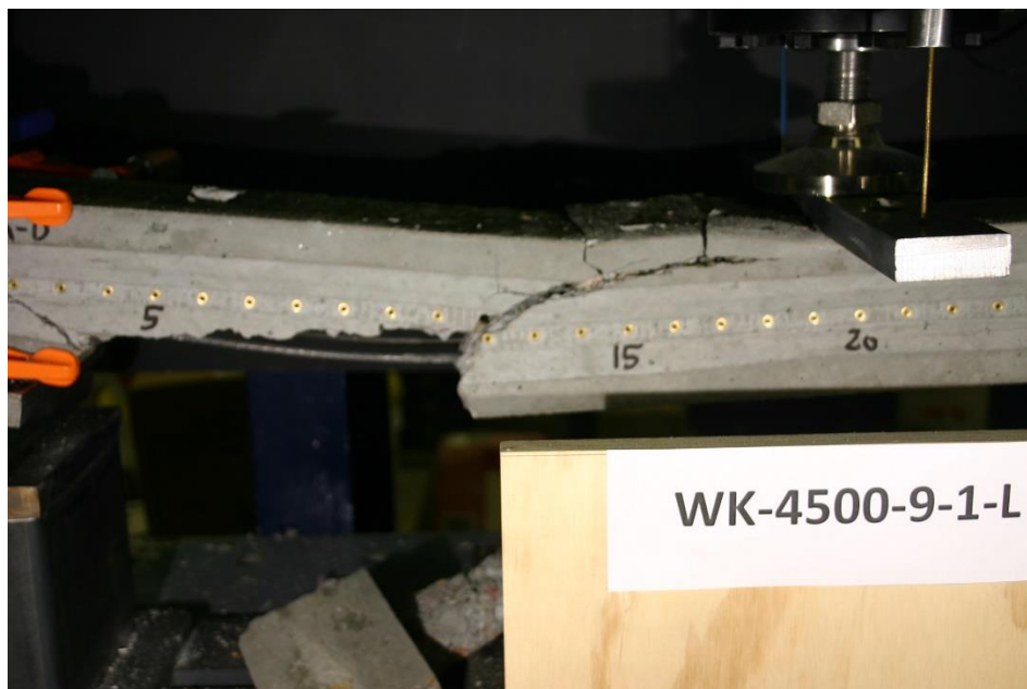
Figure 285 Picture of Failed Prism WK-4500-9-1-L
