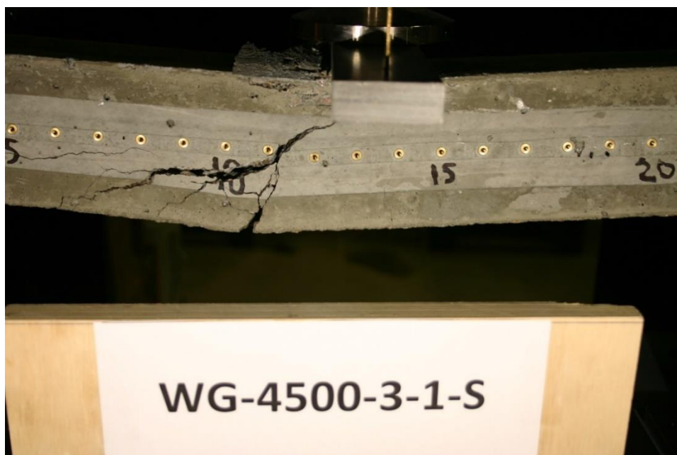
Figure 234 Picture of Failed Prism WG-4500-3-1-S
