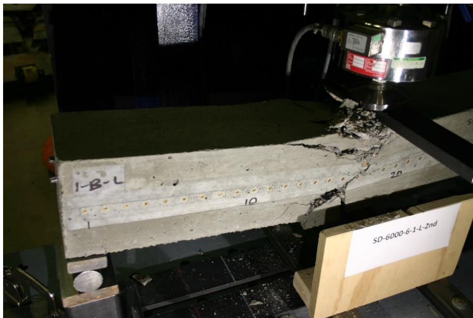
Figure 468 Picture of Failed Prism for SD-6000-6-1-L-2nd
