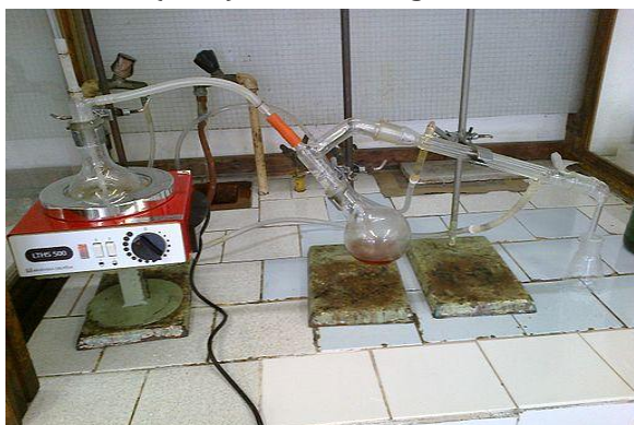
Fig 3:-Process of extraction of essential oil through Water and steam distillation technique
