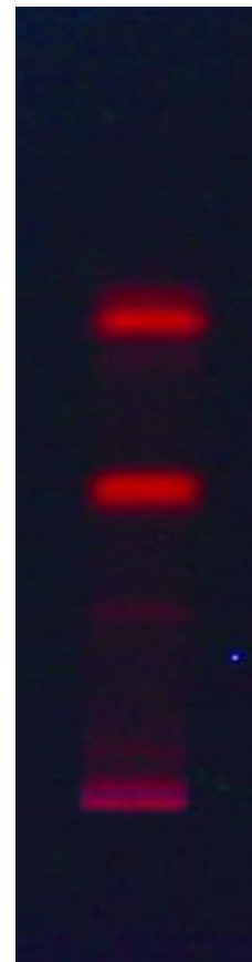
Fig 8: HPTLC Plate with solvent system Toluene: Ethyl acetate: Formic acid (9:1: 0.1)
