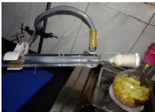
Condensation of Arka vapours
