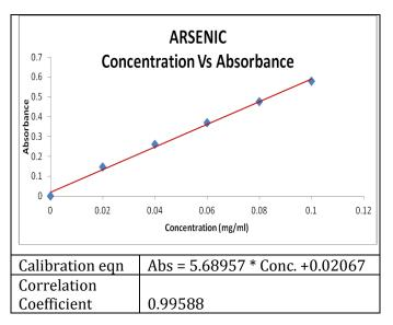
Arsenic was analysed at a maximum wavelength of 300 nm and at different conc. (0, 0.02, 0.04, 0.06, 0.08 and 0.1) and the corresponding absorbance was obtained. A graph is plotted between concentration and absorbance is called Calibration Curve. Based on this graph, the concentration of Arsenic in various samples was identified.
