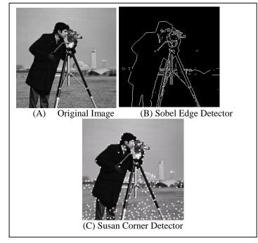
Figure 2: Edge and Corner Detection for Camera-Man image
