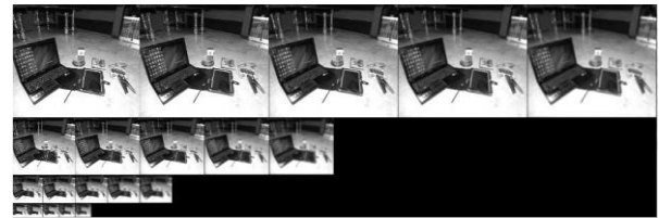
Figure (8). Pyramid scaling of the original image scaled into 4 octaves of G filter, scaled into five intervals of dimension in every octave.
