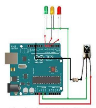
Figure 2: The Second Circuit Design Using (IR).
