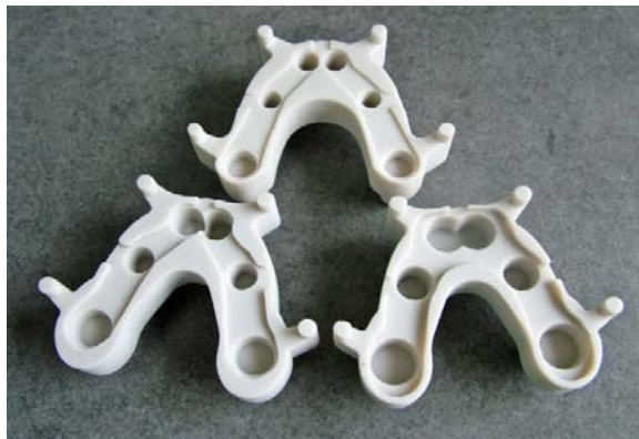
Fig. 2 – Custom trays with 1, 2 and 3 mm spacing made by rapid prototyping.
