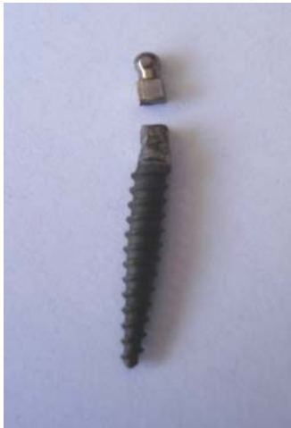
Figure 3. MDI broken during installation
