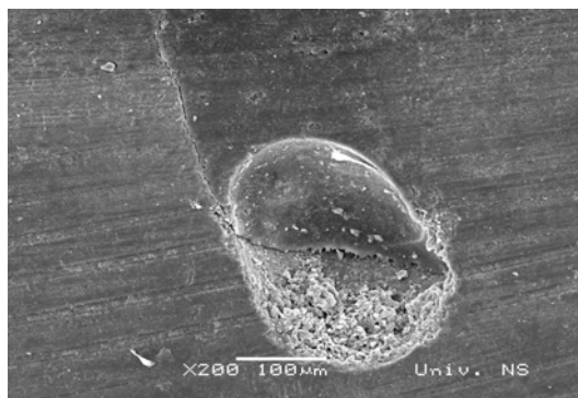
Figure 3. Air-bubble beneath glass-ionomer fissure sealant (200×).
