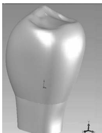
Figure 3. Final 3D model of an intact tooth with defined boundary conditions
