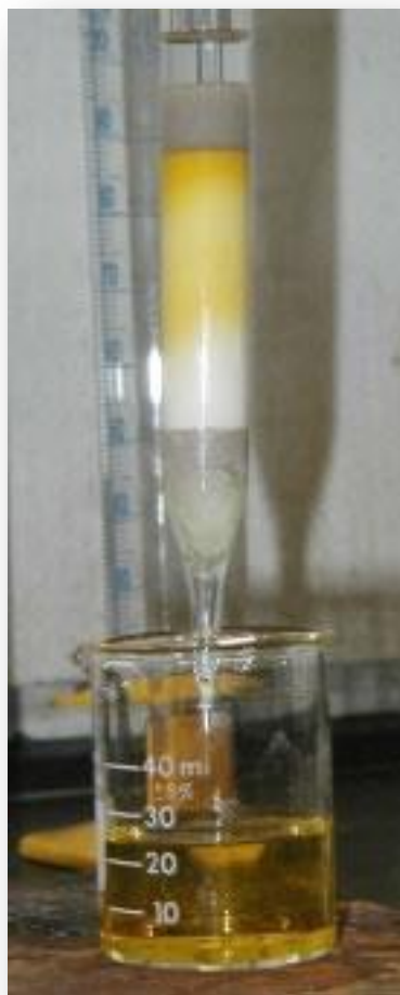
Fig. 2: Bands separation in Silica gel G column chromatography
