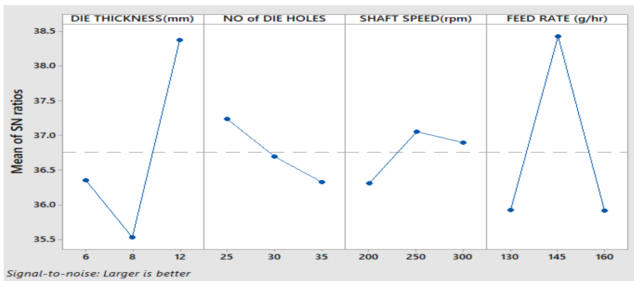
Fig. 2 Effects of S/N ratio for pelletizing efficiency versus die thickness (mm), number of die holes, shaft speed (rpm) and feed rate (g/h)
