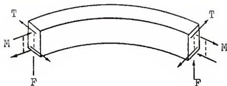
Fig. 2. A sign convention that can be applied to the end of any span
