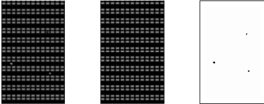
Fig. 5a Image from a chip with different repeating patterns in rows and columns
