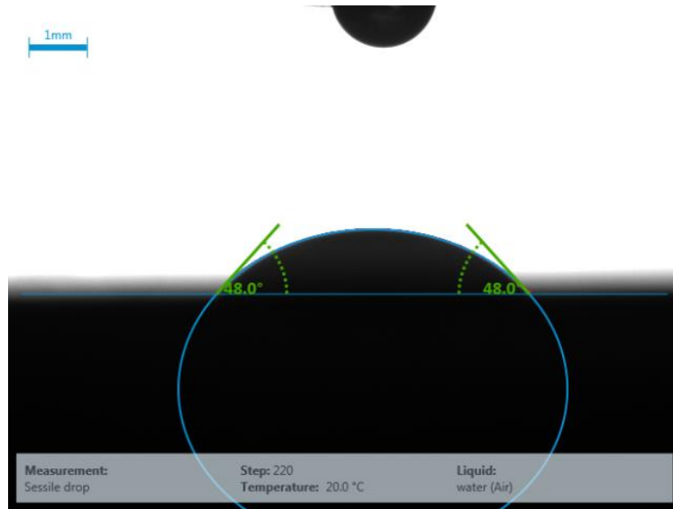
Figure 15 Contact angle of the Nylon filter membrane
