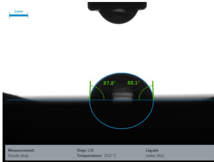
Figure 15 Contact angle of the Nylon filter membrane
