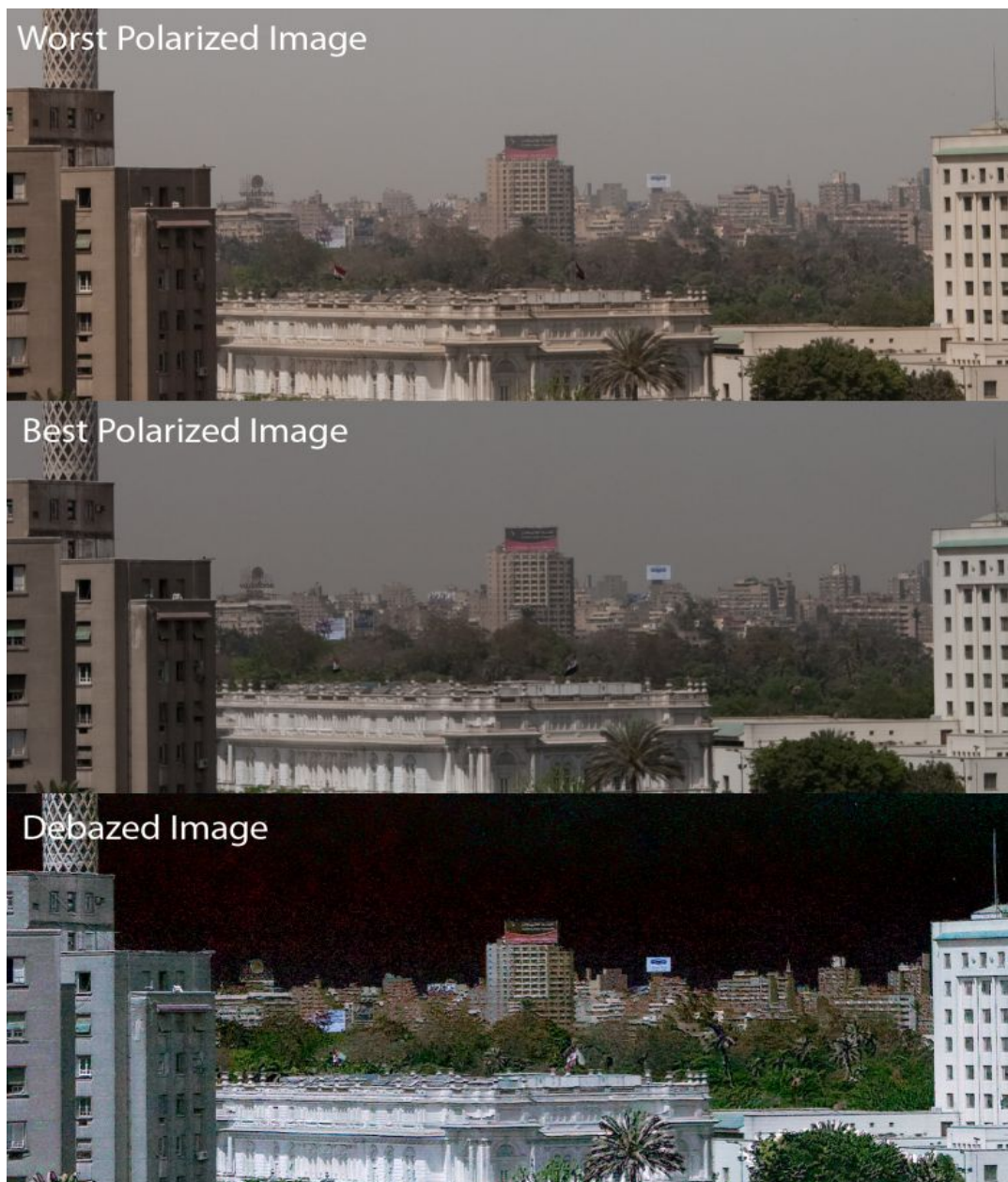
Figure 16: The worst polarized image, best polarized image and the dehazed image produced by the polarization-based dehazing algorithm.
