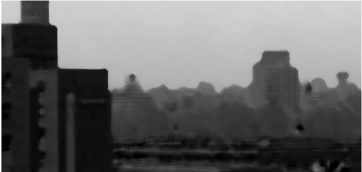
Figure 20: A cropped and enlarged region of the depth map produced by the algorithm. This figure shows the increase in brightness with depth.
