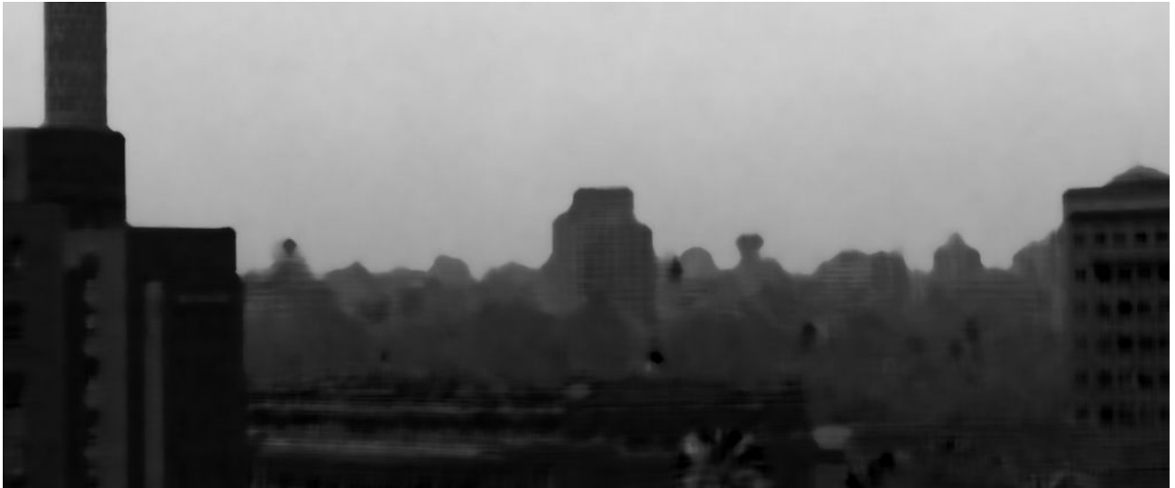
Figure 18: The range map byproduct of the dehazing process shows the relative depth of objects in the scene in the form of a grayscale image (lighter shaded objects have more depth). This image shows the same scene as in figure 16.
