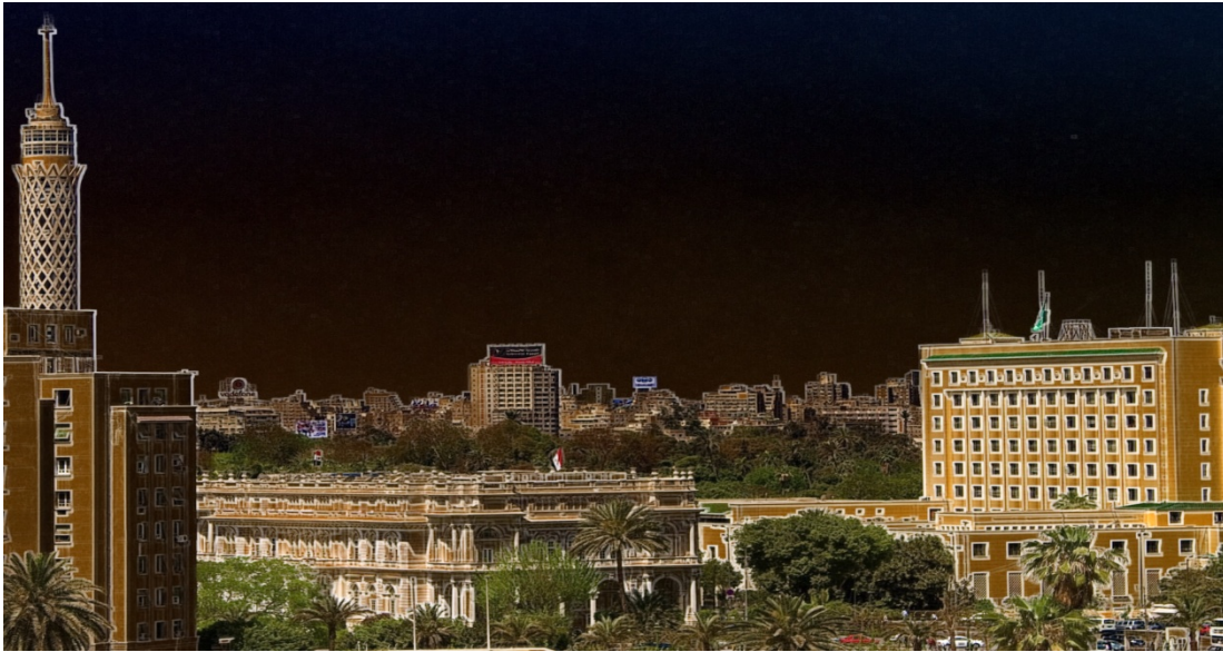
Figure 24: A dehazed image of a scene using the dark channel dehazing algorithm. Some of the colors are distorted due to their colors being close to the colors of airlight.
