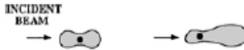
Figure 8: Shows Rayleigh scattering (left) which scatters the same intensity symmetrically backwards and forwards. Mie scattering is predominantly in the forward direction as seen on the right [31].
