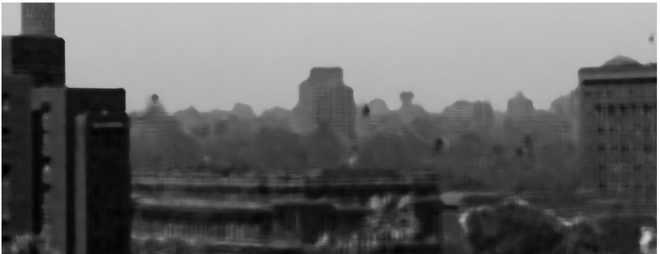
Figure 19: Similar to the previous figure, the haze extracted from the scene can be displayed as a grayscale map.
