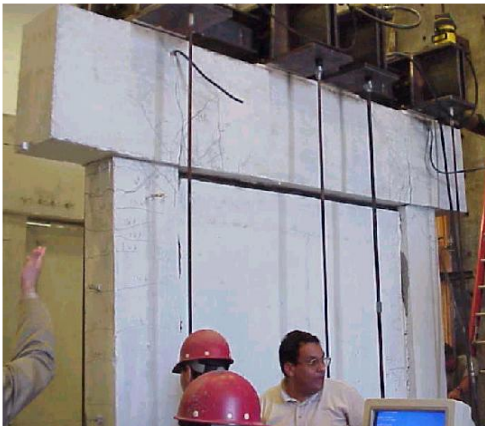
Figure 1.6 A column bent with an infill wall where a gap was left between the wall and the bent cap for field construction purposes. [3]
