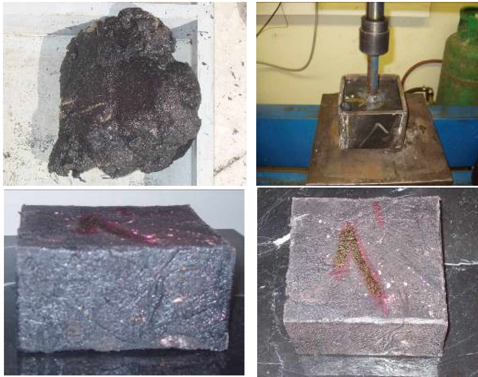
Figure 26: Mix Paste (Up Left); Press (Up Right); Produced Sample (Down)
