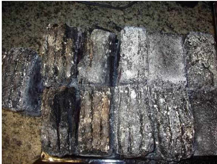
Figure 54: Melted Samples with Salt Precipitation
