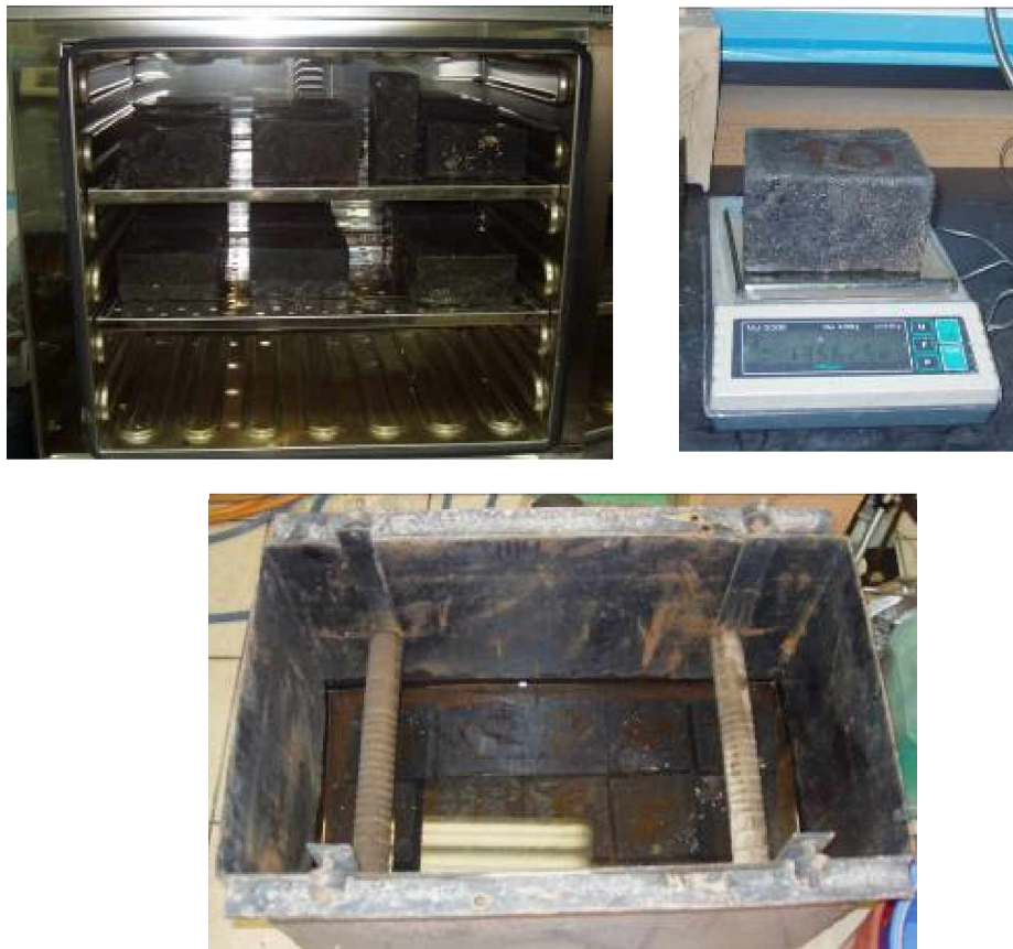
Figure 33: Conditioning ( Up Left ), Weighing ( Up Right ) and Immersion ( Center )
