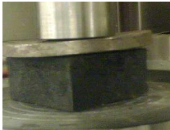
Figure 53: Deformation of Loading Plate on 810 MTS Machine
