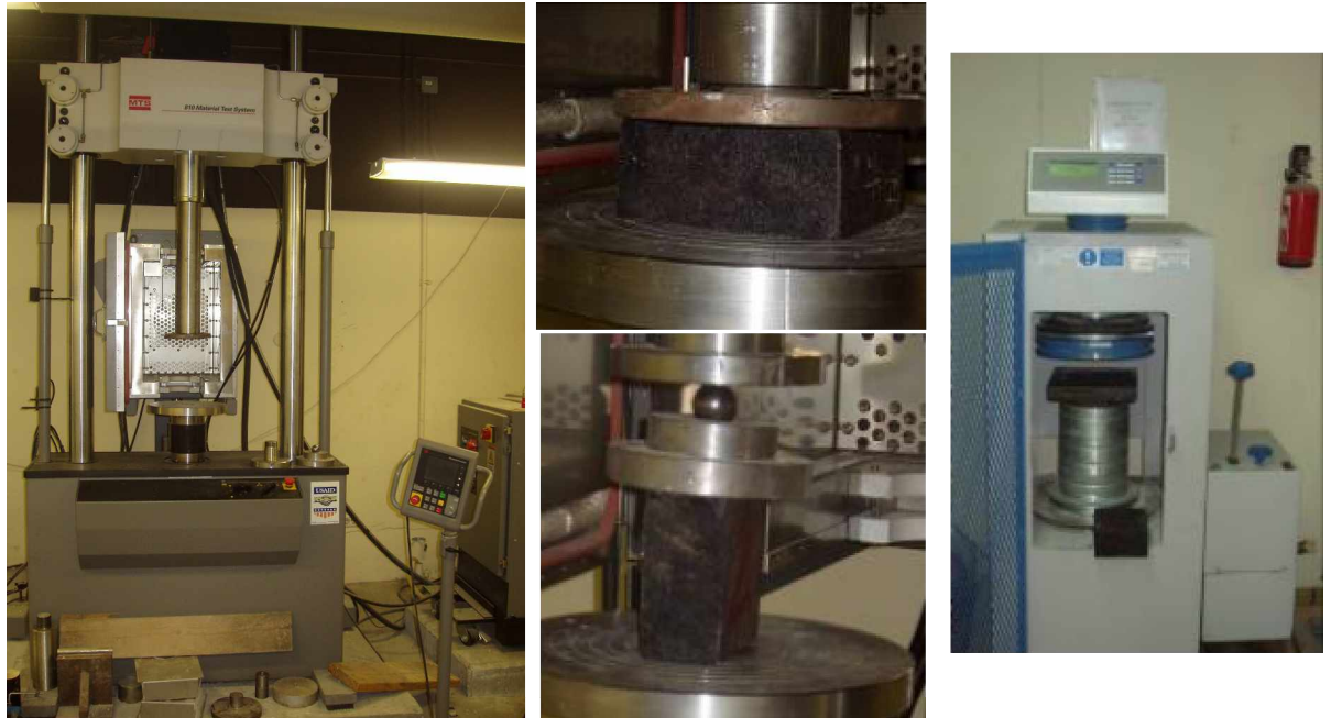
Figure 35: MTS Machine (Left), Parallel Loading (Center Up), Perpendicular Loading (Center Down), Fracture Machine (Right)
