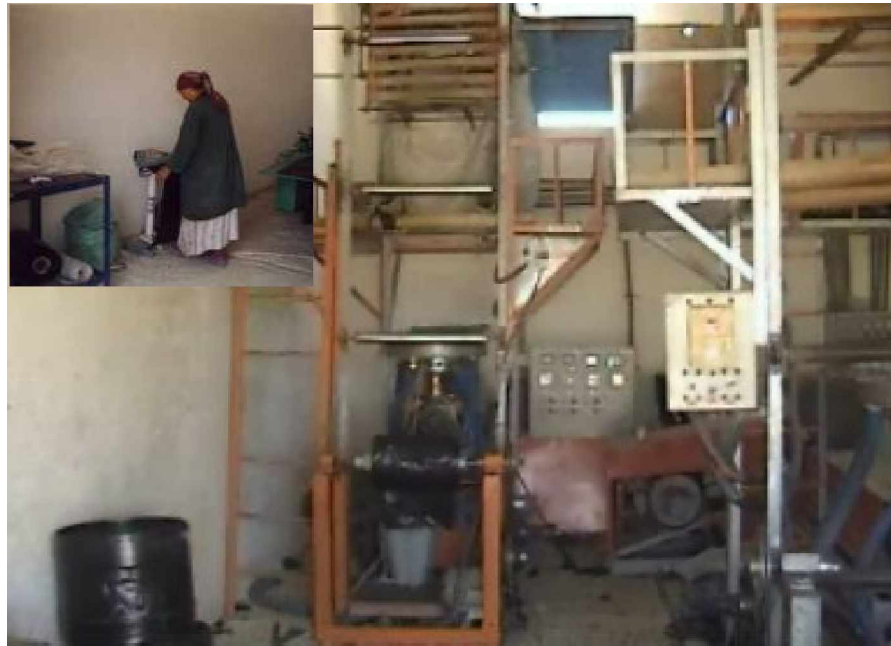
Figure 15: Film machine that converts LDPE into garbage plastic bags
