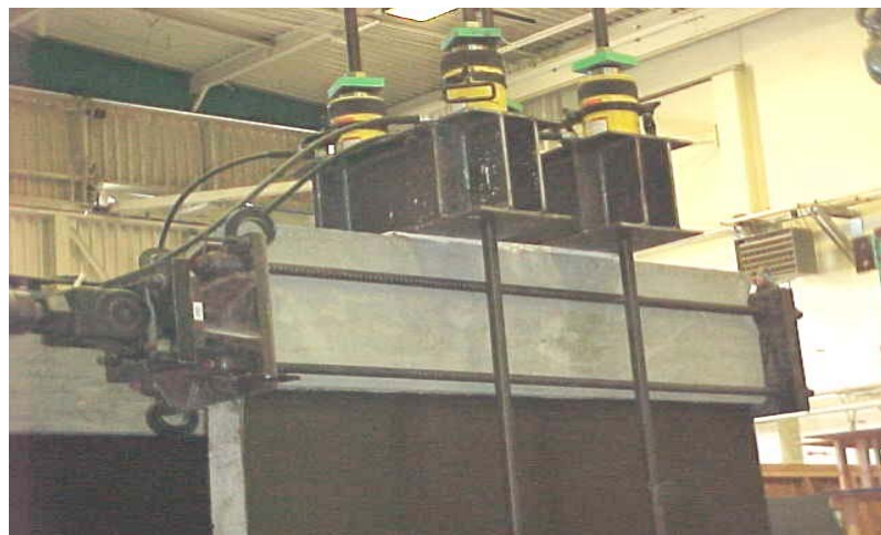
Figure (2.11) Gravity and cyclic shear loading on typical wall
