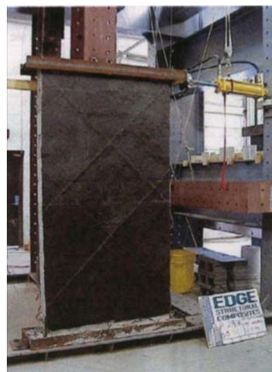
Figure (2.5) Retrofitted shear specimen at failure
