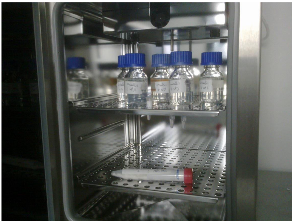
Figure 48: solutions of worm-like micelles with different concentrations prepared for this experiment and kept at constant temperature below their Kraft point
