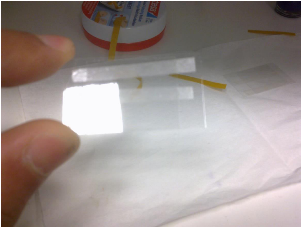
Figure 49: sample chamber before pipetting in the solution to be studied, double sticky tape is used to hold both glasses together, sealing (with nail polish) goes at the sides
