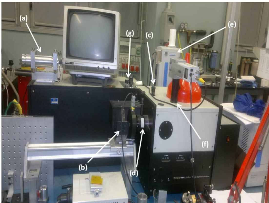
Figure 4.15. (a) is the infinite adjusted telescope used to adjust the position of the sample, (b) the second lens L2 that focus the image on the entrance slit of the spectrometer, (c) the second slit inside the spectrometer, (d) the first entrance slit, (e) Symphony CCD, (f) the periscope mounted inside the spectrometer and its image is shown on the monitor. (g) the diffraction grating resolution of the image (1800 gr/mm).
