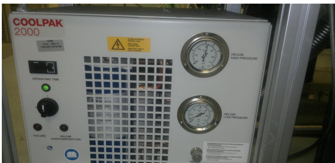
Figure 4.6. The cryogenic device, capable of cooling the system down to 10 K.
