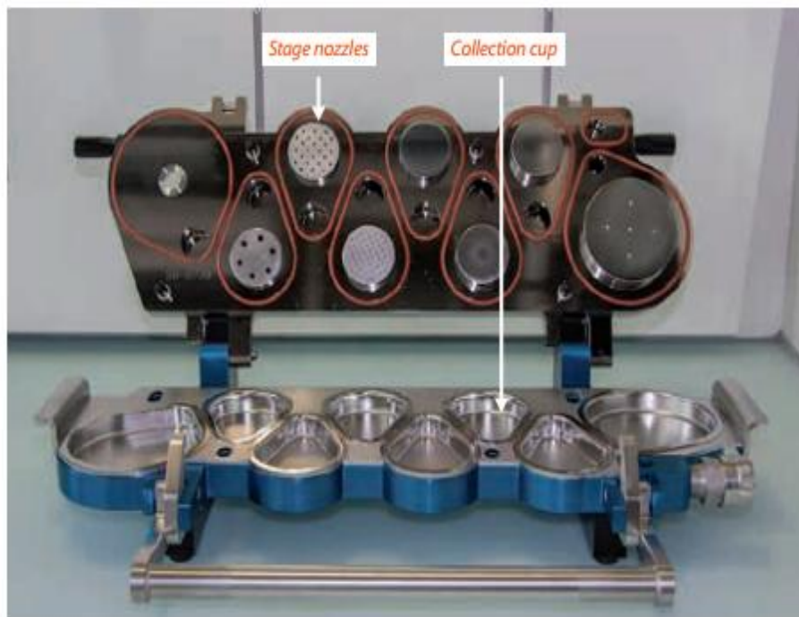
Figure 12: NGI Assembly (Induction port, Preseparator, Stages 1-7 and MOC) – Dry Powder will be moving from DPI placed at the mouth adaptor along the whole apparatus from the left to the right when vacuum is turned on. Particles will then deposit in different compartments of the NGI based on the AD cutoffs- Retrieved from www.solvias.com/sites/default/files/solvias_prospects_02_2012_web.pdf , December, 2014.
