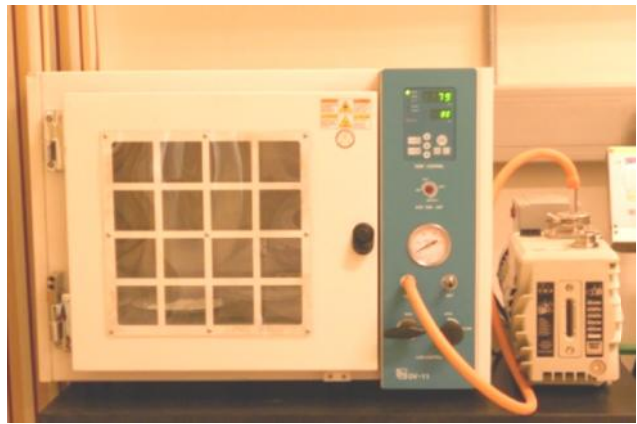
Figure 4.10: Vacuum Oven (OV-11) used for degassing
