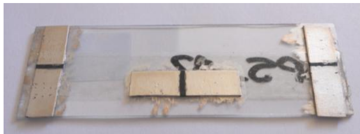
Figure 4.15: Specimens produced by flash type mold adhered to glass slide
