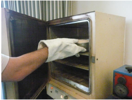
Figure 4-2: Putting the wood waste to be dried
