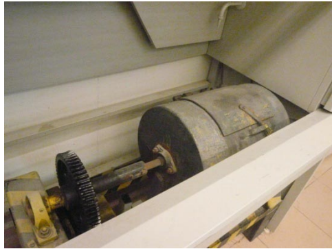
Figure 4-9: The furnace used for heating the shredded particles to form a paste
