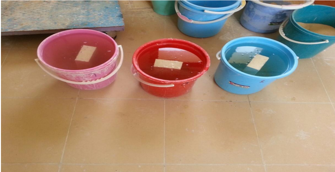
Figure 3.21: Water Absorption Test
