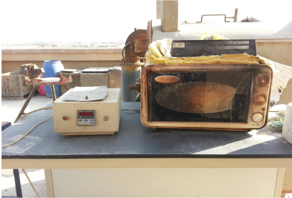
Figure 3.8: Heating Oven and its Temperature Control Unit
