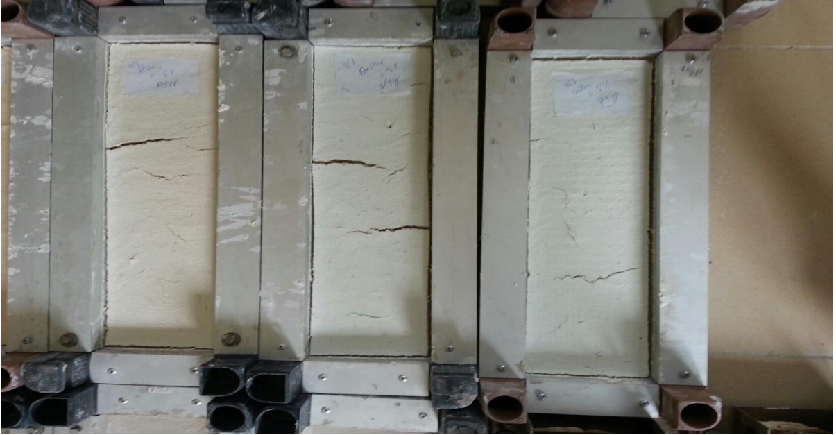
Figure 4.9: Cracks in Unheated Gypsum Samples
