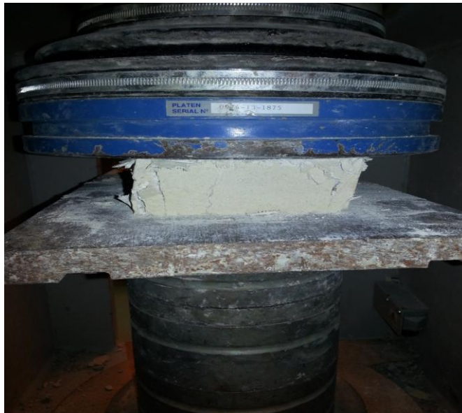
Figure 3.19: Specimen after Failure of Compressive Strength Test
