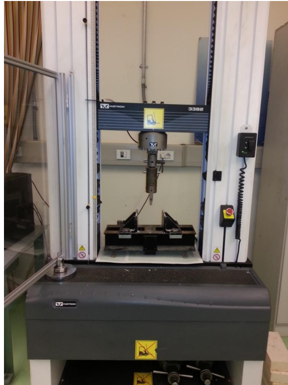
Figure 3.16: Bluehill Instron Machine – 3382 Used for Flexural Strength Test
