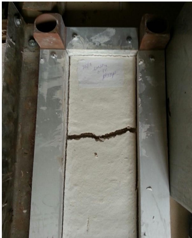
Figure 4.10: Cracks in Unheated Gypsum Samples
