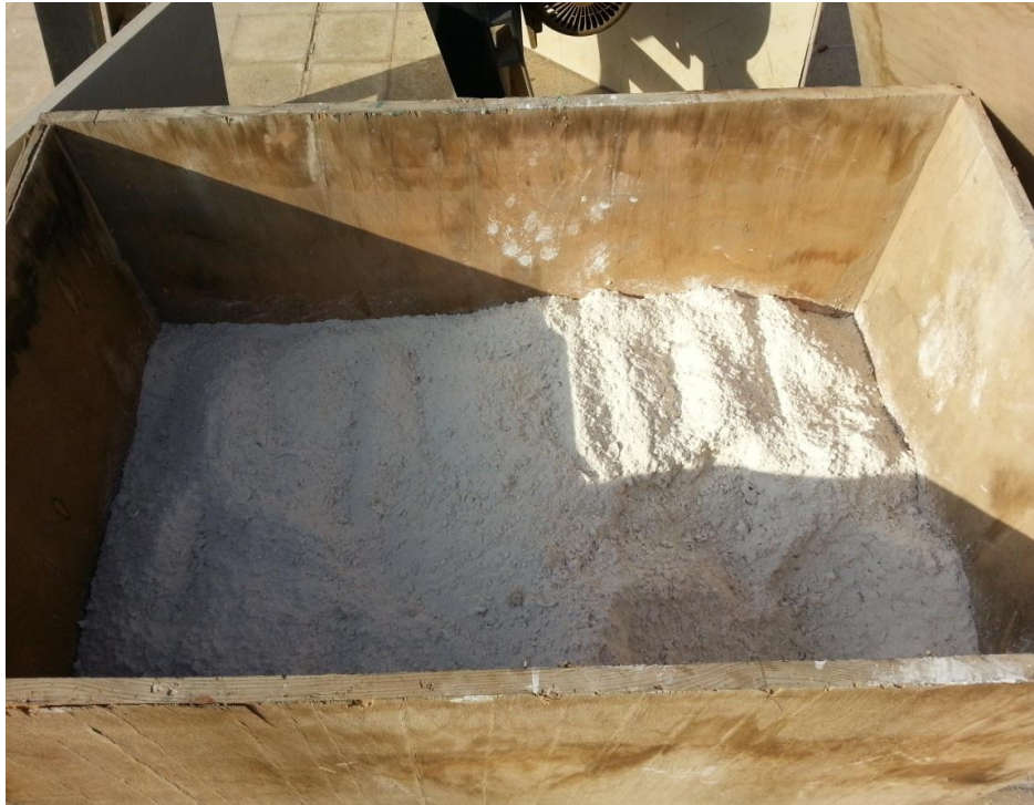
Figure 3.10: Unheated Gypsum Board Waste after the Grinding Process
