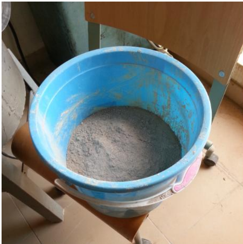
Figure 3.9: Waste Gypsum Board after the Heating Process
