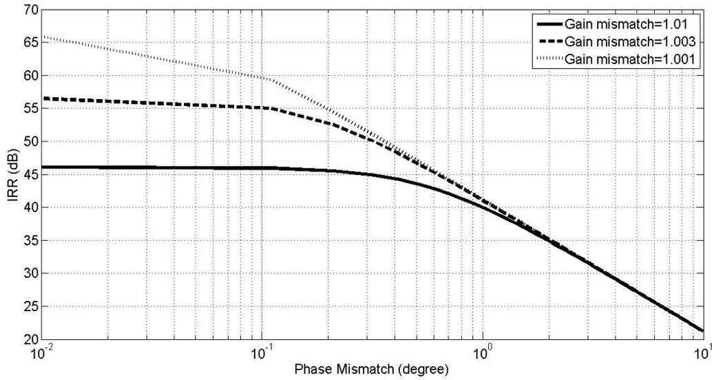
**Fig. 2: IRR across Phase Mismatch ( $\phi$ ) at different gain mismatches ( $g$ )**
