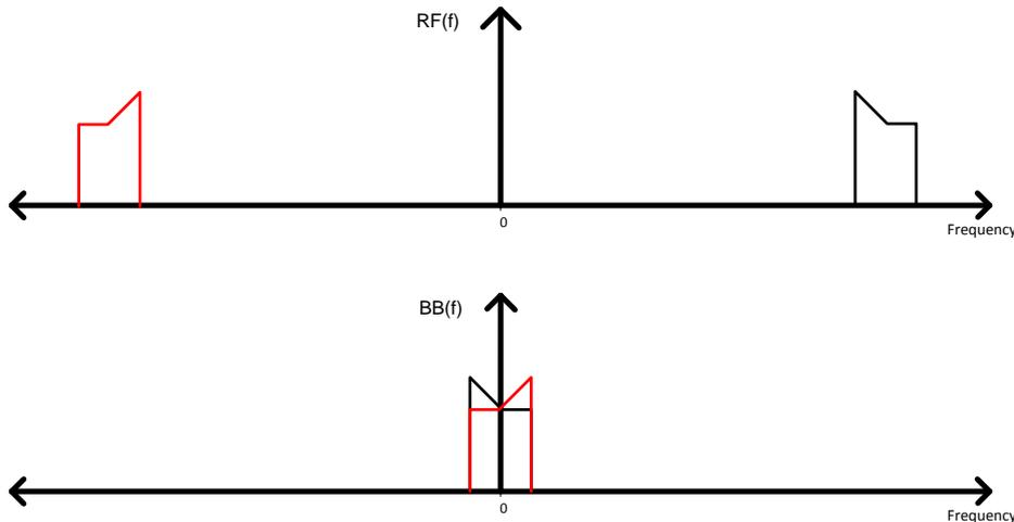
Fig. 6: Self Imaging In Direct Conversion Receiver
