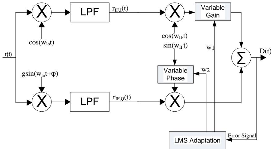
**Fig. 31: Image reject receiver with IQI Calibration loops using LMS adaptation and an external test tone at the image frequency**
