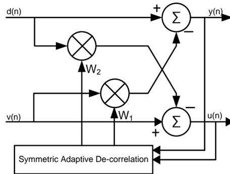
Fig. 41: Symmetric Adaptive De-correlation (SAD) Block Diagram[24]
