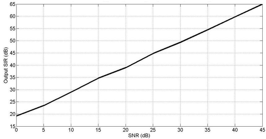
**Fig. 85: Output SIR across SNR ,  $g=1.02$ ,  $\phi=2$  degree’s, input SIR=-20dB and  $N=100$**
