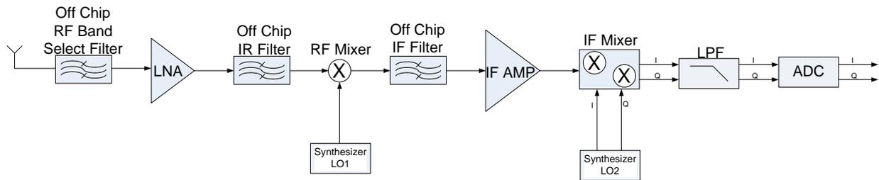
**Fig. 4: Superheterodyne Receiver Architecture**
