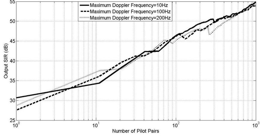
**Fig. 80: Output SIR across number of Pilots “N” , g=1.02, phi=2 degree’s, input SIR=-20dB, SNR=35dB with Rayleigh Fading**
