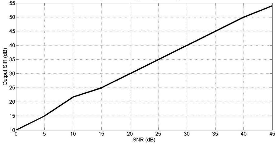
**Fig. 81: Output SIR across SNR , g=1.02, phi=2 degree’s, input SIR=-20dB and N=100**
