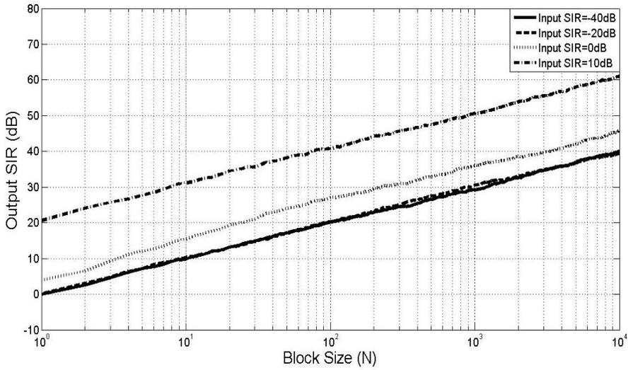
**Fig. 59: Dual-tap IQI compensation using method of moments, Output SIR across Time Iterations (N),  $g=1.02$ ,  $\phi=2^\circ$ , SNR=35dB**
