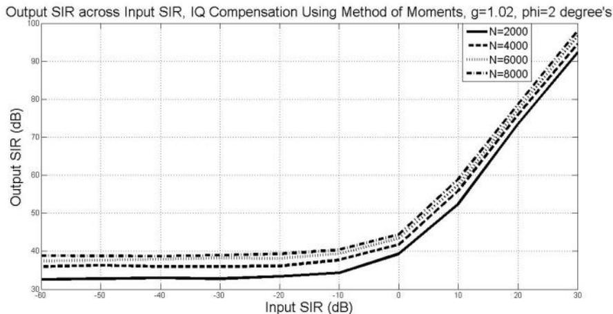
Fig. 57: 2-Tap Method Using Method of Moment, Output SIR across input SIR,  $g=1.02$ ,  $\phi=2^\circ$ ,  $SNR=35dB$
