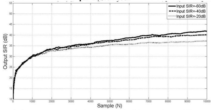
**Fig. 48: single-tap IQI compensation method using Method of Moment, Output SIR across Time,  $g=1.1$ ,  $\phi=10^0$ , SNR=35dB**
