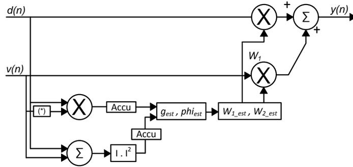
Fig. 42: IQI Compensation Using Signal & Image Separation using 2-Tap Filters
