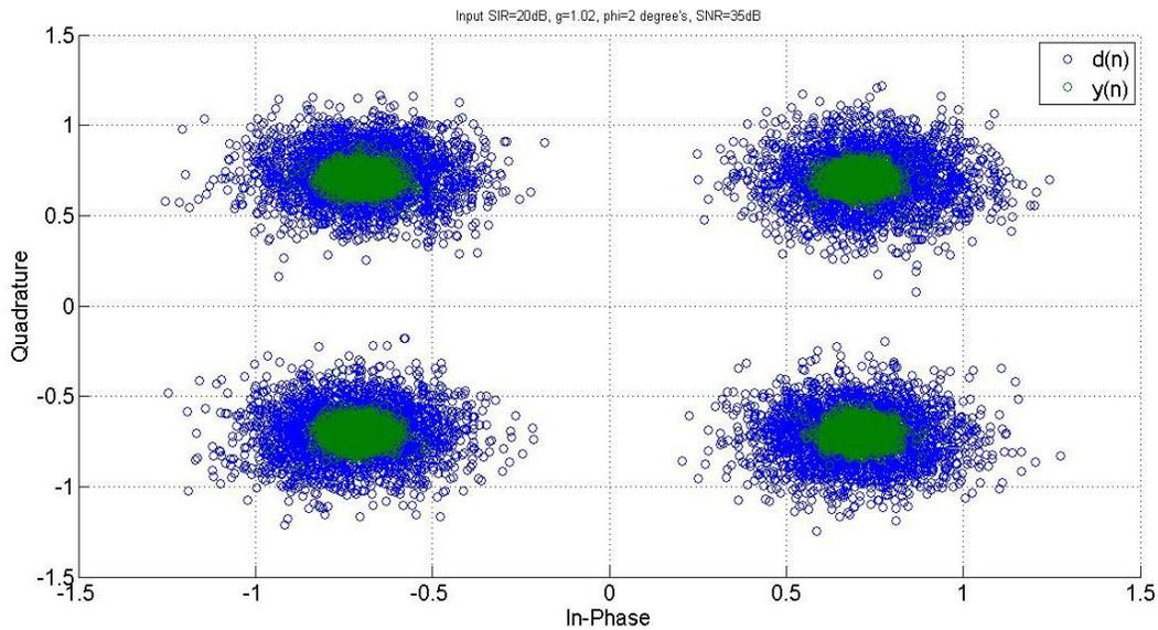
**Fig. 64: Signal constellation for the compensated signal  $y(n)$  and the uncompensated signal  $d(n)$ ,  $g=1.02$ ,  $\phi=2$  degree's, input SIR=-20dB**
