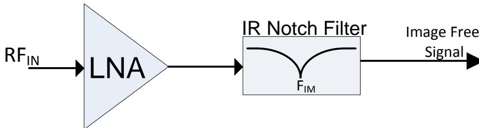
Fig. 13: Image Reject LNA using an image reject notch filter
