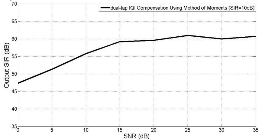
Fig. 62: Output SIR across SNR for the dual-tap IQI compensation using method of moments
