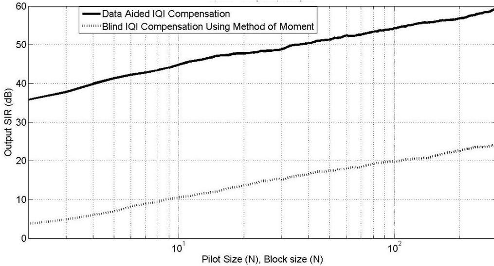
Fig. 77: Output SIR across the block size "N" for the blind IQI compensation using method of moments, and across the pilot size "N" for the data aided matrix-nulling method
