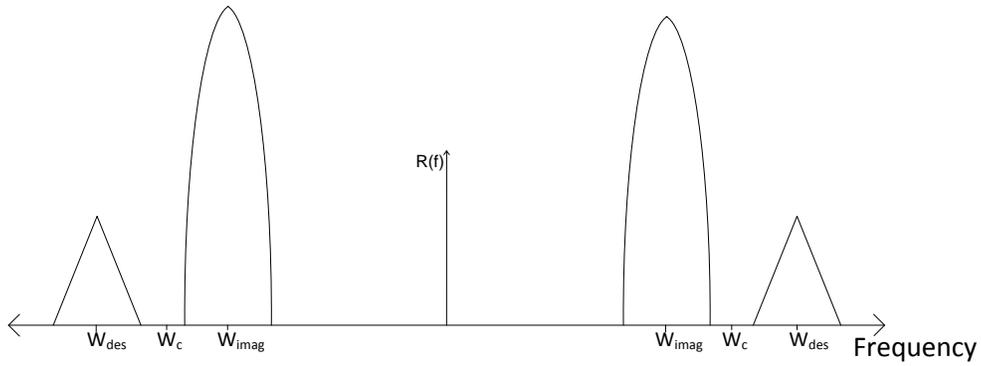
**Fig. 3: Multi channel frequency band**
