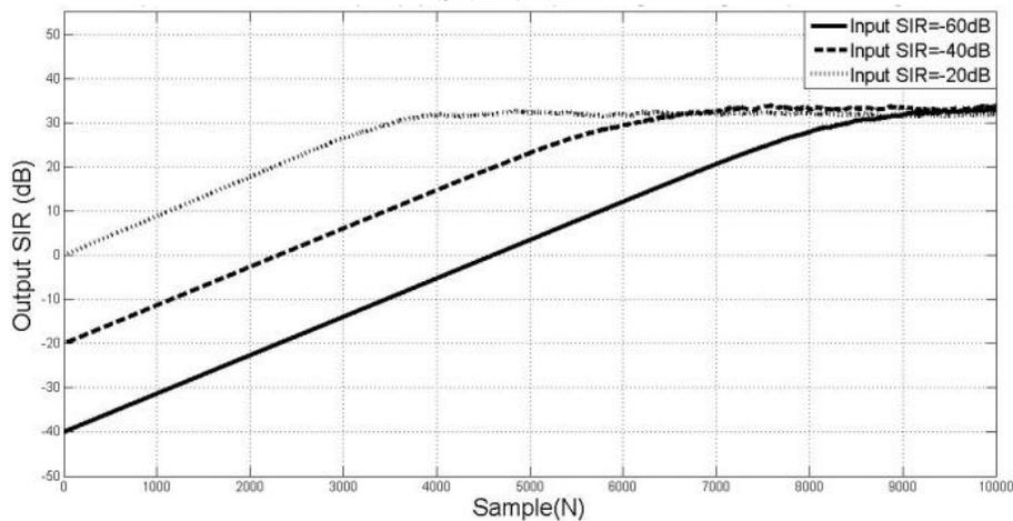
**Fig. 46: single-tap IQI compensation method using LMS, Output SIR across Time,  $g=1.1$ ,  $\phi=10^\circ$ , SNR=35dB**
