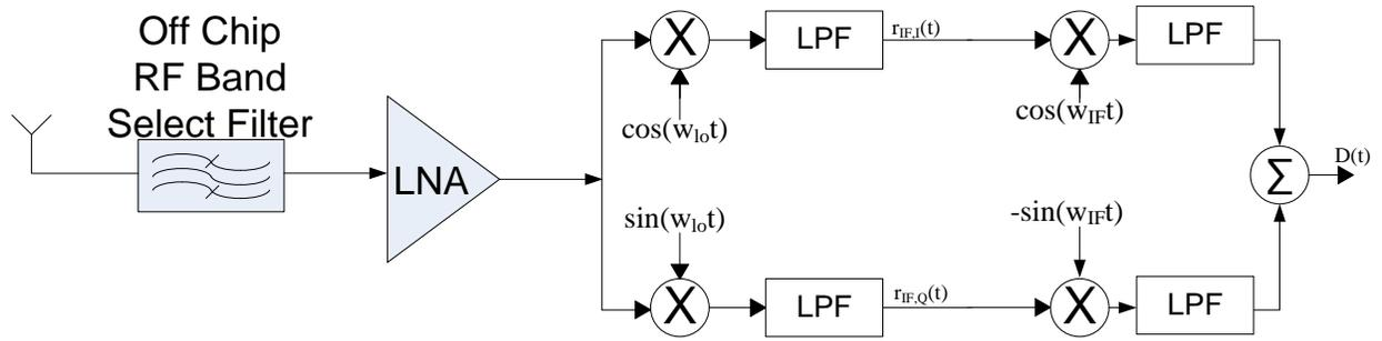
**Fig. 19: Weaver Receiver Architecture For Image Reject Mixers (For Low IF Receivers or Direct Conversion Receivers with Symmetric Channel Responses)**
