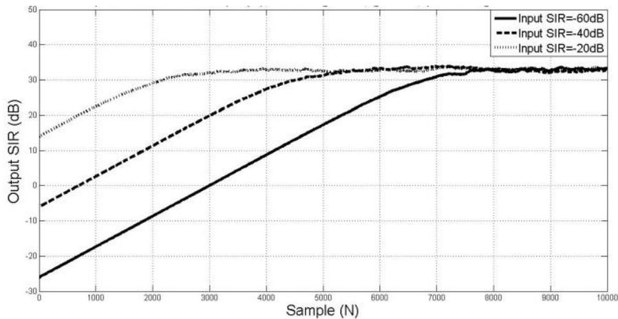
**Fig. 45: single-tap IQI compensation method using LMS, Output SIR across Time,  $g=1.02$ ,  $\phi=2^\circ$ , SNR=35dB**
