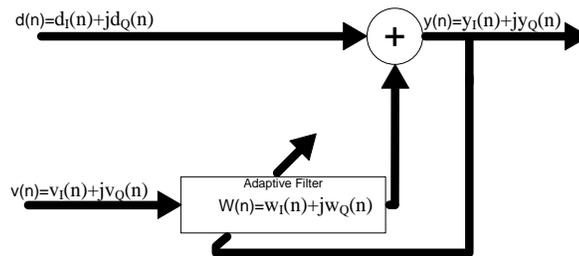
Fig. 40: Single-tap IQI Compensation using LMS Block Diagram
