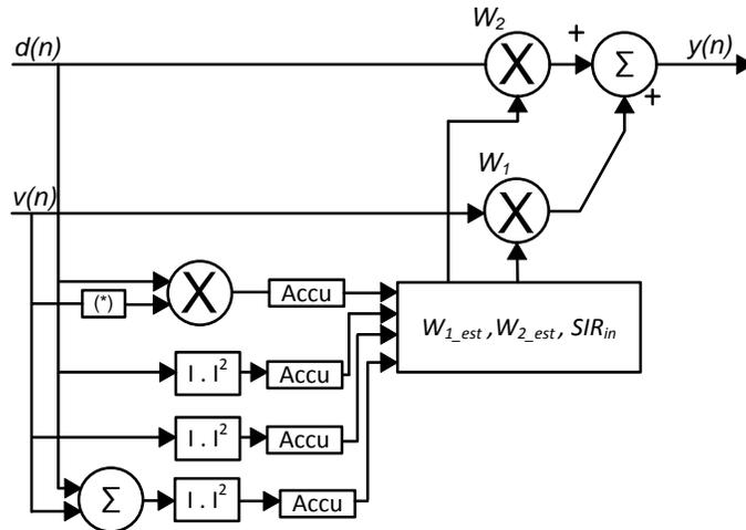
Fig. 56: Dual-Tap IQI Compensation using method of moments, second approach measuring four moments
