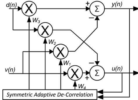
**Fig. 67: Proposed dual-tap IQI compensation with output signal rescaling**
