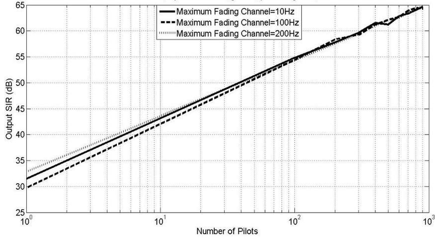
**Fig. 83: Output SIR across number of Pilots “N/L”,  $g=1.02$ ,  $\phi=2$  degree’s, input SIR=20dB, SNR=35dB with Rayleigh Fading,  $L=2$**
