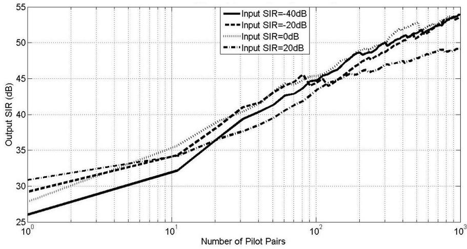
**Fig. 78: Output SIR across number of Pilots “N” ,  $g=1.02$ ,  $\phi=2$  degree’s, SNR=35dB with slow fading conditions**
