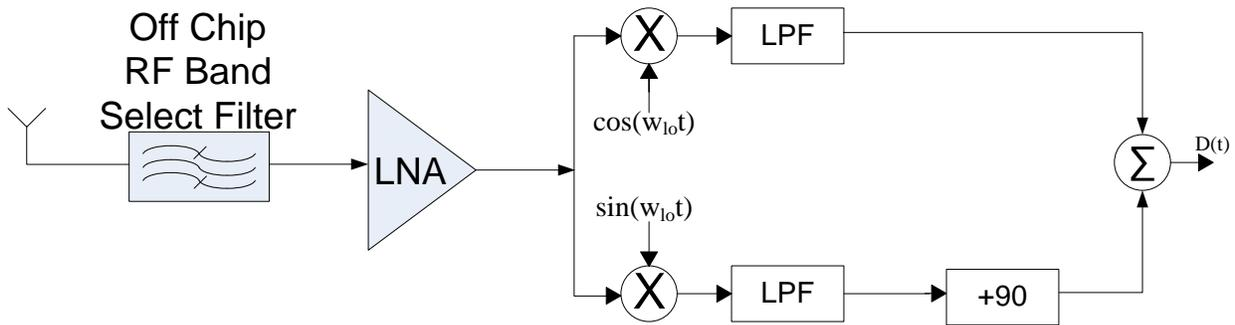
Fig. 15: Hartley Receiver Architecture
