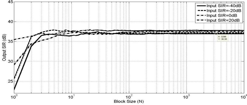
Fig. 72: Output SIR across the known sequence length "L", at SNR=35dB,  $g=1.02$ ,  $\phi=2$  degree's
