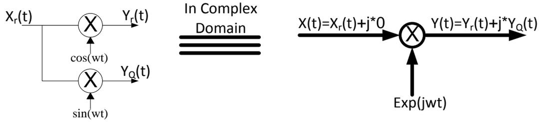
Fig. 8: Quadrature Mixing In Real & Complex Domain
