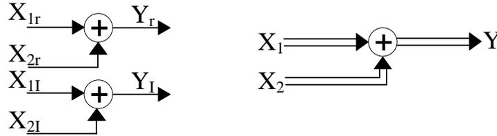
Fig. 10: Complex Signal Addition
