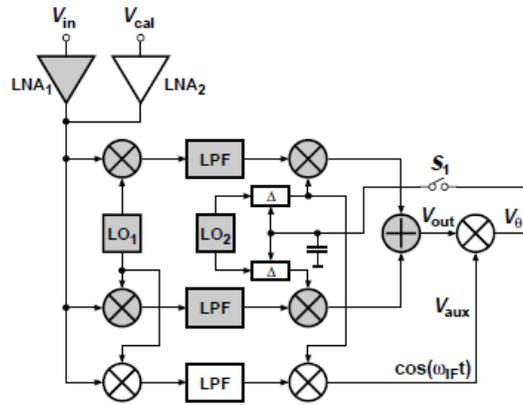
**Fig. 30: Image reject receiver with phase calibration loop using auxiliary path**
