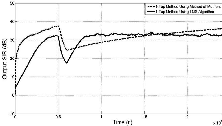
**Fig. 51: Output SIR across Time(n) at input SIR=-30dB and SNR=35dB, varying gain mismatch linearly from  $g=1.02$  to  $g=1.03$  and phase mismatch from  $g=2^0$  to  $g=2.5^0$  starting at  $n=5000$  till  $n=6000$ .**
