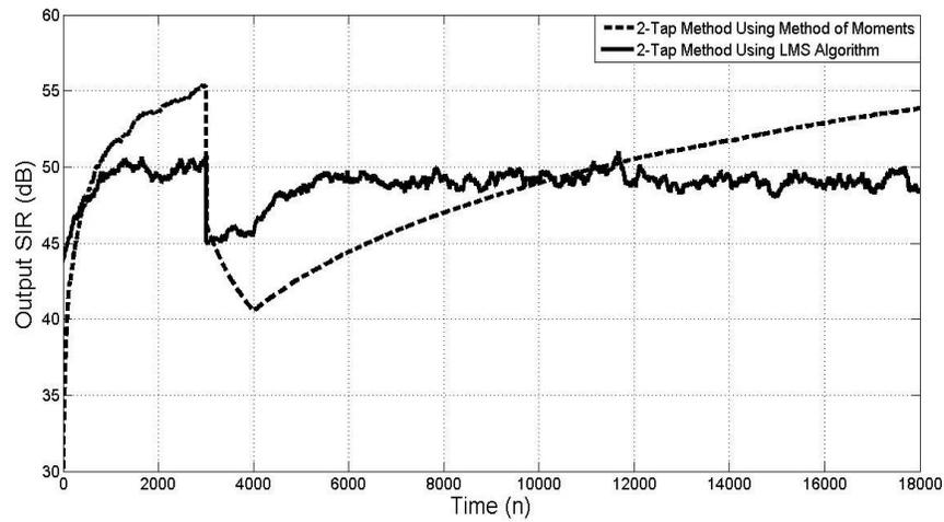
**Fig. 70: Output SIR across Time(n) at input SIR=10dB, varying the gain mismatch at  $n=3000$  from  $g=1.02$  to  $g=1.05$  then linearly from  $g=1.05$  to  $g=1.1$  till  $n=4000$ , and increasing phase mismatch linearly from  $g=2^0$  to  $3^0$  starting at  $n=3000$  till  $n=4000$ .**
