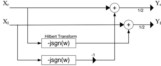
**Fig. 22: Real Signal Model For the Complex Filter**
