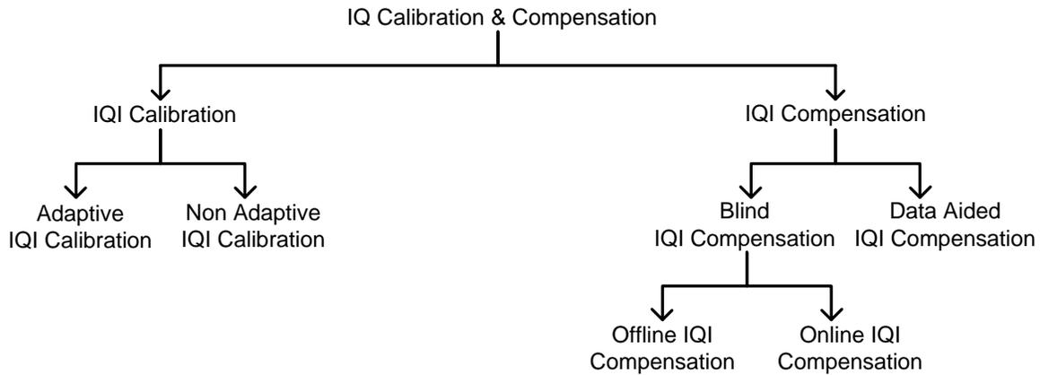
Fig. 29: IQI Calibration and Compensation Classification
