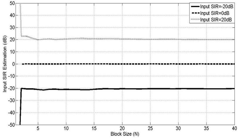
Fig. 60:  $SIR_{in}$  estimation against the block size ( $N$ ) at  $SNR=35dB$  using a single realization,  $g=1.02$  and  $\phi=2^0$
