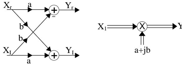
Fig. 9: Real & Complex Signal Multiplication
