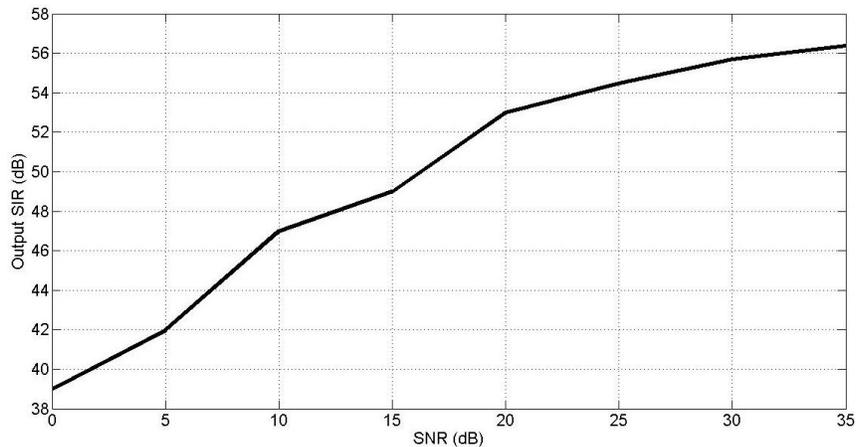
**Fig. 71: Output SIR across SNR at different values of input SIR,  $g=1.02$ ,  $\phi=2^0$**
