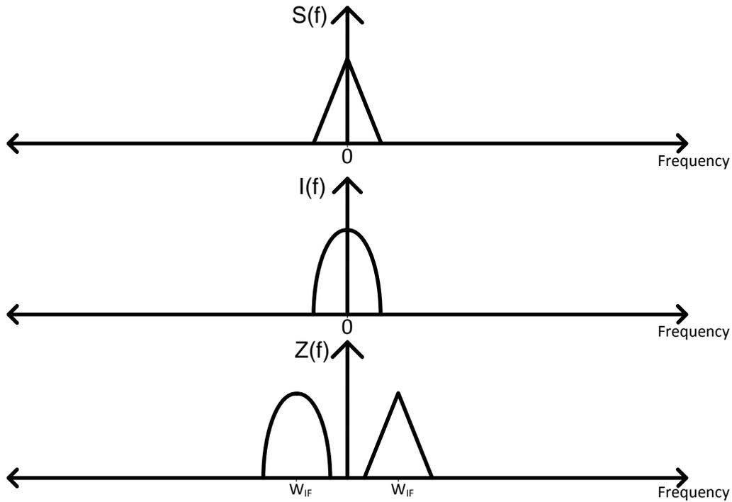
**Fig. 25: Frequency response of the base band desired Signal, base band image signal, Non Symmetric Low Pass Equivalent signal for the RF signal**
