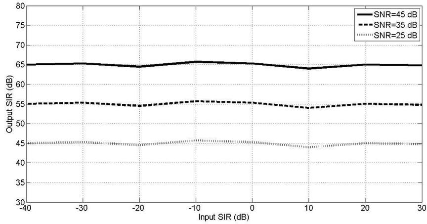
Fig. 74: Output SIR across Input SIR for different SNR values,  $g=1.02$ ,  $\phi=2$  degree's
