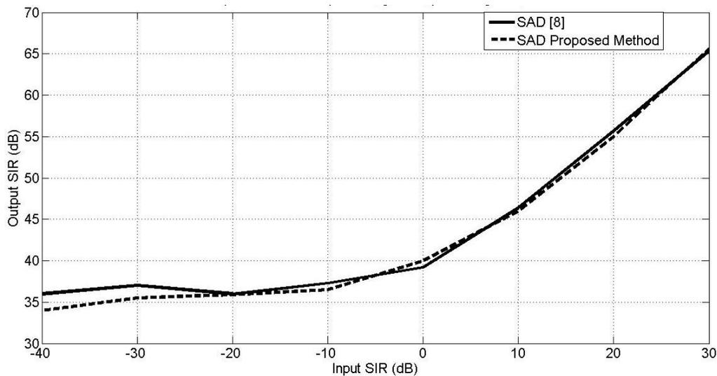
Fig. 68: Output SIR across Input SIR for the SAD in [11] and the its variant proposed in this work,  $g=1.02$ ,  $\phi=2$  degree's,  $N=1e4$
