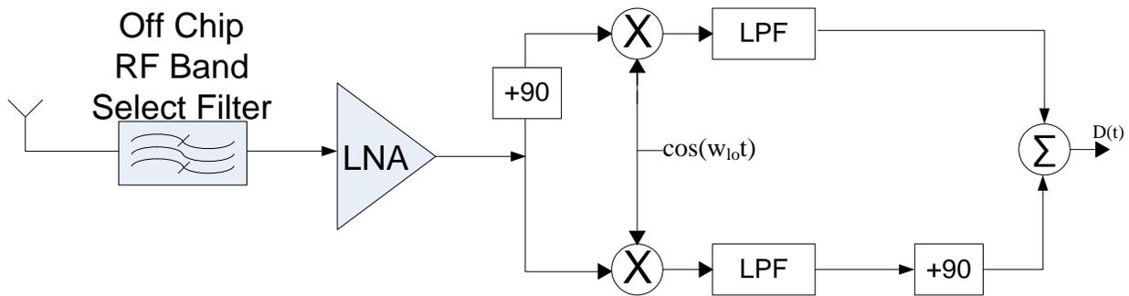
**Fig. 17: Hartley Receiver Architecture Using  $90^\circ$  Hybrid at the RF & IF Sides**
