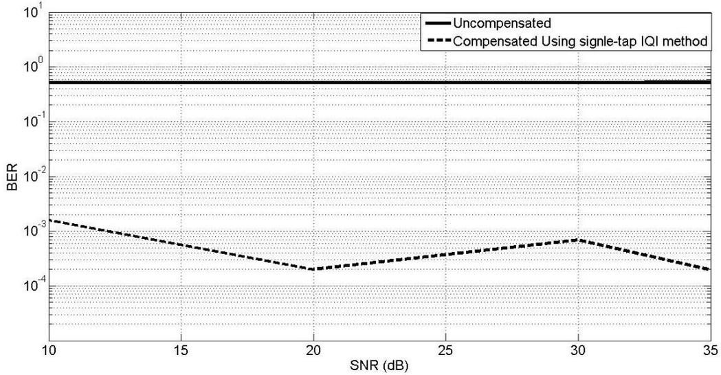
**Fig. 53: BER across SNR for the single-tap IQI compensation technique,  $g=1.02$ ,  $\phi=2$  degree's, input SIR=-40dB**
