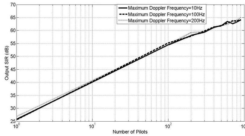
**Fig. 82: Output SIR across number of Pilots “ $N/L$ ”,  $g=1.02$ ,  $\phi=2$  degree’s, input SIR=-20dB, SNR=35dB with Rayleigh Fading,  $L=2$**
