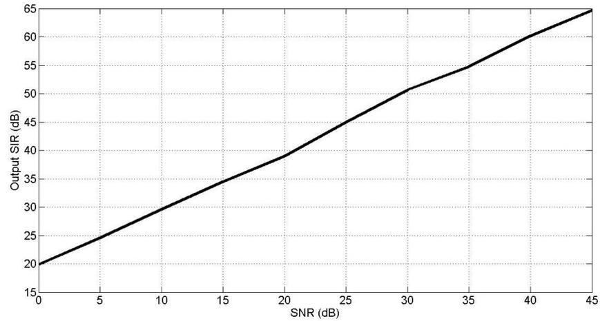
Fig. 75: Output SIR across the SNR for input SIR=-20dB,  $g=1.02$ ,  $\phi=2$  degree's
