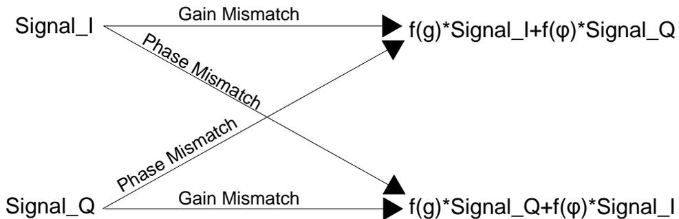
**Fig. 35: Impact of the IQ mismatch on the Relation Between the I & Q Signals**
