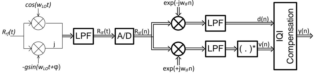
**Fig. 1: Secondary Double Quadrature Mixing Image Reject Receiver (Modified Weaver Architecture)**
