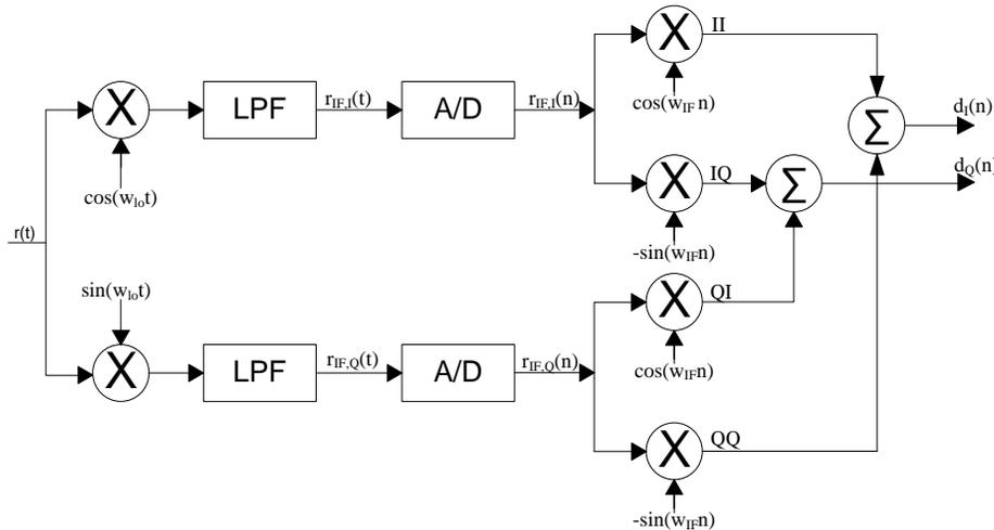
**Fig. 20: Modified Weaver Receiver Architecture (Secondary Double Quadrature Receiver)**
