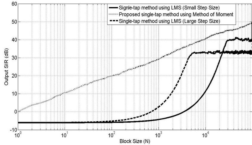
**Fig. 49:  $SIR_{out}$  across time ( $n$ ) for the single-tap method using LMS and the proposed single-tap method using Method of Moments,  $SIR_{in}=-40dB$ , SNR=35dB,  $g=1.02$  and  $\phi=2^0$**
