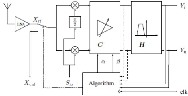
**Fig. 33: Low IF Receiver with complex filter, Adjusting IQI using Adjusting Block "C" [17]**
