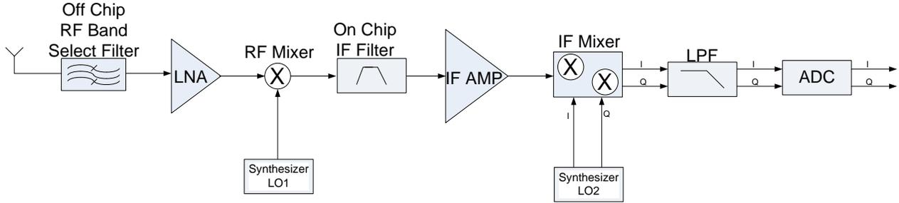
**Fig. 7: Low IF Receiver Architecture**
