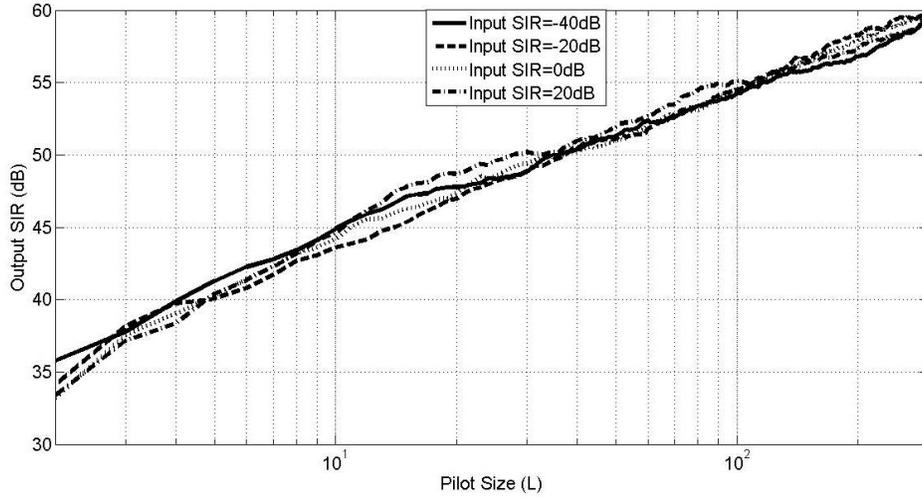
Fig. 73: Output SIR across pilot length (L), SNR=35dB,  $g=1.02$ ,  $\phi=2$  degree's
