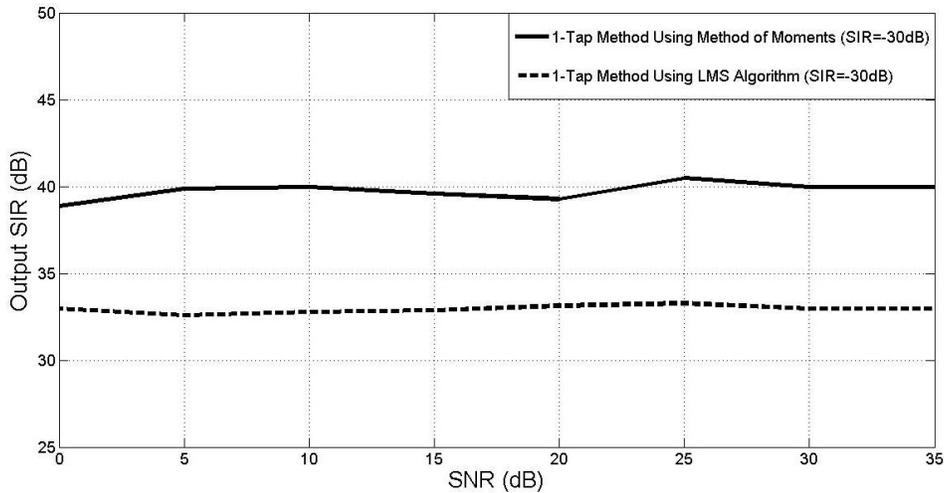
**Fig. 52: Output SIR across SNR at different values of input SIR,  $g=1.02$ ,  $\phi=2^0$**
