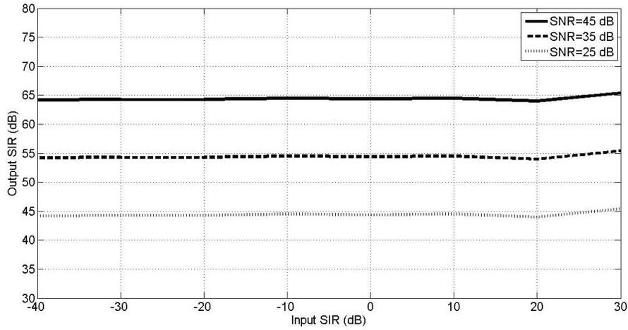
**Fig. 84: Output SIR across input SIR for different SNR values,  $g=1.02$ ,  $\phi=2$  degree’s**
