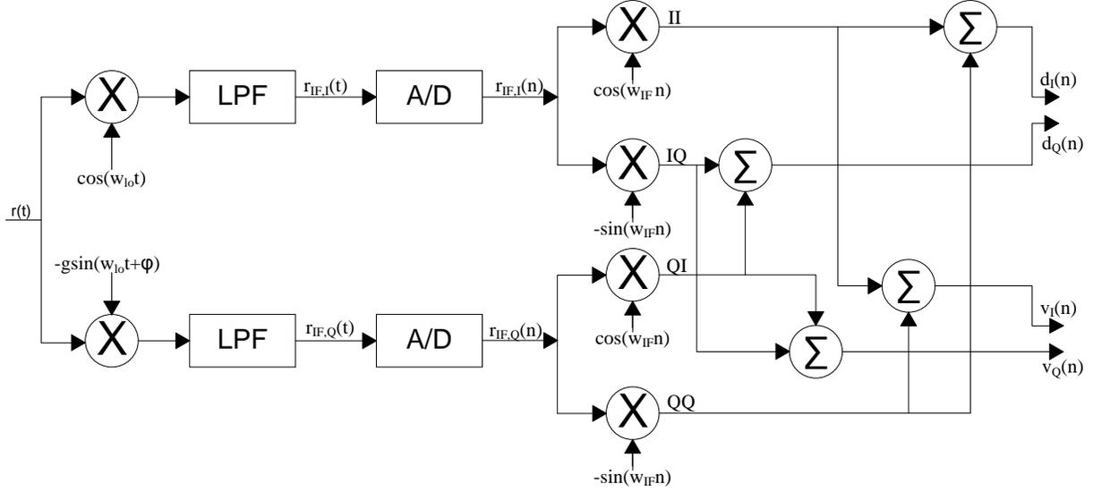
**Fig. 23: Modified Weaver Architecture Model Including IQ Mismatches**
