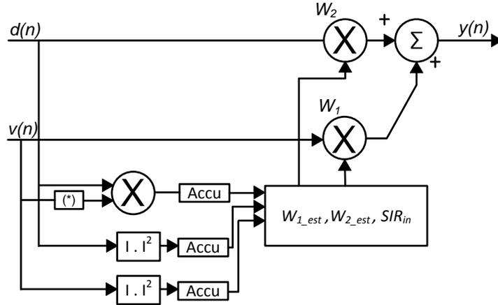
Fig. 55: Dual-Tap IQI Compensation using method of moments, first approach measuring three moments
