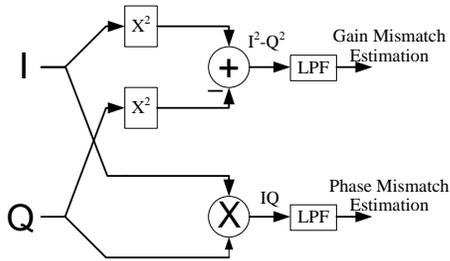
**Fig. 36: The IQ Correlation Used as indication for phase mismatch, while the difference between the variances is used as indication for the gain mismatch [22]**
