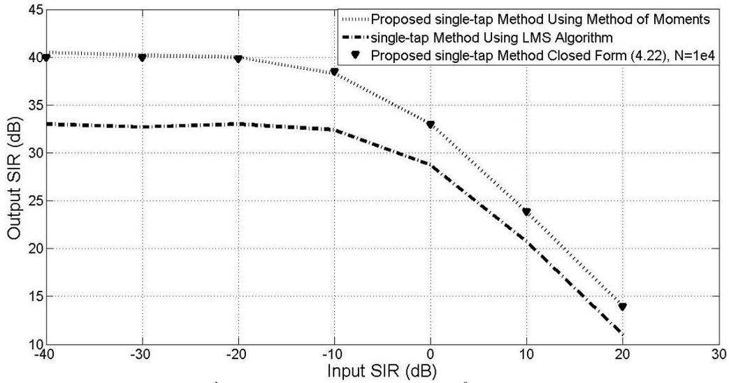
Fig. 50:  $SIR_{out}$  across  $SIR_{in}$  at  $N=10^4$ ,  $SNR=35dB$ ,  $g=1.02$  and  $\phi=2^0$ .
