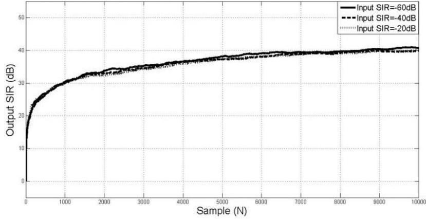
**Fig. 47: single-tap IQI compensation method using Method of Moment, Output SIR across Time,  $g=1.02$ ,  $\phi=2^0$ , SNR=35dB**
