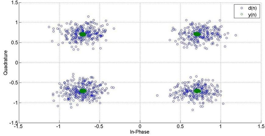
Fig. 76: Signal constellation for the compensated signal  $y(n)$  and the uncompensated signal  $d(n)$ ,  $g=1.02$ ,  $\phi=2$  degree's, input SIR=-20dB, SNR=35dB
