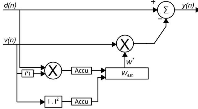
**Fig. 44: Single-tap IQI Compensation Using Method of Moments**
