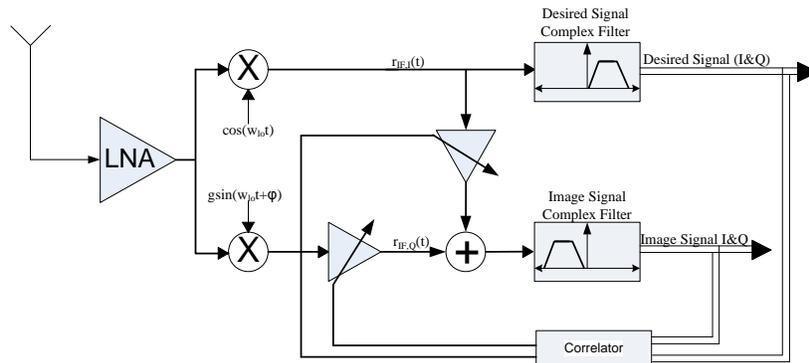
**Fig. 38: IQ compensation generating the desired and image signal using two analog complex filters [25]**
