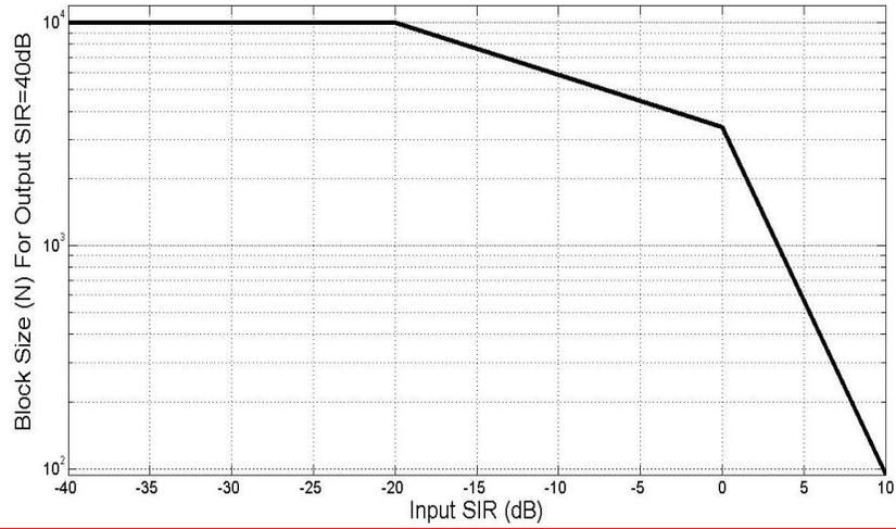
Fig. 61: The Block Size ( $N$ ) required to reach  $SIR_{out}=40dB$  across  $SIR_{in}$  for the proposed dual-tap IQI Compensation Using Method of Moments.
