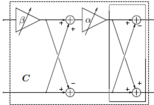
**Fig. 34: Adaptive block for IQI Compensation in signal path [17]**
