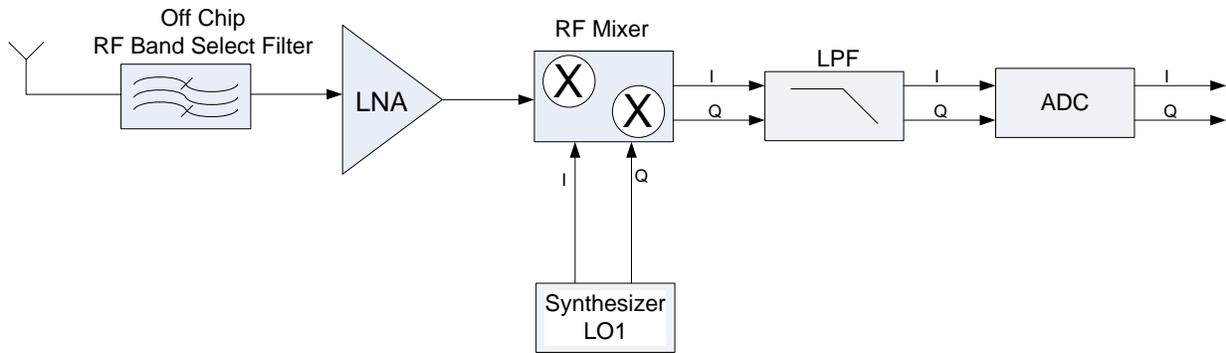
Fig. 5: Direct Conversion Receiver Architecture
