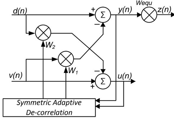
**Fig. 66: Symmetric Adaptive De-correlation With Equalizing Filter**
