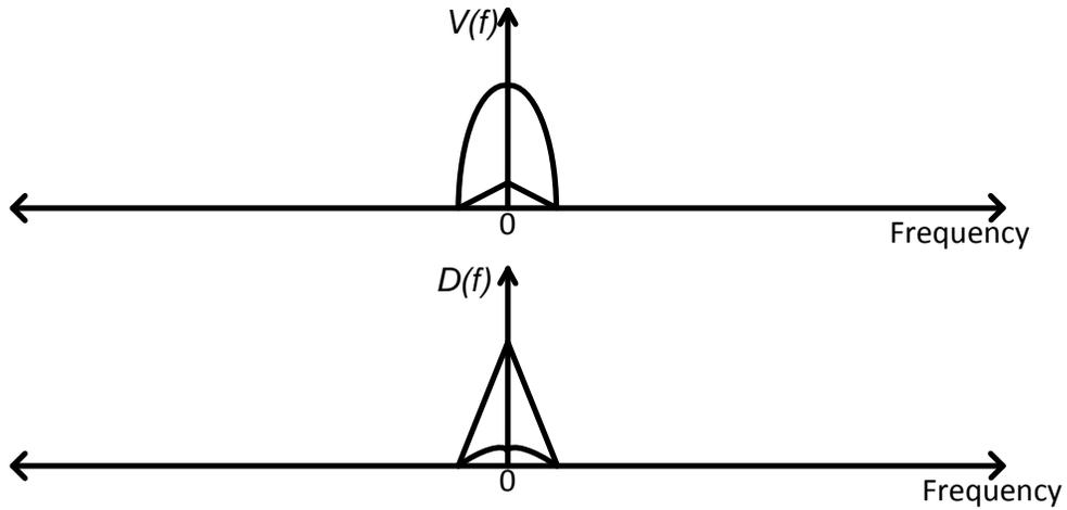
**Fig. 28: a) The Image signal corrupted by the desired signal b) The desired signal corrupted by the image signal**
