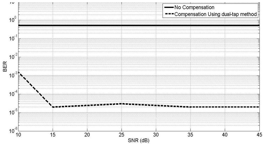
**Fig. 63: BER across SNR for the dual-tap IQI compensation technique,  $g=1.02$ ,  $\phi=2$  degree's, input SIR=-40dB**
