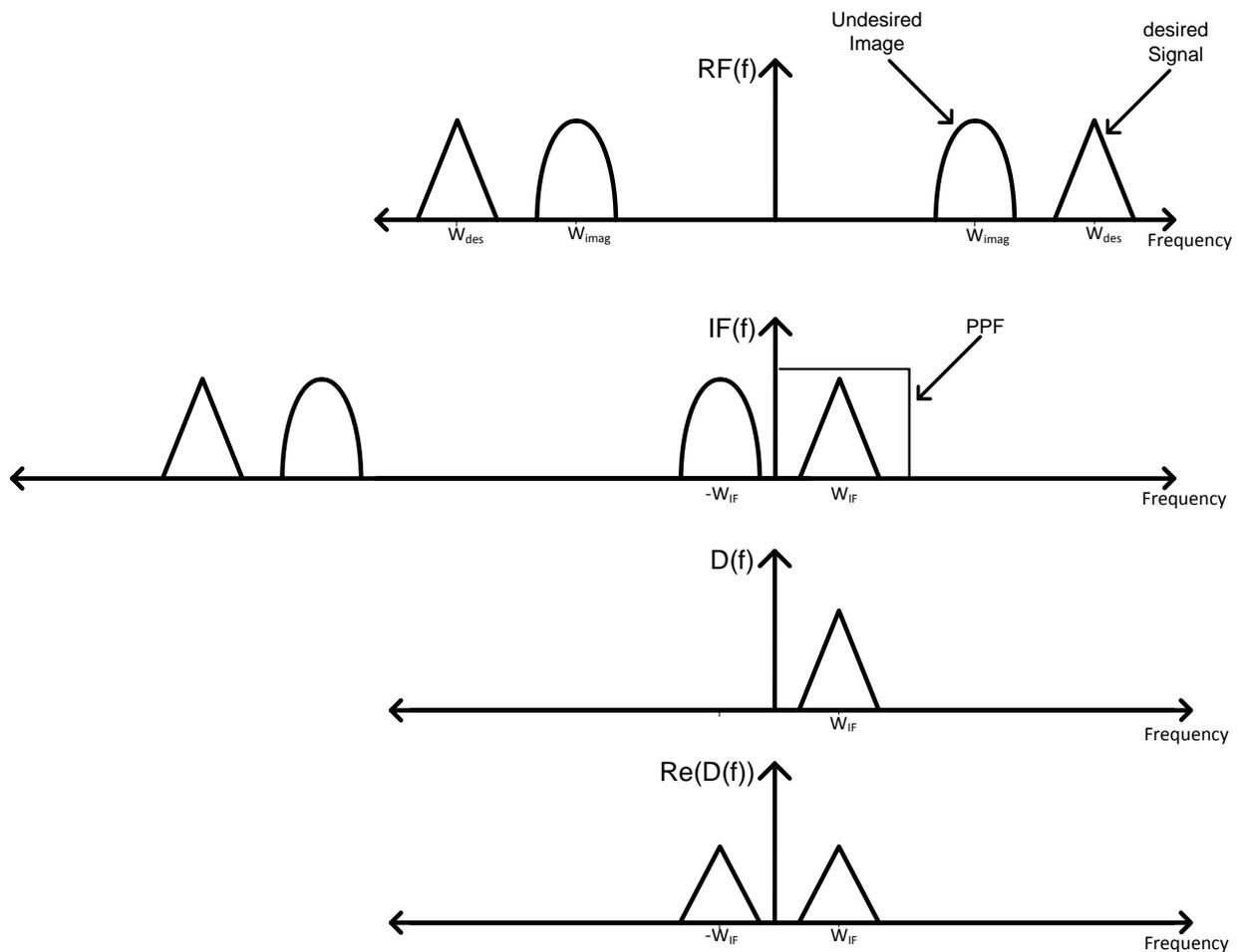
Fig. 21: Complex Frequency Spectrum For the Quadrature Mixing & Image Signal Filtration
