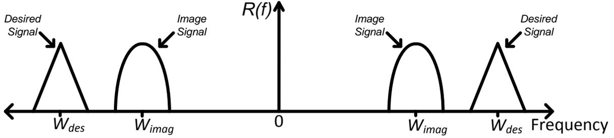
Fig. 26: Frequency Response of the RF signal  $r(t)$
