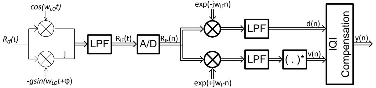
**Fig. 24: Modified Weaver Architecture in Complex Domain**
