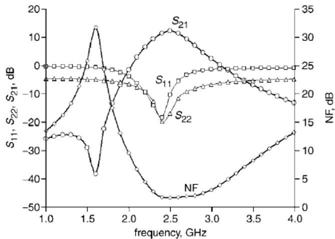
Fig. 14: Frequency Response of the image reject LNA [18]
