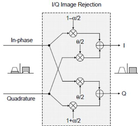
**Fig. 37: Gain & Phase Mismatch Estimates are used as inputs for a Compensating block in the signal path**
