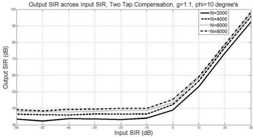
**Fig. 58: 2-Tap Method Using Method of Moment, Output SIR across input SIR,  $g=1.1$ ,  $\phi=10^\circ$ , SNR=35dB**
