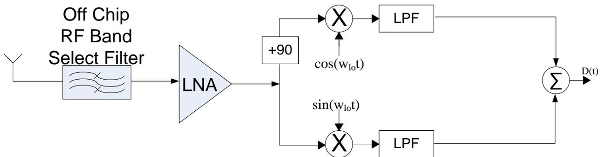
Fig. 16: Hartley Receiver Architecture Using  $90^\circ$  Hybrid at the LO & RF Sides
