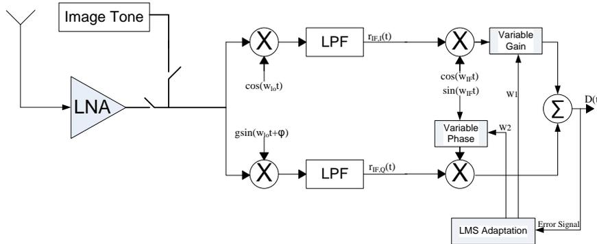
**Fig. 32: Generating the image signal on chip to allow adaptive calibration**
