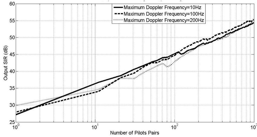
**Fig. 79: Output SIR across number of Pilots “N” ,  $g=1.02$ ,  $\phi=2$  degree’s, input SIR=-40dB, SNR=35dB with Rayleigh Fading**
