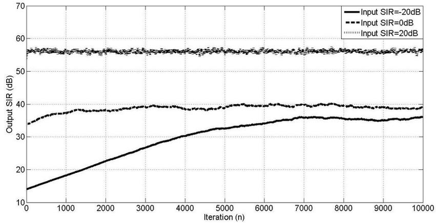
**Fig. 69: Proposed dual-tap IQI compensation Using LMS Algorithm, Output SIR across Time Iterations (n),  $g=1.02$ ,  $\phi=2^0$ , SNR=35dB**
