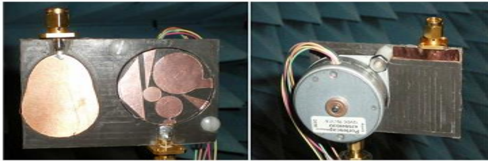
Figure 2.5: The fabricated antenna with the stepper motor mounted on the back of the substrate.
