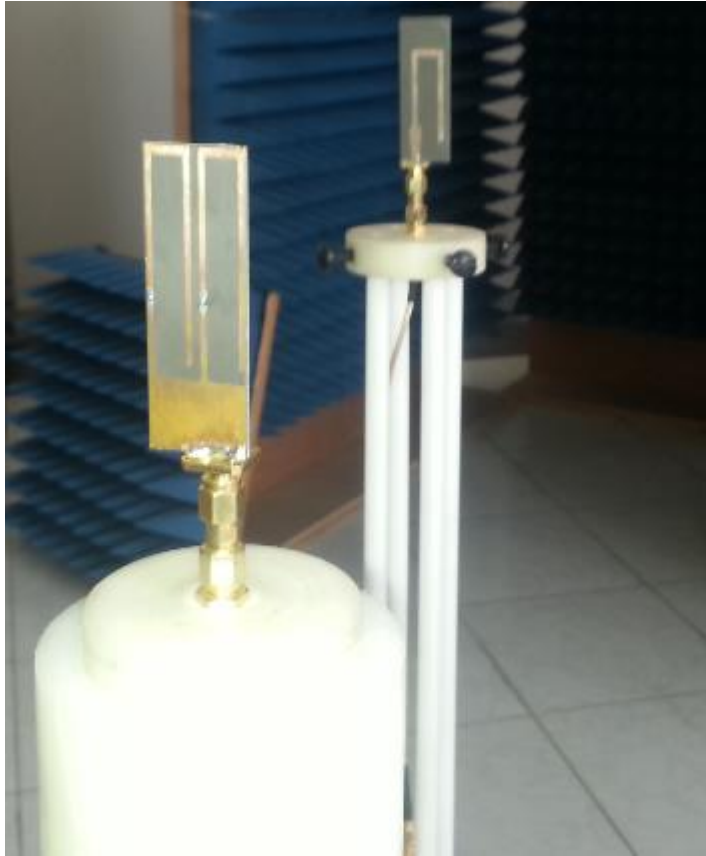
Figure 5.12: Two identical antennas were used in free space to measure the radiation pattern.
