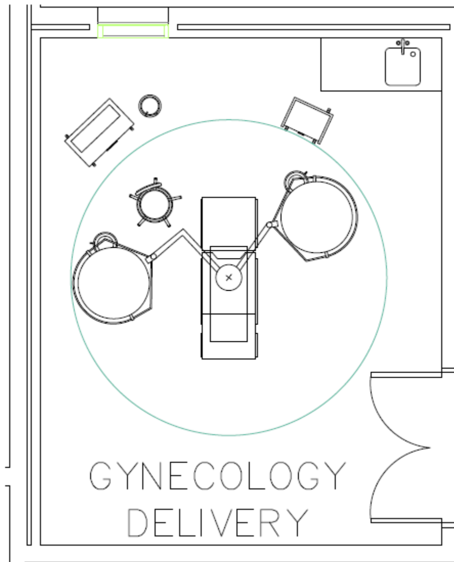
Figure 62: Gynecology plan in an ED Scale 1:50
