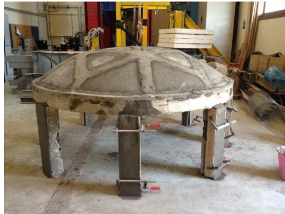
Fig. 103: Plastering of all model columns
