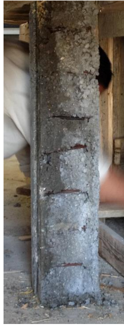
Fig. 102: Honeycombing found in two of the model columns
