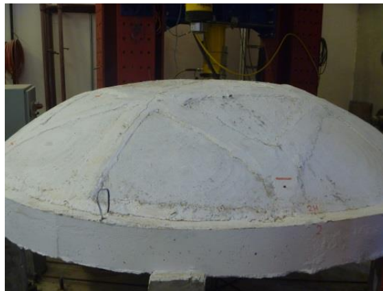
Fig. 178: Flattening of the central region of the experimental model
