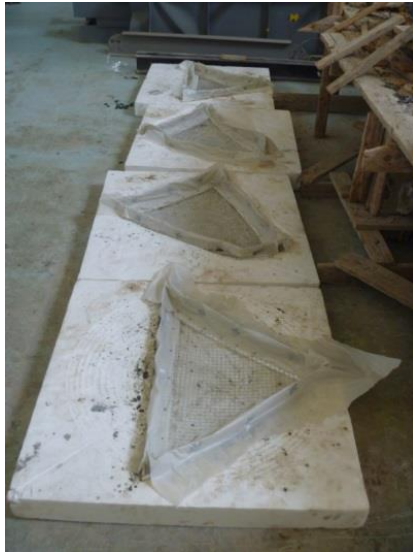
Fig. 86: Panels cast with reinforcement insulation
