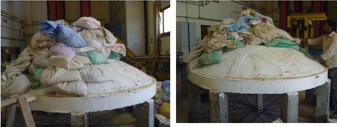
Fig. 113: Unsymmetrical loading of test 2
