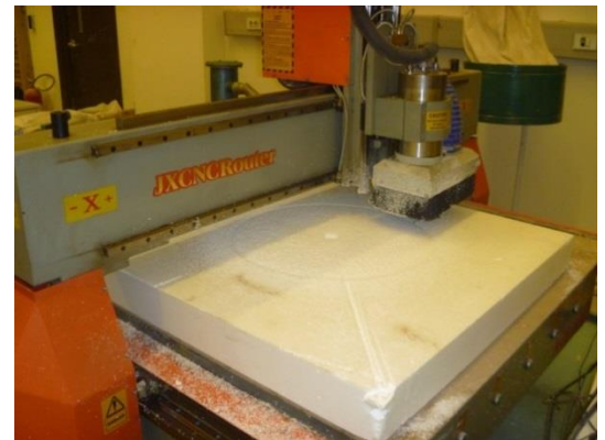
Fig. 72: Mold fabrication using CNC router machine
