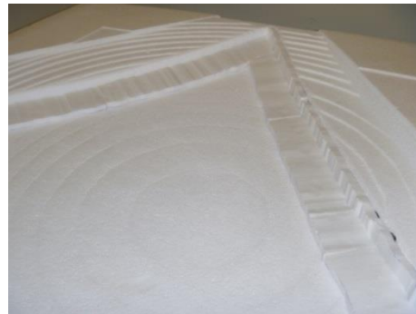
Fig. 74: Lining of the molds to create panel joints
