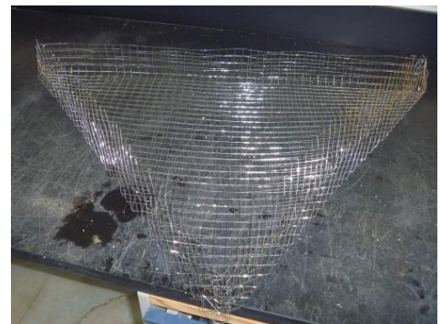
Fig. 83: Wire mesh used to reinforce shell panels
