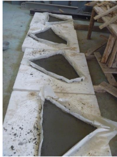
Fig. 86: Panels cast with reinforcement insulation
