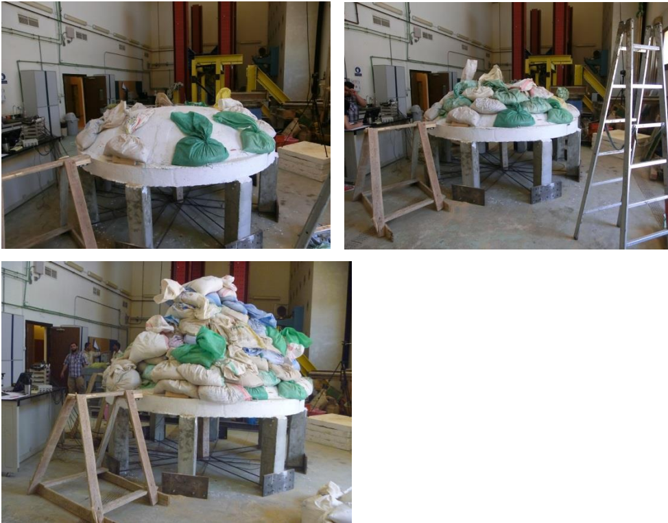
Fig. 112: Axisymmetric loading of test 1
