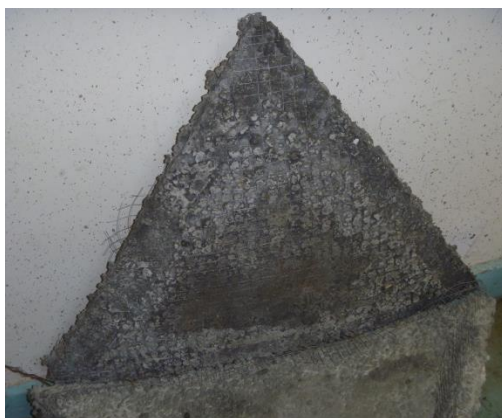
Fig. 66: Panel cast using initial concrete mix
