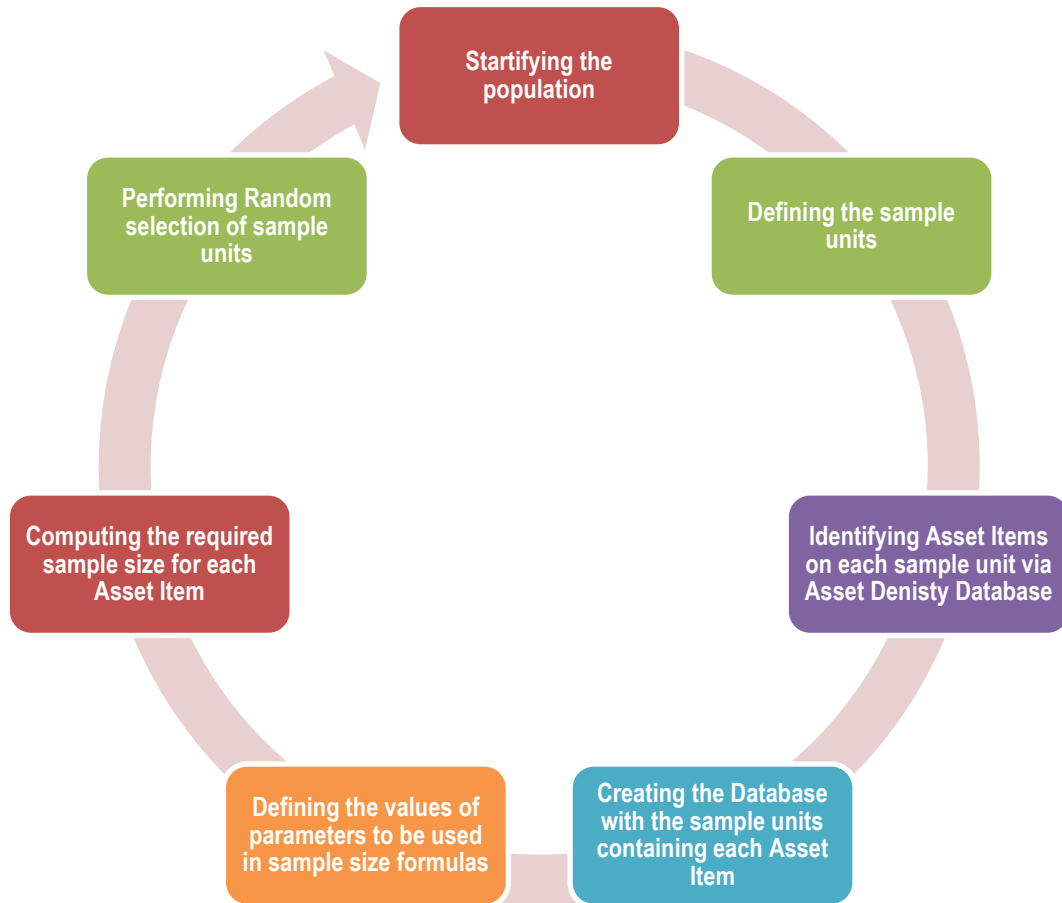
Figure 2-11: Seven steps for pavement sampling procedures for PBRMC (De la Garza et al., 2008)
