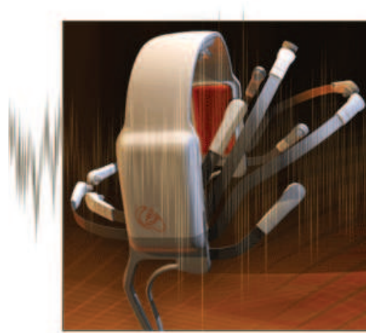
Figure 3.6: Emotiv headset with 16 electrodes to cover the different parts of the brain.
