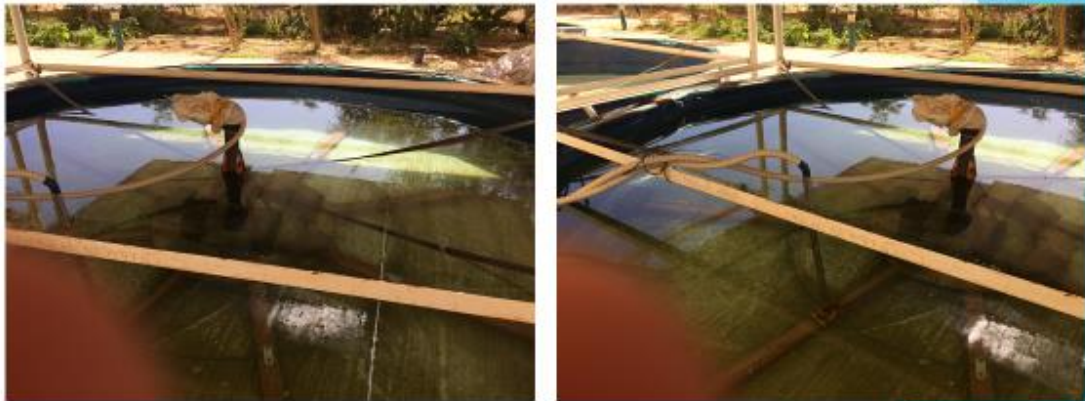
Image from east side starting to disappear as sun moves more to the south (towards zero azimuth) , sun image reducing further to around 13%
