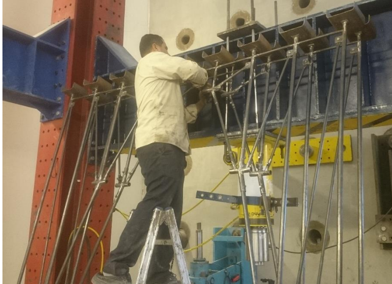
Figure 40: Assembling the trusses
