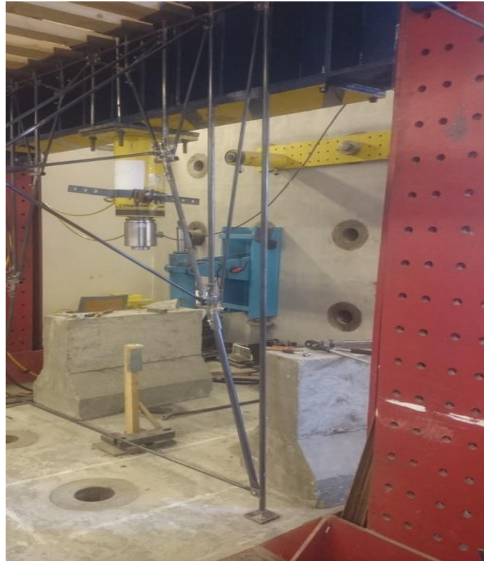
Figure 48: the Truss members did not have any Plastic Deformation
