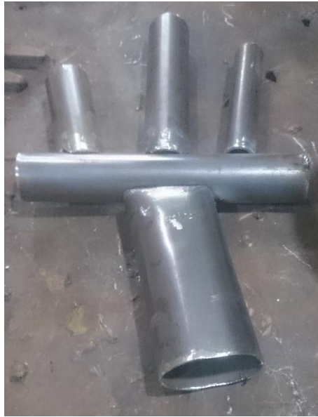
Figure 17: Connection at point 2 in the truss
