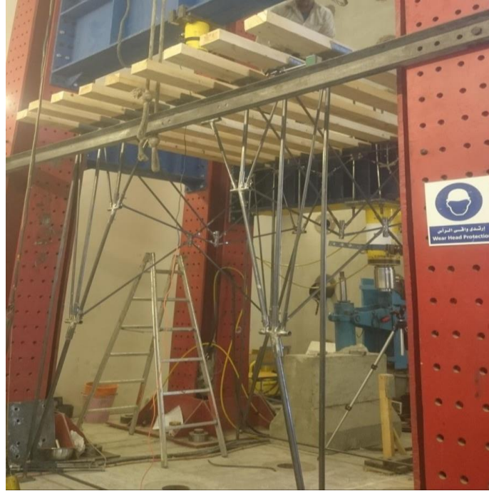
Figure 43: The installation of the joists
