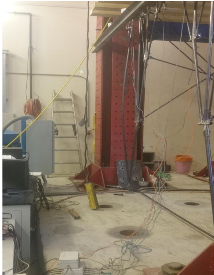
Figure 54: the Left Exterior Vertical experiences out of Plane Buckling
