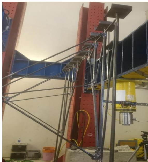
Figure 41: Connecting the Bracing System
