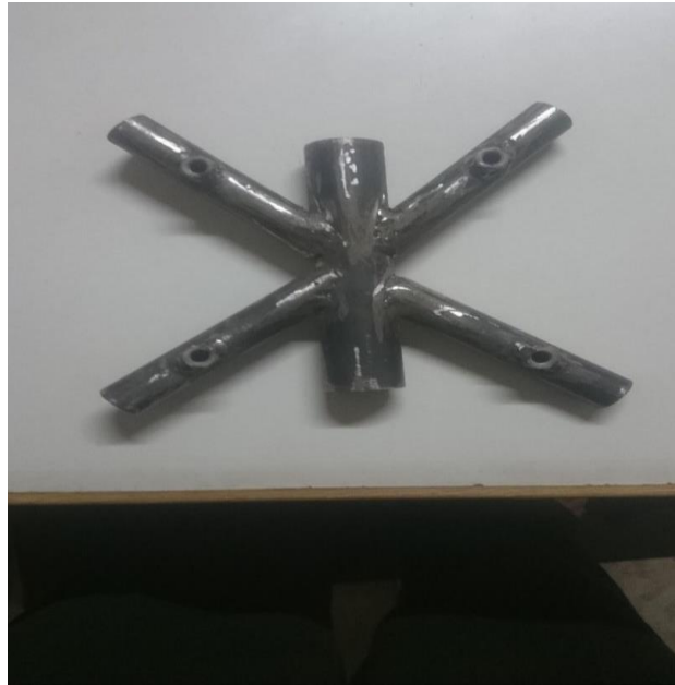
Figure 18: Connection at Bracing members
