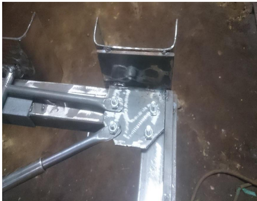
Figure 19 : Intermediate Hinge Connection
