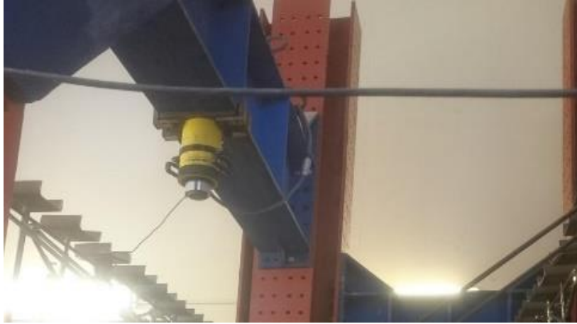
Figure 37: The Load Cell
