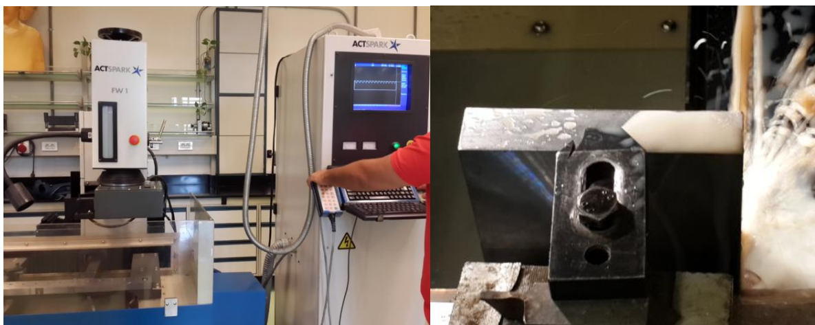
FIGURE 50 WIRE CUT MACHINE USED TO SHAPE THE DIE
