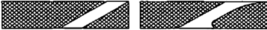
Figure 2.11: Straight and shaped (inlet and exit) non-tangential slots' configurations studied by Farmer et al. [42]
