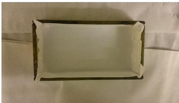
Figure 4.2: Membrane in a glass mold for IP reaction
