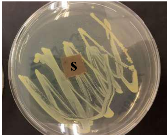
Figure 25: Testing of thermoformed LDPE sheet containing 10% w/w of GSE against Staph. aureus . There is no inhibition zone for Staph. aureus around the sheet(S).
