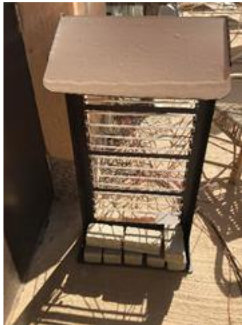
Figure 3-6 Rack and housing of coil heater loads, each load connected to its terminal in the logger and to a PV
