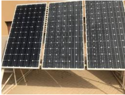
Figure 3-7 Angle 60 PVs with the left PV cleaned every day
