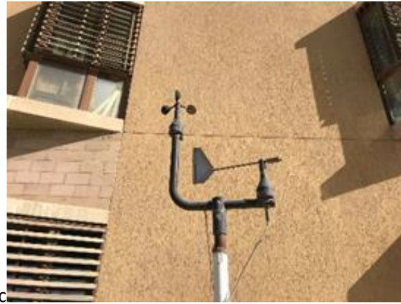
Figure 3-3 Wind speed sensor, wind direction sensor
