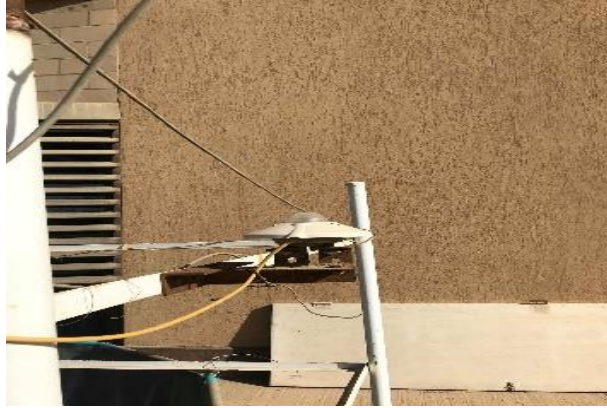
Figure 3-1 Pyranometer for measuring solar radiation
