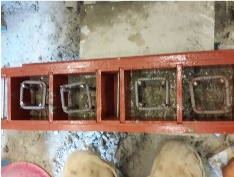
Figure 3.7: The steps of pouring reinforced concrete samples
