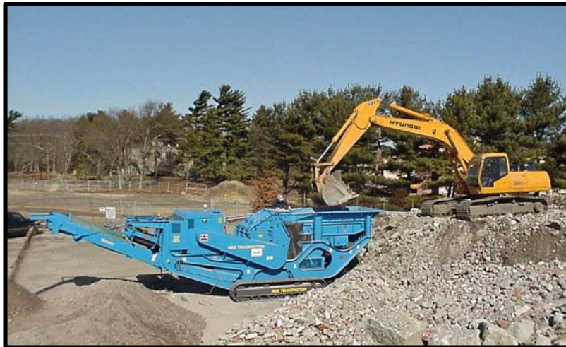
Figure 5-1: Simple recycled concrete aggregate crusher (Eagle Crushers, 2016)
