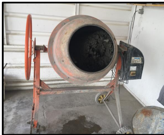
Figure 3-6: Mixing of concrete constituents using 0.06 \text{ m}^3 mixer
