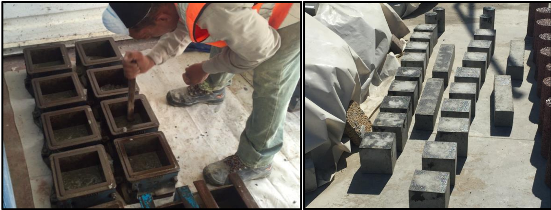
Figure 3-7: Placing and finishing of concrete specimens
