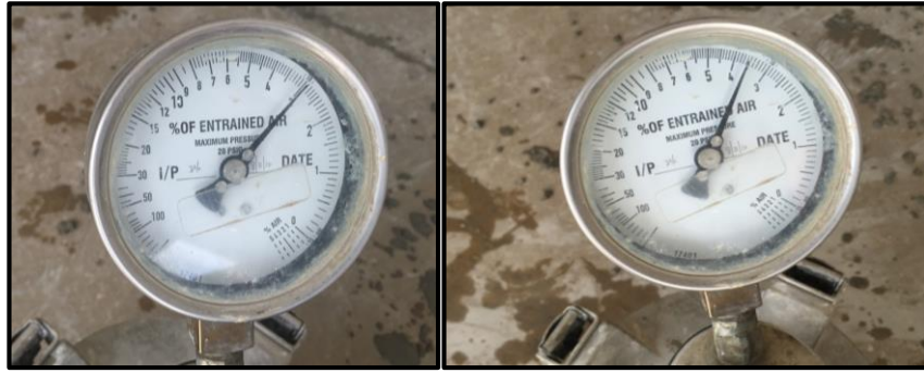
Figure 4-3: Air Content test readings for 2 different mixtures
