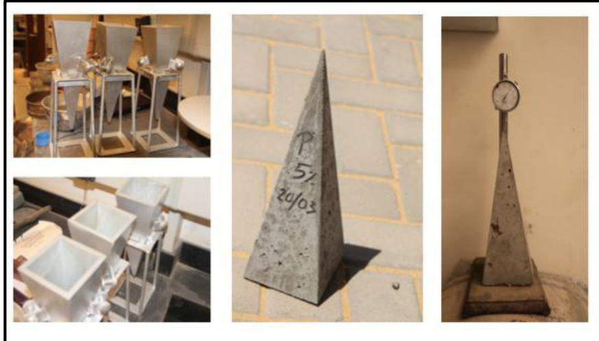
Figure 3-8: Prisms and apparatus used to perform shrinkage assessment test (Abou-Zeid, et al. 2015)
