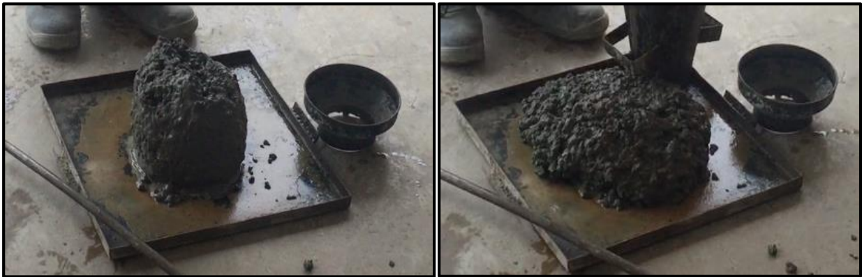
Figure 4-2: Picture showing difference in slump between Conventional mixture (left) and Perlite mixture (right)
