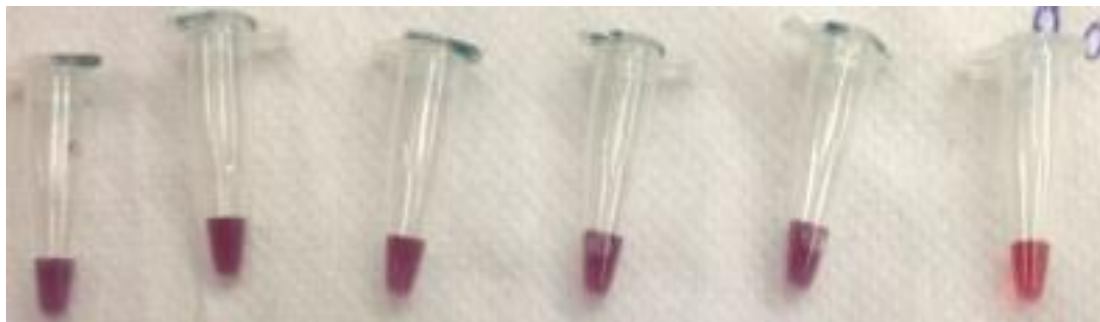
Figure 26. Cationic AuNPs assay of rpoB amplicons of MTB DNA samples. 335, 358, 331, 100 and 98. S: M. smegmatis sample. The MTB samples were amplified by the rpoB primers then cationic AuNPs were added to the amplicons. The attraction between the negatively charged amplicons and the positively charged AuNPs induced the color from red to violet due to the AuNPs aggregation. The M. smegmatis was not amplified because it lacks the complementary sequences for the primers hybridization so the AuNPs remained dispersed.
